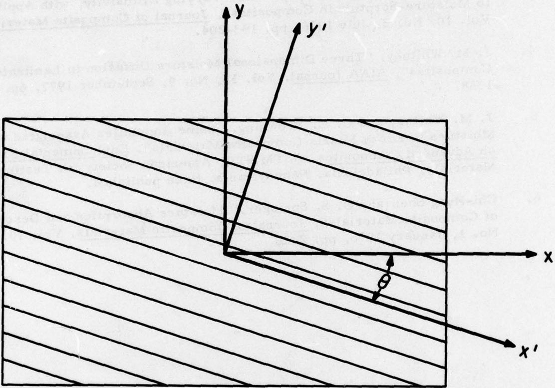
Figure 1. Off-Axis Unidirectional Lamina
