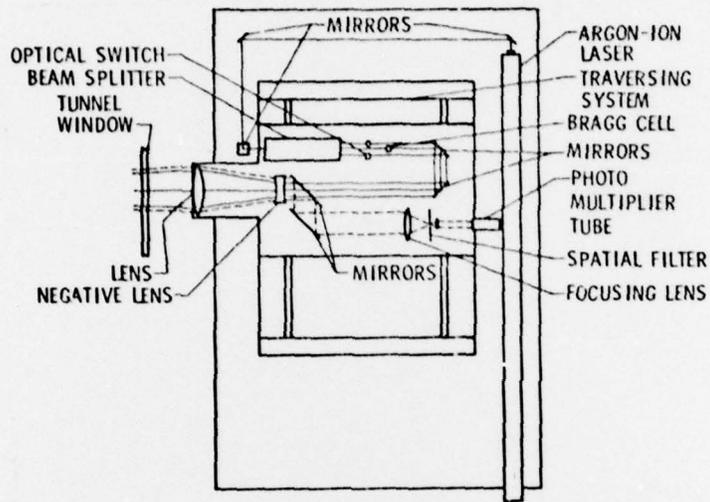
Figure 2. - Schematic of the LV optics.
