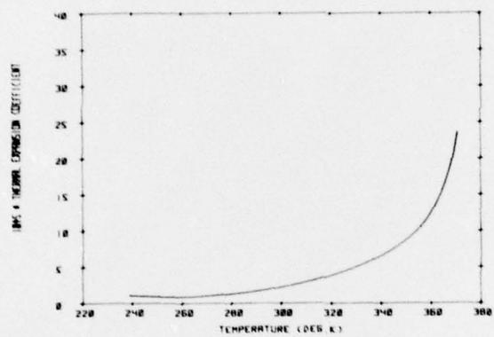
Figure 4. Linear Expansion Coefficient for ANTLAR POLA 4077 (Gardex)
