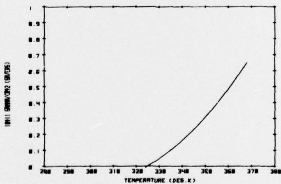
Figure 8. Gruneisen parameter for cross-ph. S Glass epoxy.
