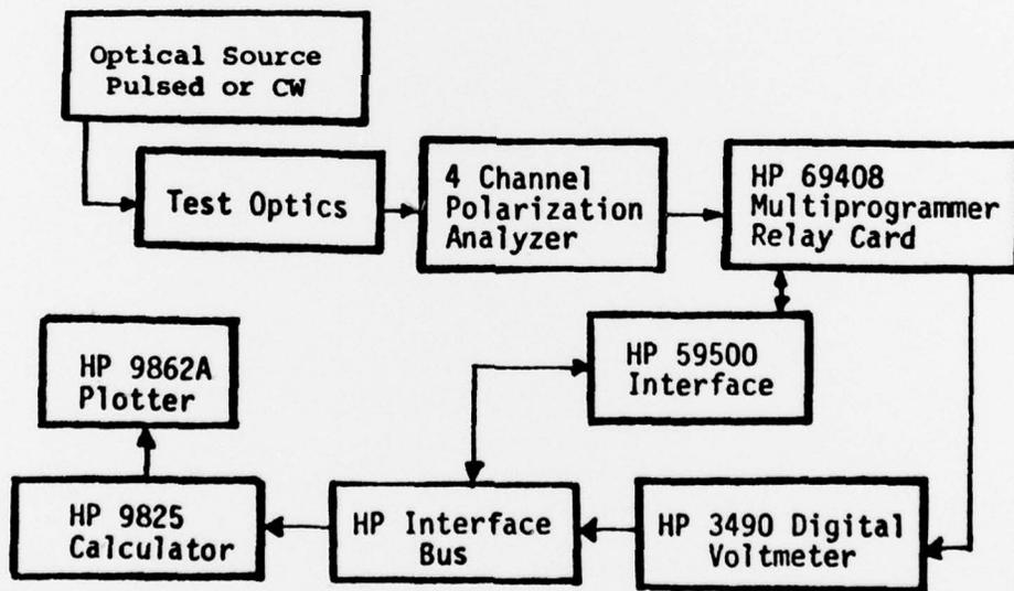
Figure 5. Block diagram of the computer-controlled polarimeter.
