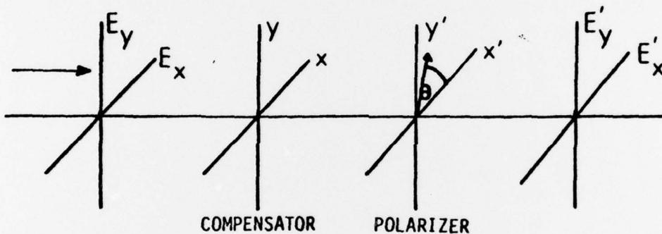
Figure 1. Measurement of the Stokes polarization parameters.
