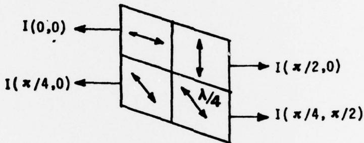
Figure 3. Parallel measurement of the Stokes polarization parameters.
