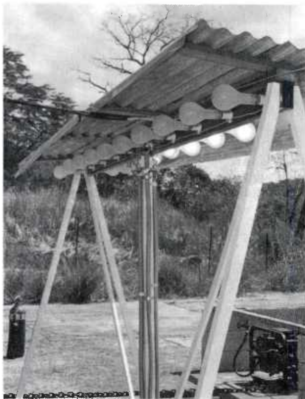
Figure 2. Load Bank System for Power Dissipation
