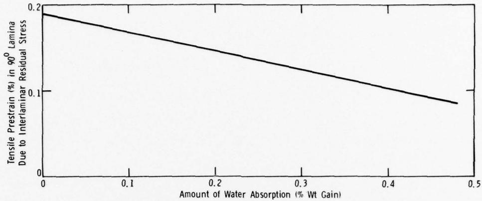
Figure 10. Effect of water absorption on the calculated tensile prestrain in the 90° lamina of a 90/0/90° laminate.
