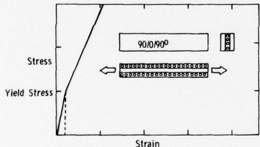
Schematic diagram of tensile stress-strain curves of a  $90/0/90^\circ$  laminate
