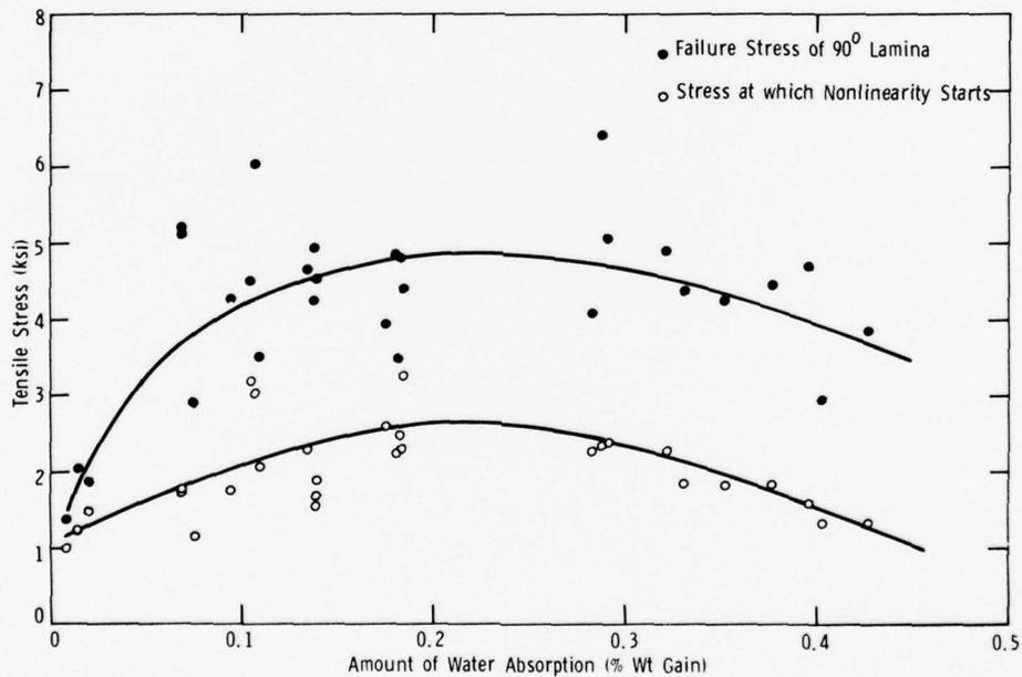
Figure 11. Effect of water absorption on the failure stress of a 90° lamina without the restraint of a 0° lamina.
