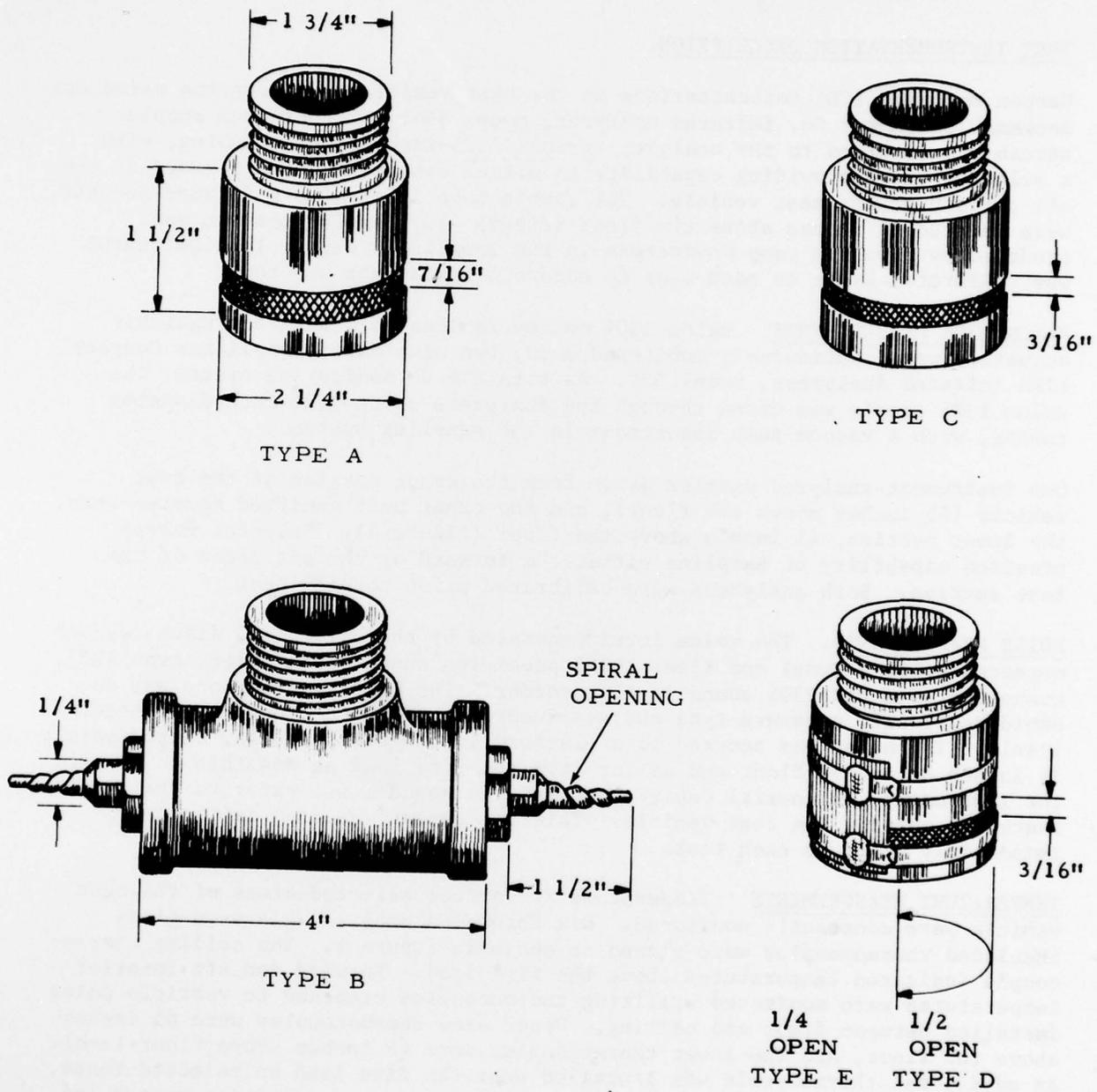
FIGURE 3. DISCHARGE NOZZLE CONFIGURATIONS
