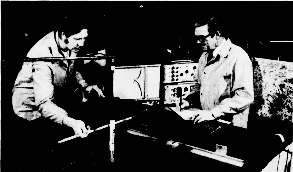
Figure 3. Typical electrolyte tank used in mapping cathodic protection electric fields.
