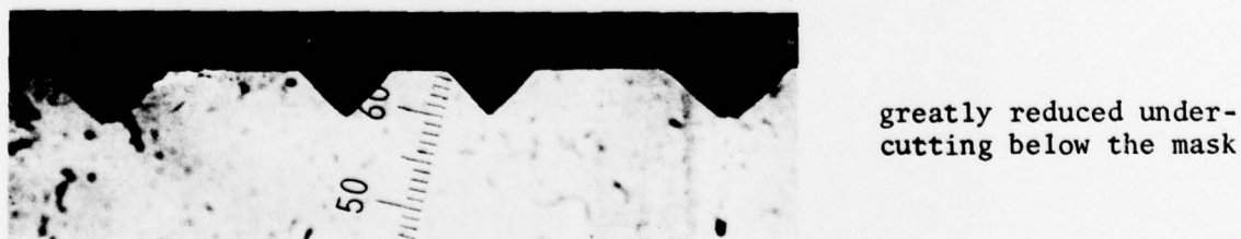
(a) mask pattern aligned parallel to to (110) reference edge
