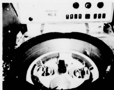
Figure 21. The red blood cell-glycerol mixture in the primary plastic collection bag is placed in an RC-3 refrigerated centrifuge, and centrifuged at 3000 rpm ( 2,350 \times g ) for seven minutes.
