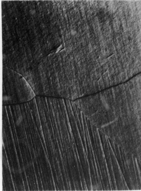
Figure 6. Etching anisotropy in \text{CaF}_2 .
