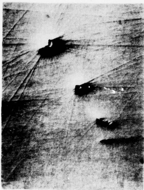
Figure 1. Craters in polishing \text{CaF}_2 caused by grinding.
