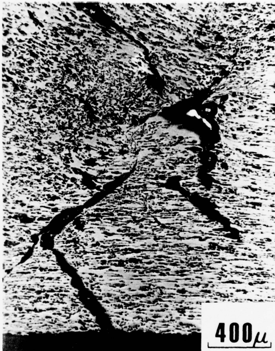
Figure 17. Longitudinal section of billet No. 8 after a total reduction of 95%.
