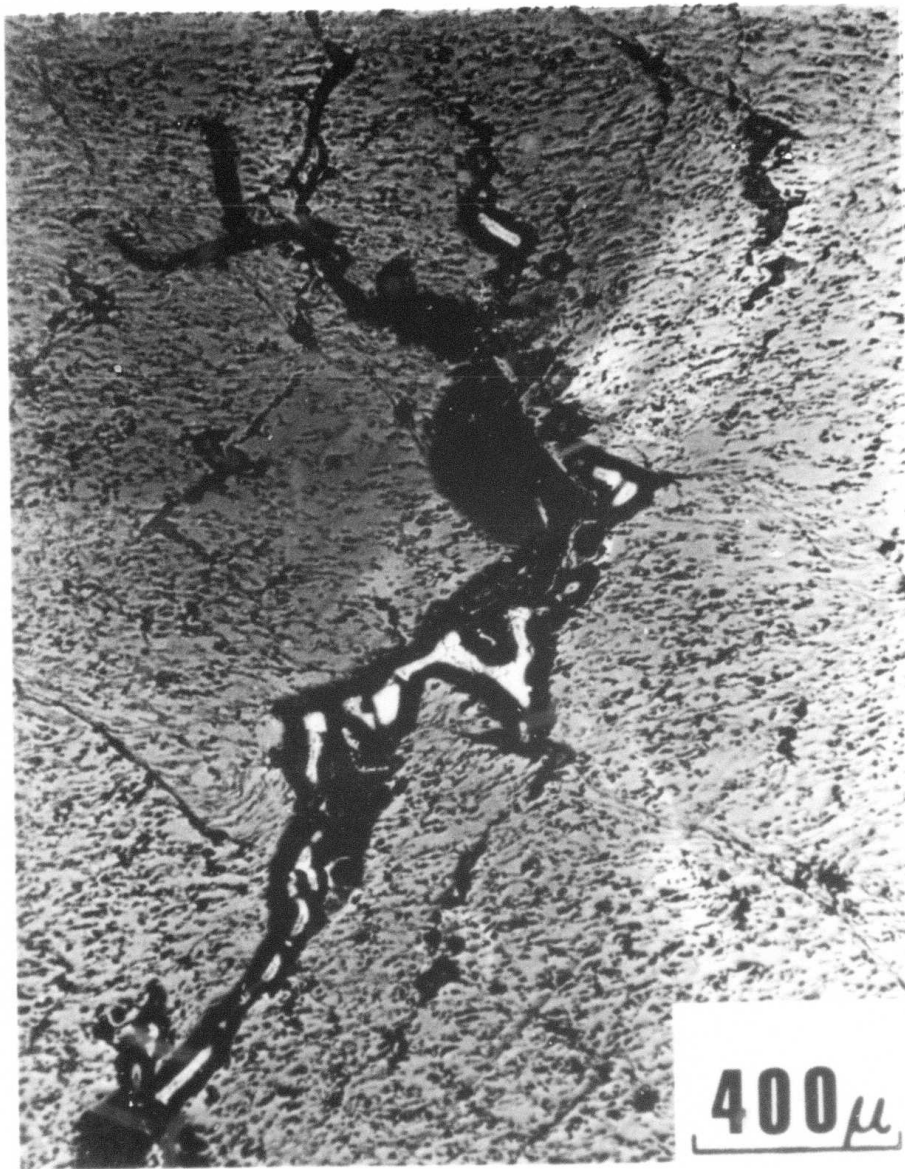
Figure 18. Longitudinal section of billet No. 7 after a total reduction of 95%.
