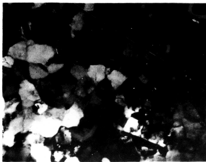
Figure 24. Electron micrograph of hydrostatically extruded Al-0.5% Fe wire. Solution treated and quenched before extrusion.
