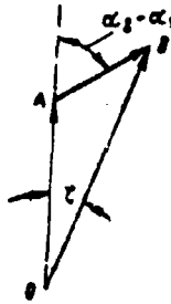
Fig. 5.8. Vector diagram of emf under the effect of the field of reradiation.
