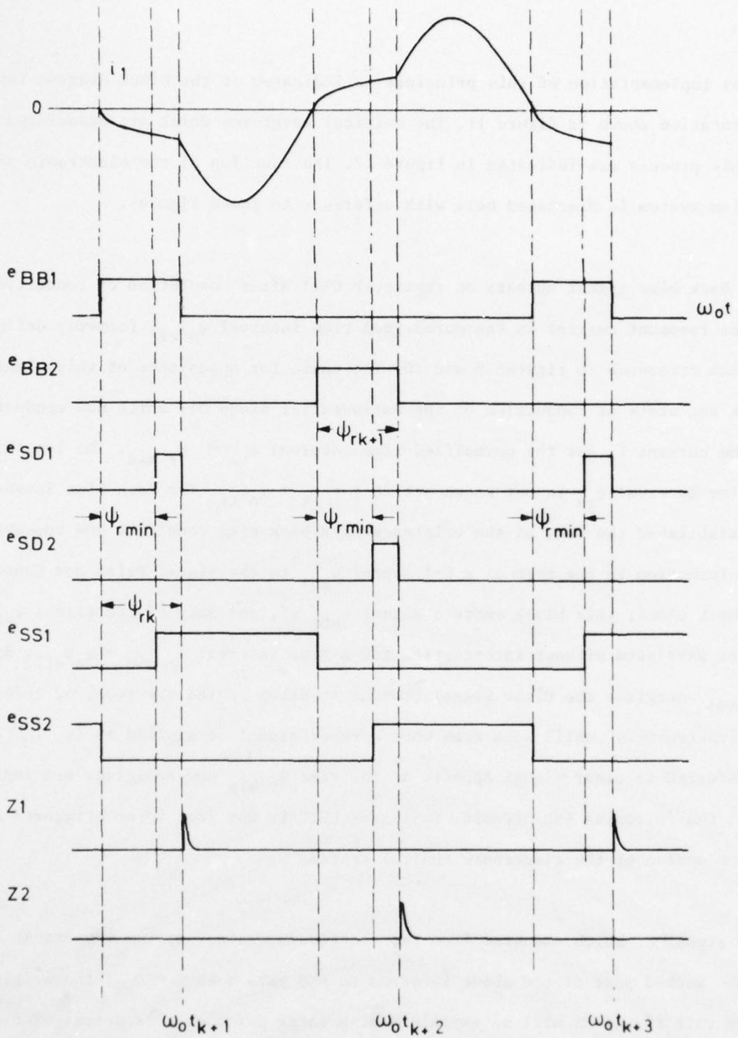
Figure 12. Critical signal waveforms of power control system.
