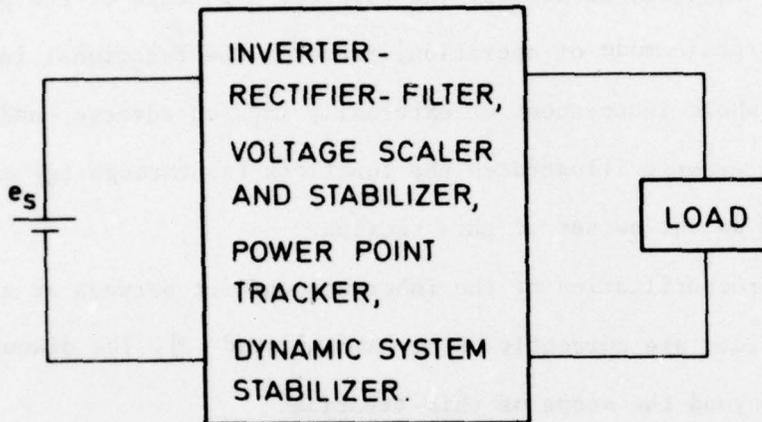
Figure 4. DC converter system in block diagram form.
