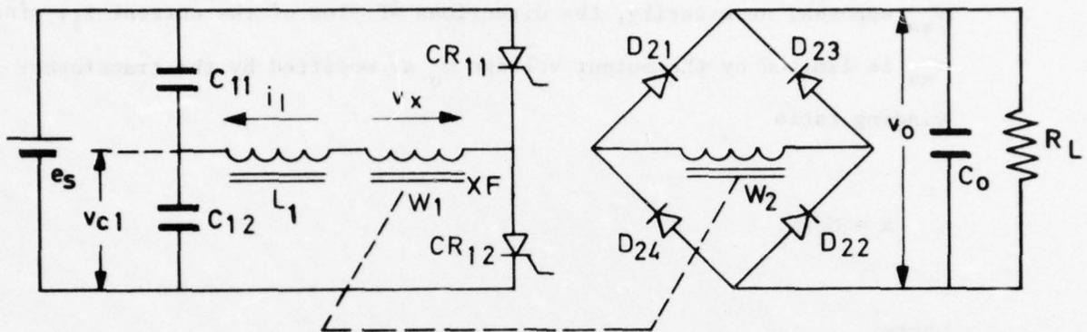
Figure 8. Simplified schematic of a dc converter which employs a series resonant circuit.
