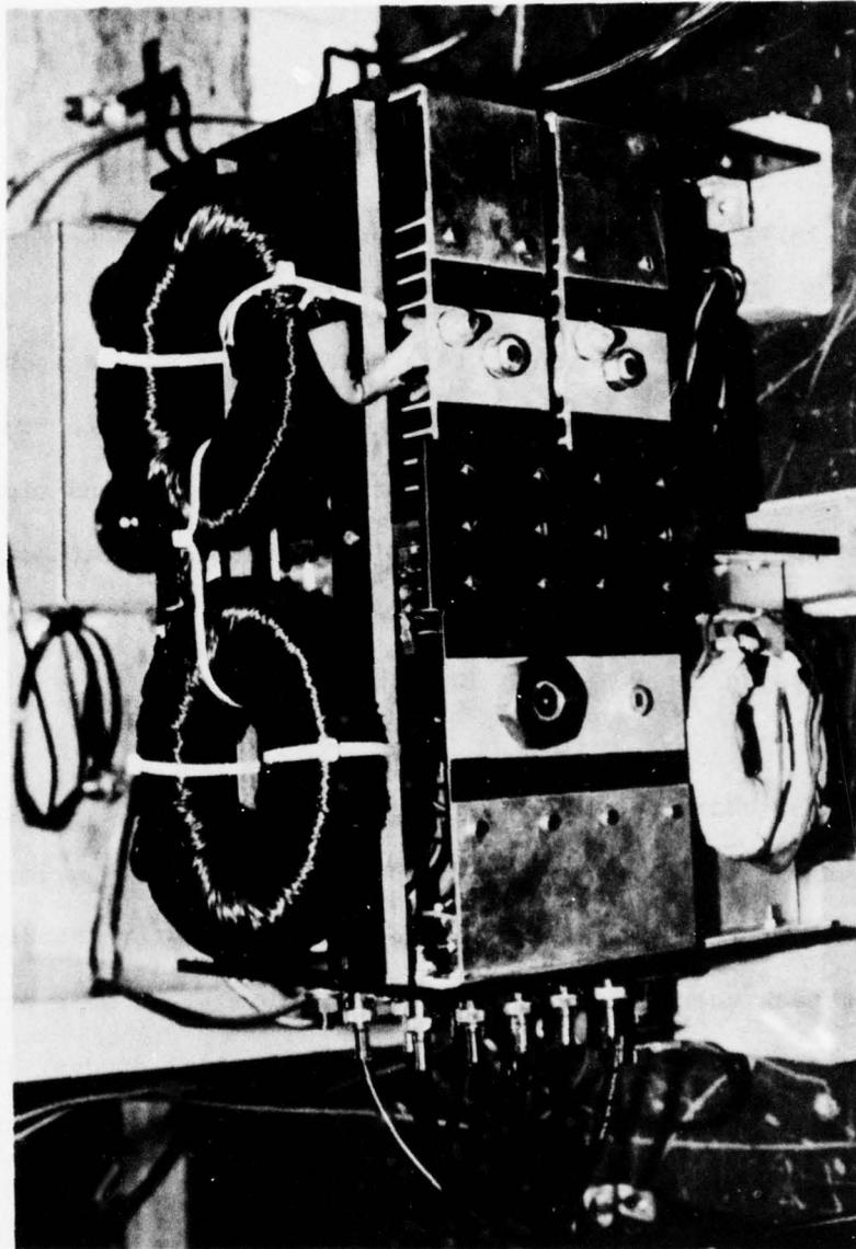
Figure 13. The power system of the light weight 10 kW converter
