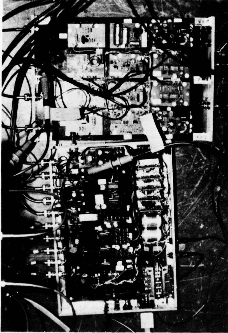
Figure 14. The control electronics of the 10 kW converter.
