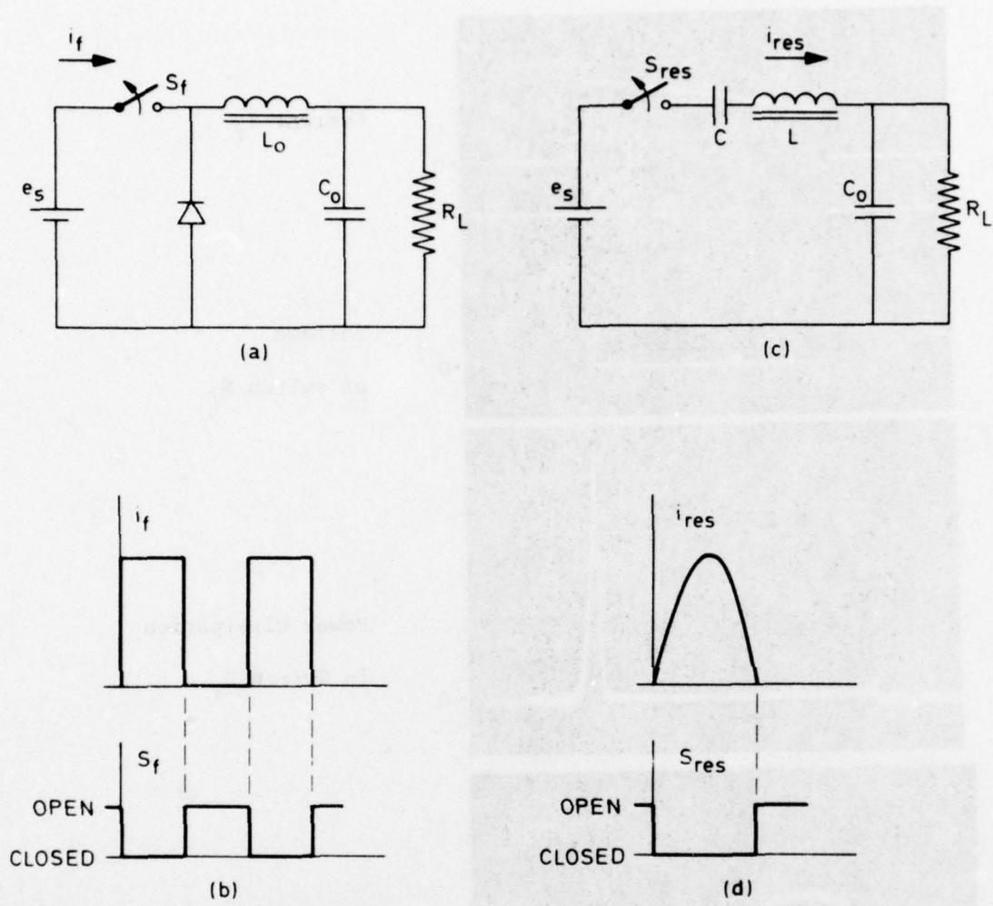
Figure 6. Power electronic switching circuits which incorporate intended and parasitic inductive elements in series with the switching elements for (a) forced interruption of the switched current, (b) the thereto pertaining current form  $i_s$  in the switch  $S_f$  and (c) switching at the instant of natural termination of the switch current  $i_{res}$  in a resonant circuit, (d) the thereto pertaining current form  $i_{res}$  in the switch  $S_{res}$ .
