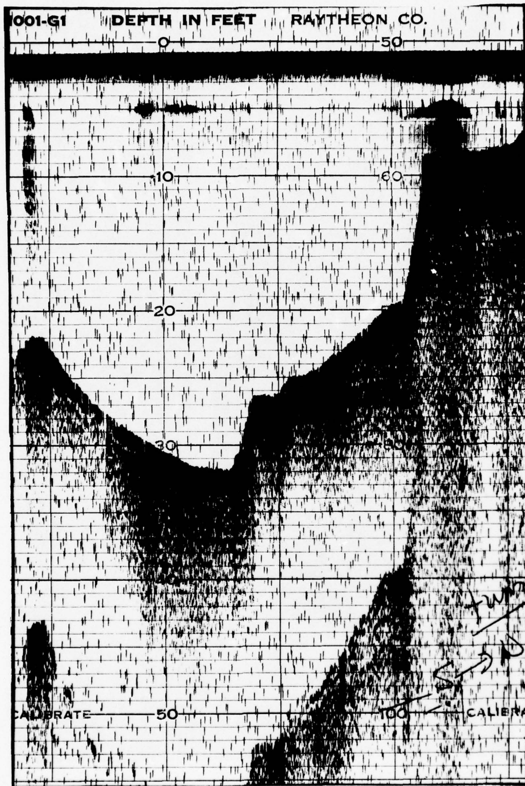
Figure 33. Sub-bottom profile across Wachapreague Inlet throat, Range 22 from north to south (north on left).
