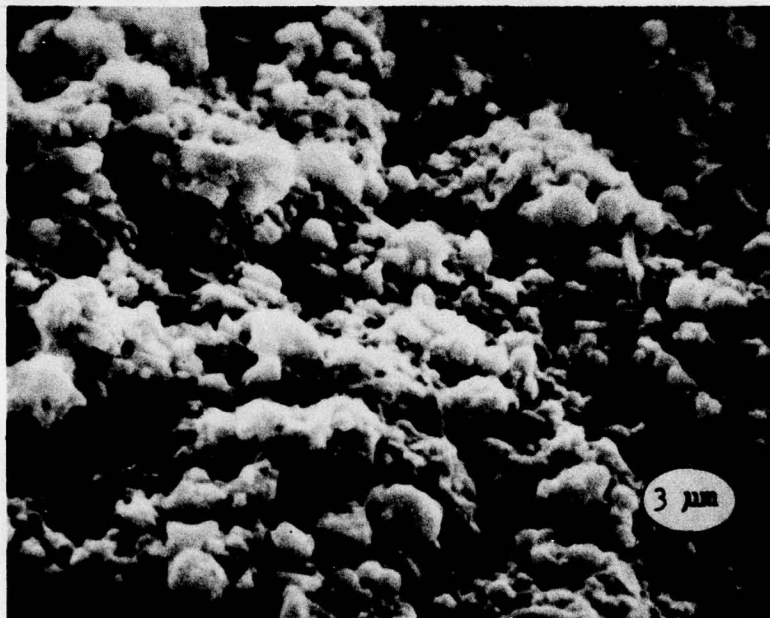
Fig. 1. Scanning electron micrograph of submicron grain size powder.
