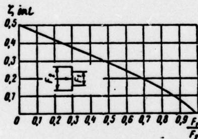
Fig. 3. The local resistance coefficient for a flow which is constricted when entering the diffuser from a rectangular chamber or from that of a different shape (other than conical).
