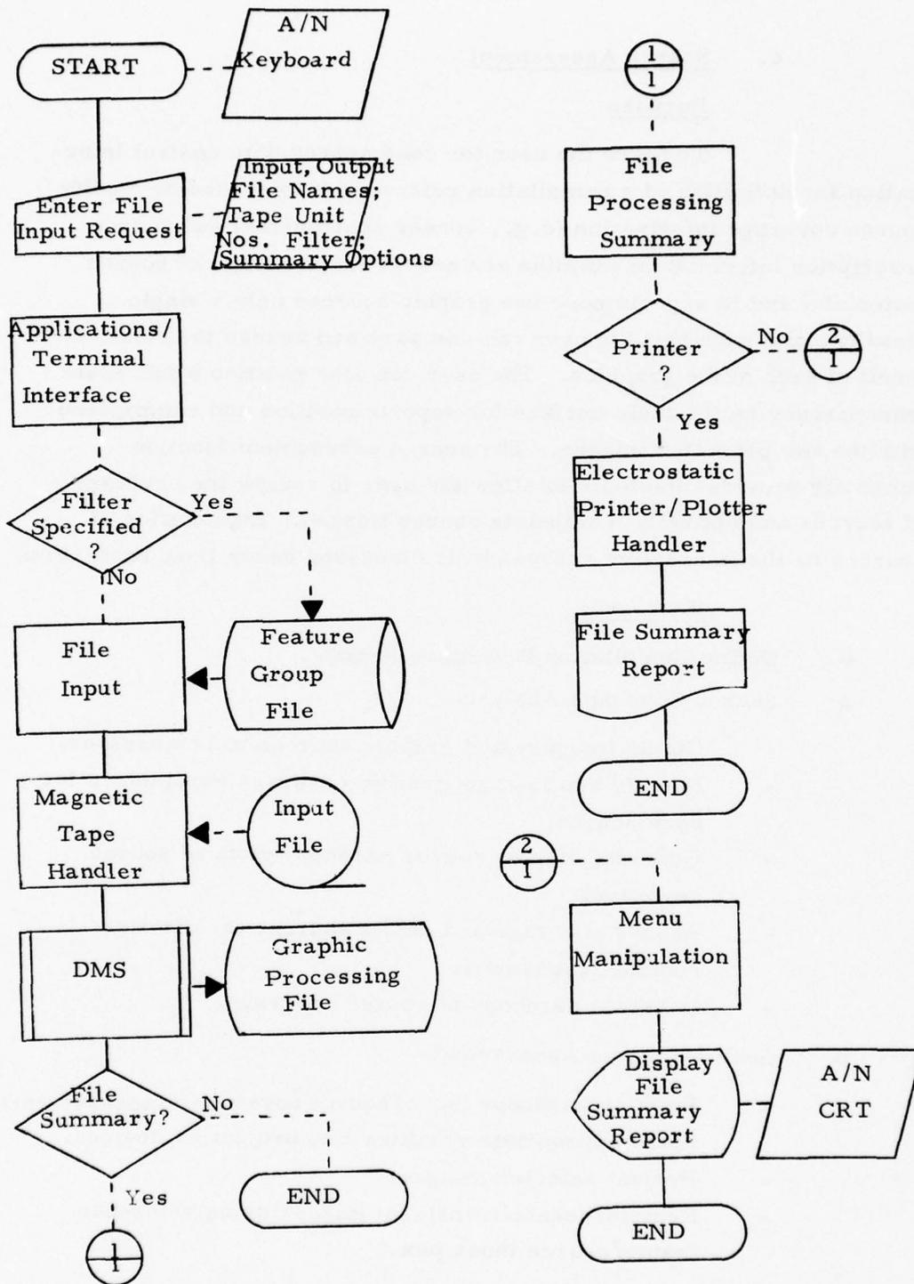
Figure III-20 - Input Processing Flow
