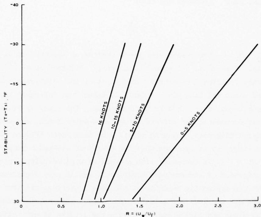
Figure 9. Characteristics of the ratio of overlake wind velocities to overlake velocities for various wind speed classes as a function of air-water temperature (after Richards et al.<sup>10</sup>)
