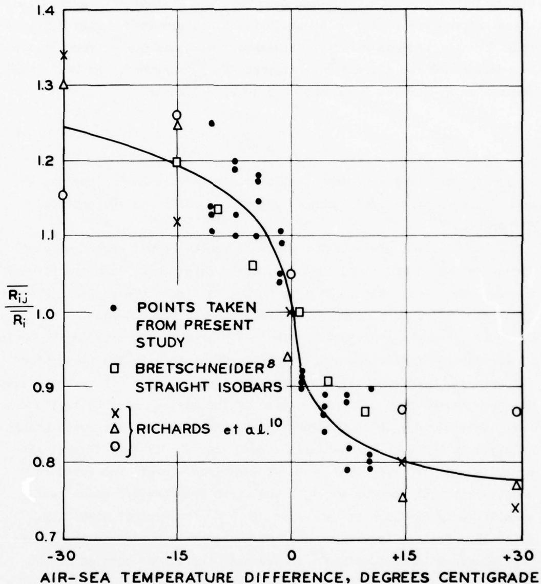
Figure 11. Comparison of empirical results of Richards et al.,<sup>10</sup> Bretschneider,<sup>8</sup> and the present study. The data of Richards et al. and Bretschneider were normalized to 1 at neutral
