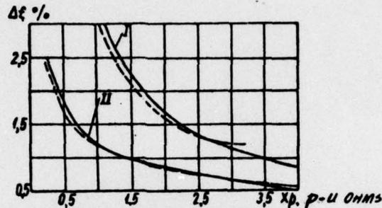
Fig. 4. Dependence of critical frequency difference on the resistance of a reactor during synchronization (design curves are shown by broken line).
