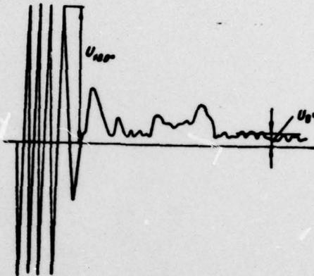
Fig. 5. Oscillogram of the process of regulation of the angle between the direction vectors of type GPCh-12/400 generators.
