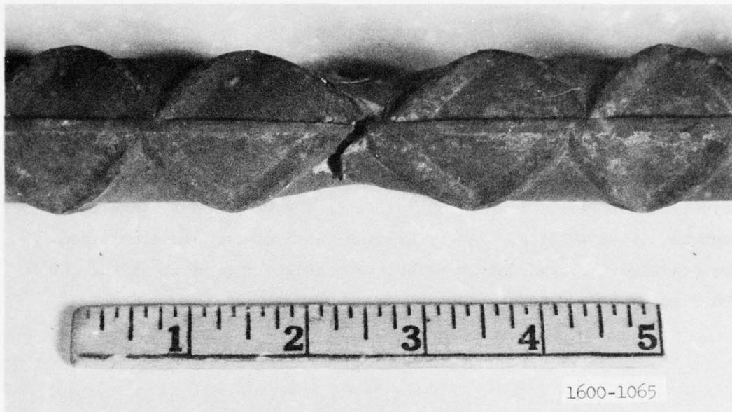
Figure 3.26 Typical ductile type fracture of No. 11 rebar.
