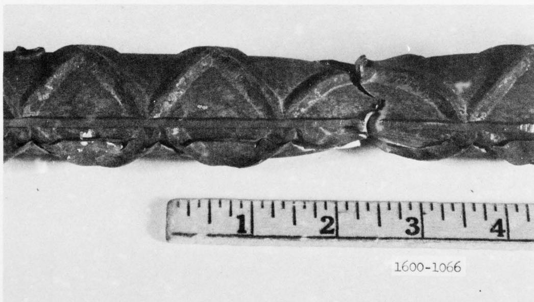
Figure 3.27 Posttest view of typical longitudinal flaw on No. 11 rebar.
