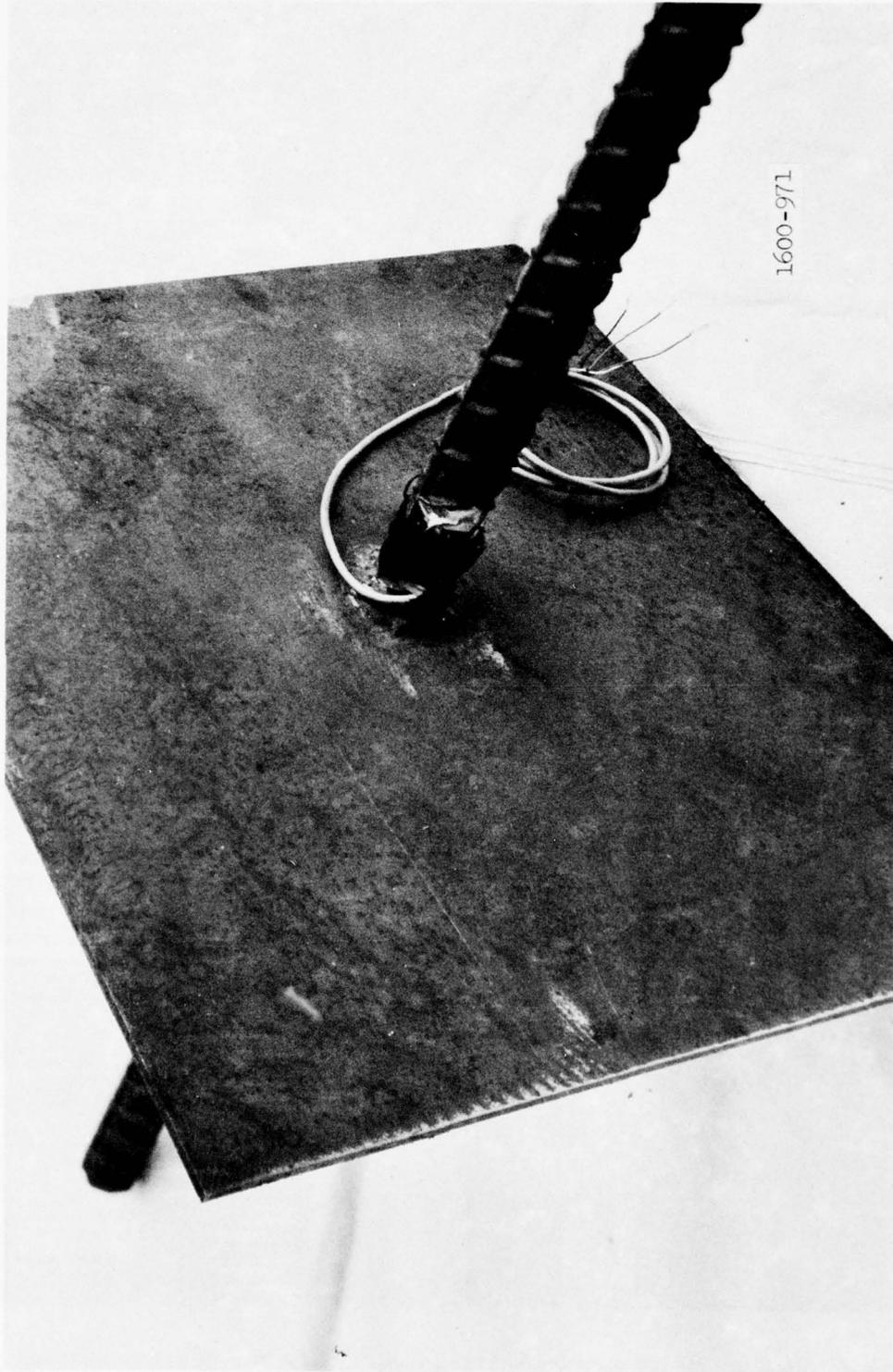
Figure 2.3 Pretest view of sample bar penetrating and welded to 1/4-inch-thick steel plate.
