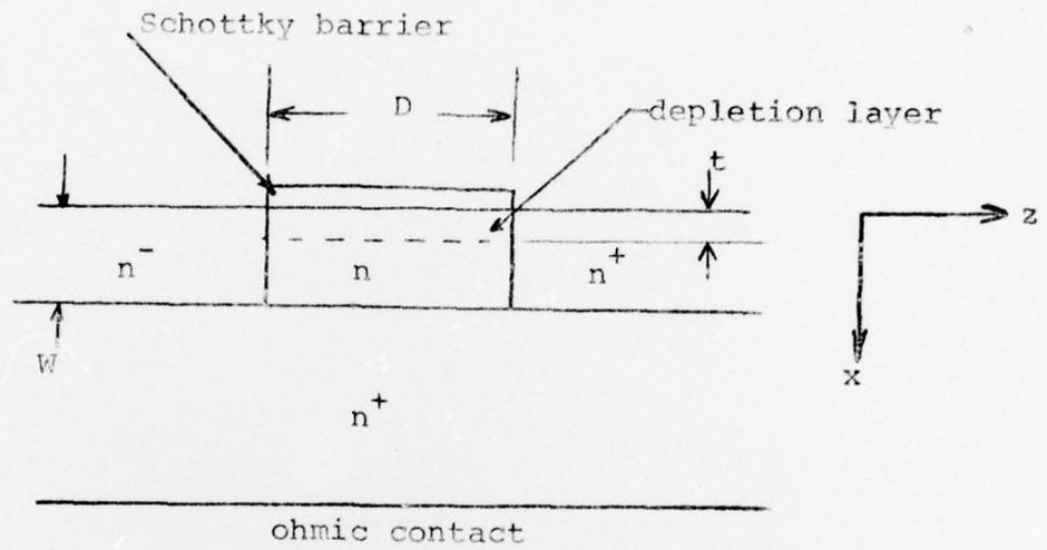
Fig. 2 The Idealized Structure for Analysis
