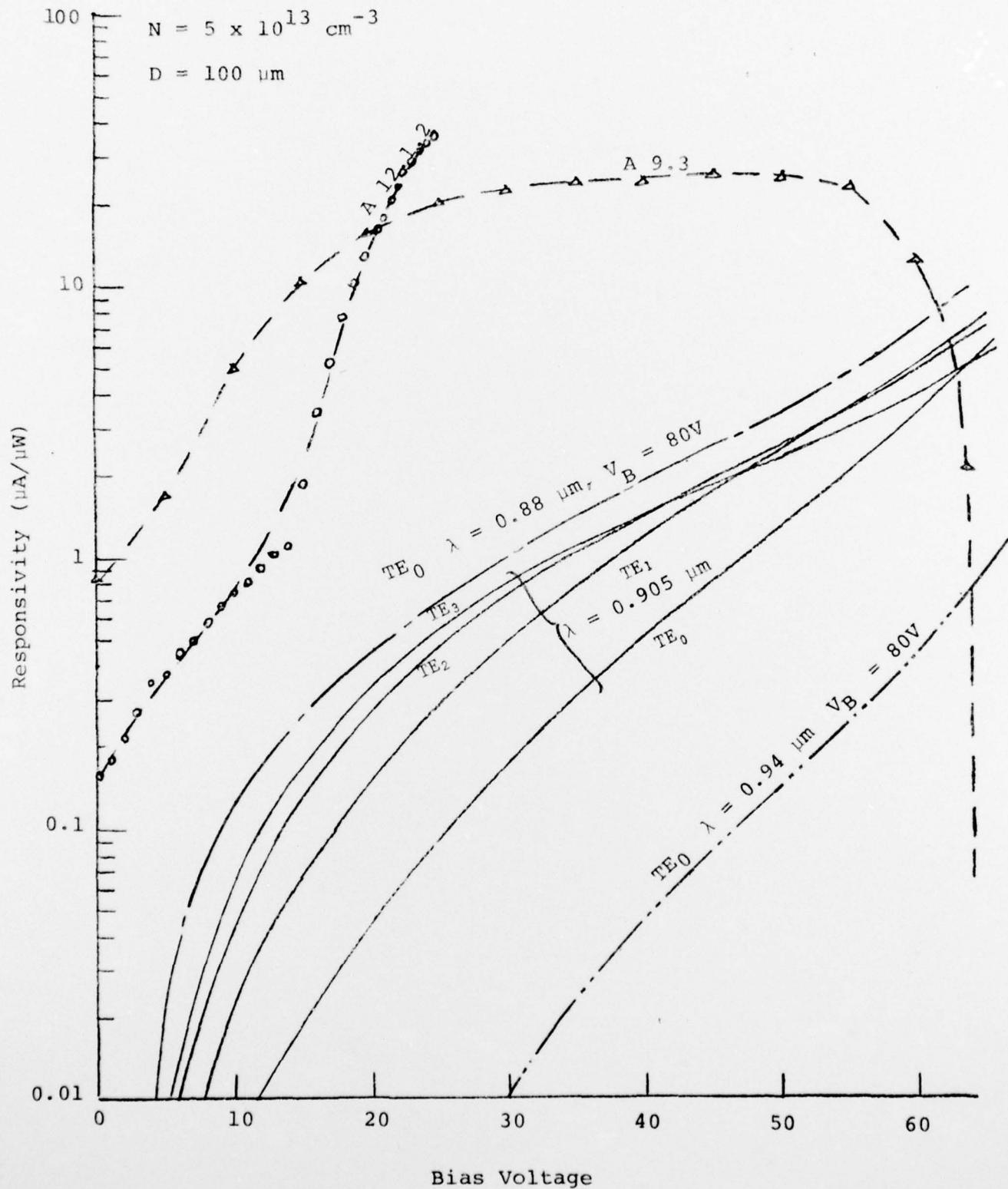
Fig. 4 The Responsivity of the EAP Waveguide Detectors
