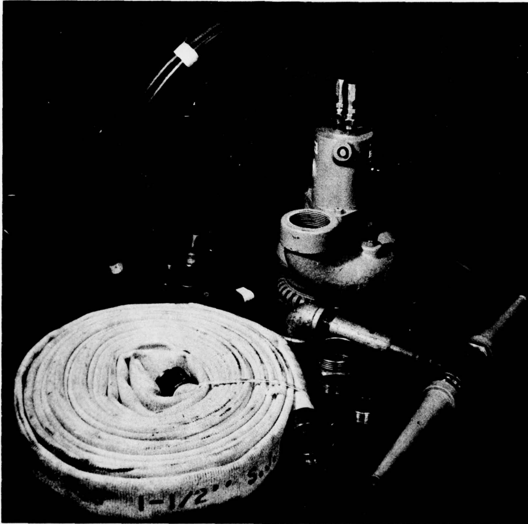
FIGURE 3-10. HYDRAULIC SUMP/JETTING PUMP, STANLEY
