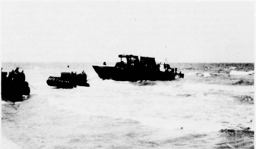
Figure D-4. P&H 6250-TC crane upper works on trailer being delivered to beach in LCM-8.
