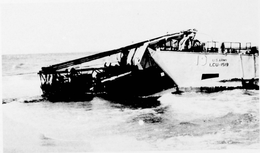
Figure D-1. P&H 9125-TC crane (tactically disassembled ) being delivered to beach in LCU.
