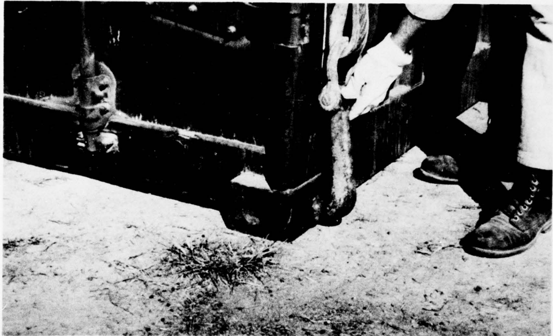
Figure 20. Modified bulb hook on sling spreader being inserted into corner fitting of container.
