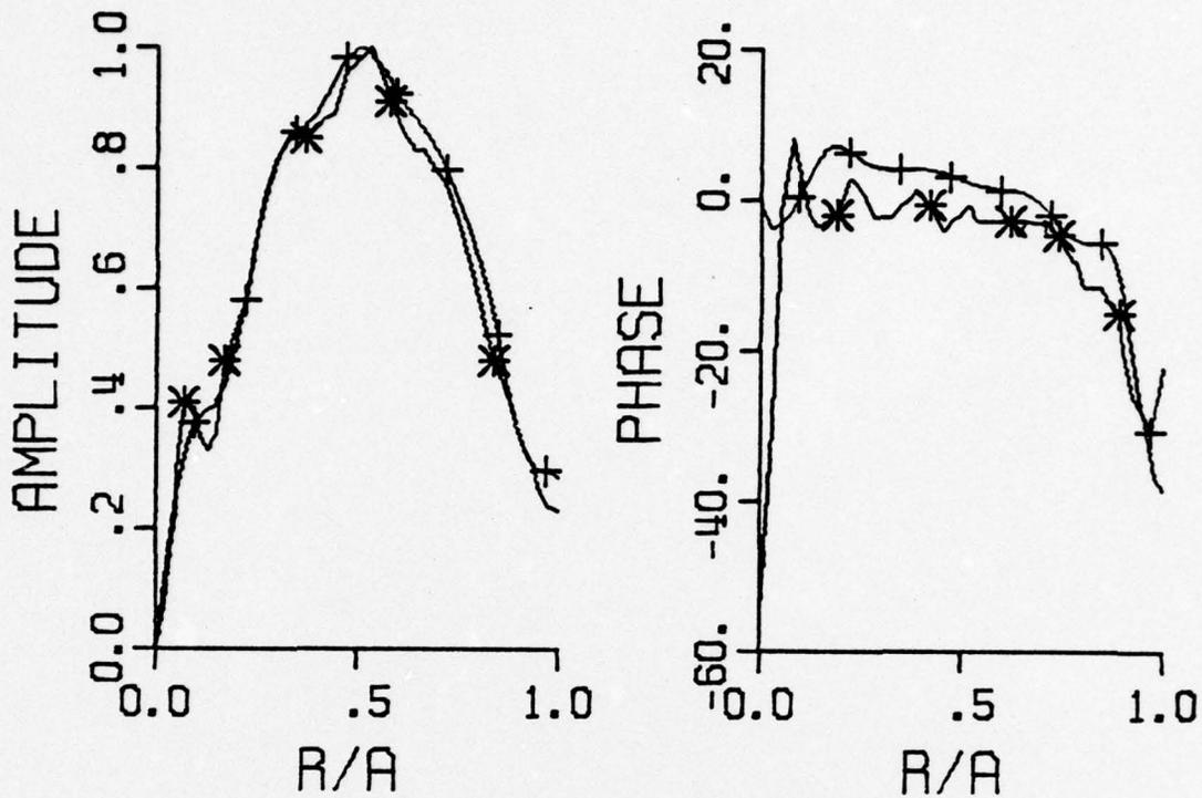
Figure 18. Relative Amplitude and Phase Distributions for the Lowest Loss,  $n = 1$  Mode
