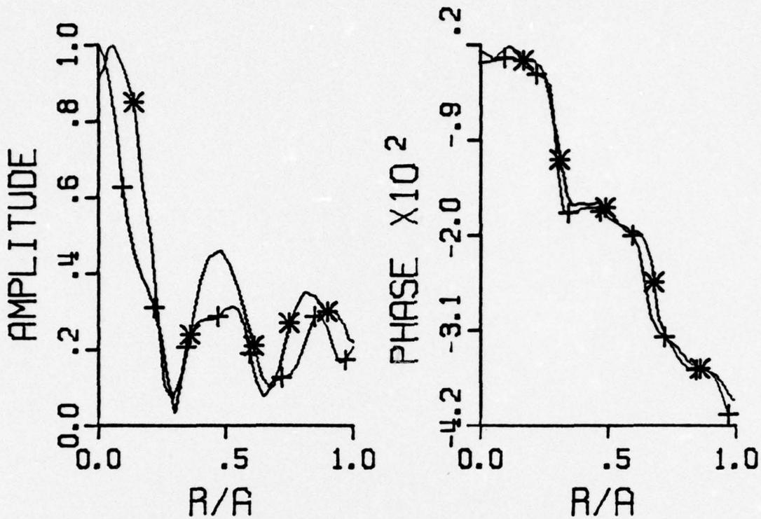
Figure 16. Relative Amplitude and Phase Distributions for the Third Lowest Loss,  $n = 0$  Mode
