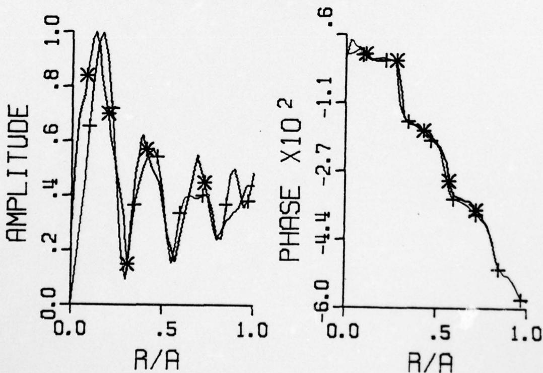
Figure 21. Relative Amplitude and Phase Distributions for the Fourth Lowest Loss,  $n = 1$  Mode
