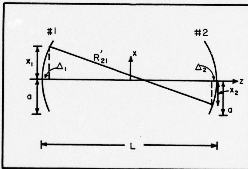
Figure 14. Geometry of a Spherical Resonator with Rectangular Mirrors
