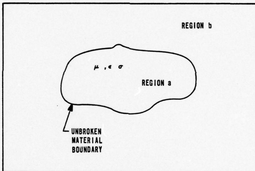
Figure 4. A Closed Resonator
