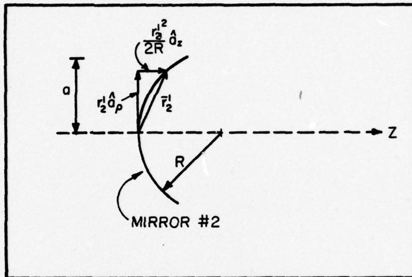
Figure 12. The Geometry of a Large Radius of Curvature Mirror
