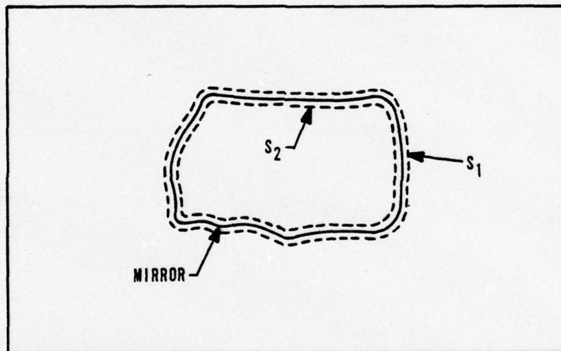
Figure 1. A Planar View of a Closed Resonator
