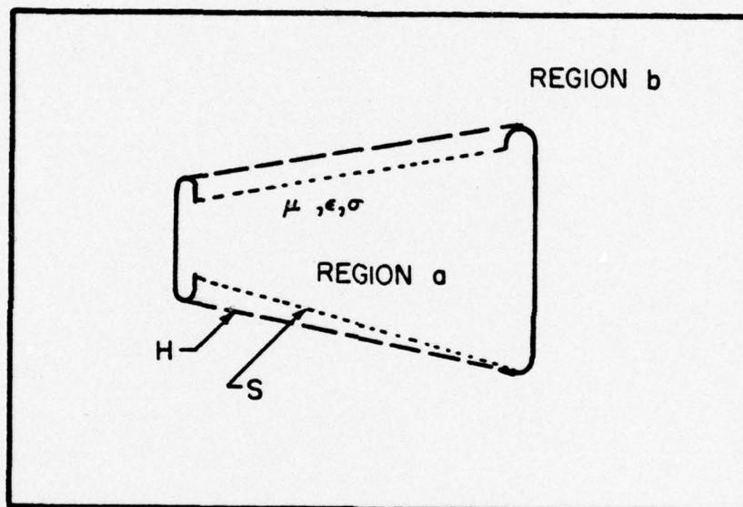
Figure 5. Surfaces Defining the Inside and Outside of an Open Resonator
