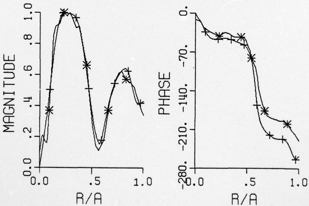
Figure 19. Relative Magnitude and Phase Distributions for the Second Lowest Loss,  $n = 1$  Mode
