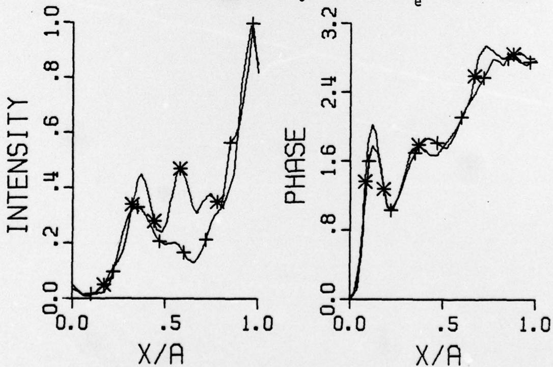
Figure 28. Relative Distributions for the Second Lowest Loss Mode with  $g = 1.8$  and  $2\pi N_e = 40$
