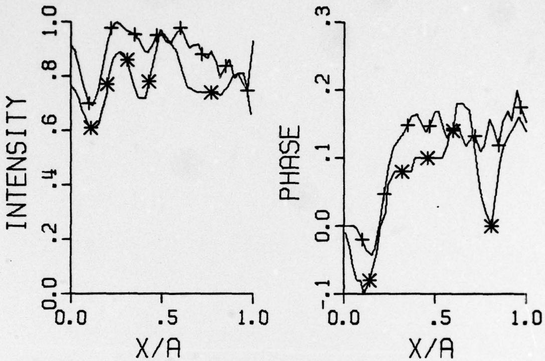
Figure 25. Relative Distributions for the Lowest Loss Mode with  $g = 1.8$  and  $2\pi N_e = 36$
