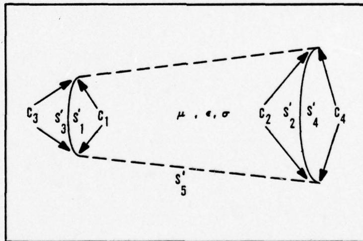
Figure 7. A Plane View of the Surfaces of an Open Resonator
