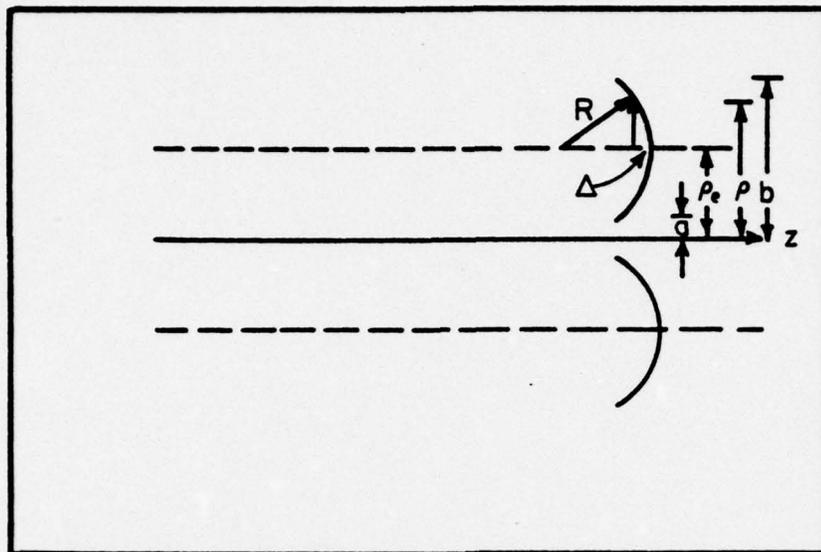
Figure 15. Intersection of a Toroidal Mirror With the x-z Plane
