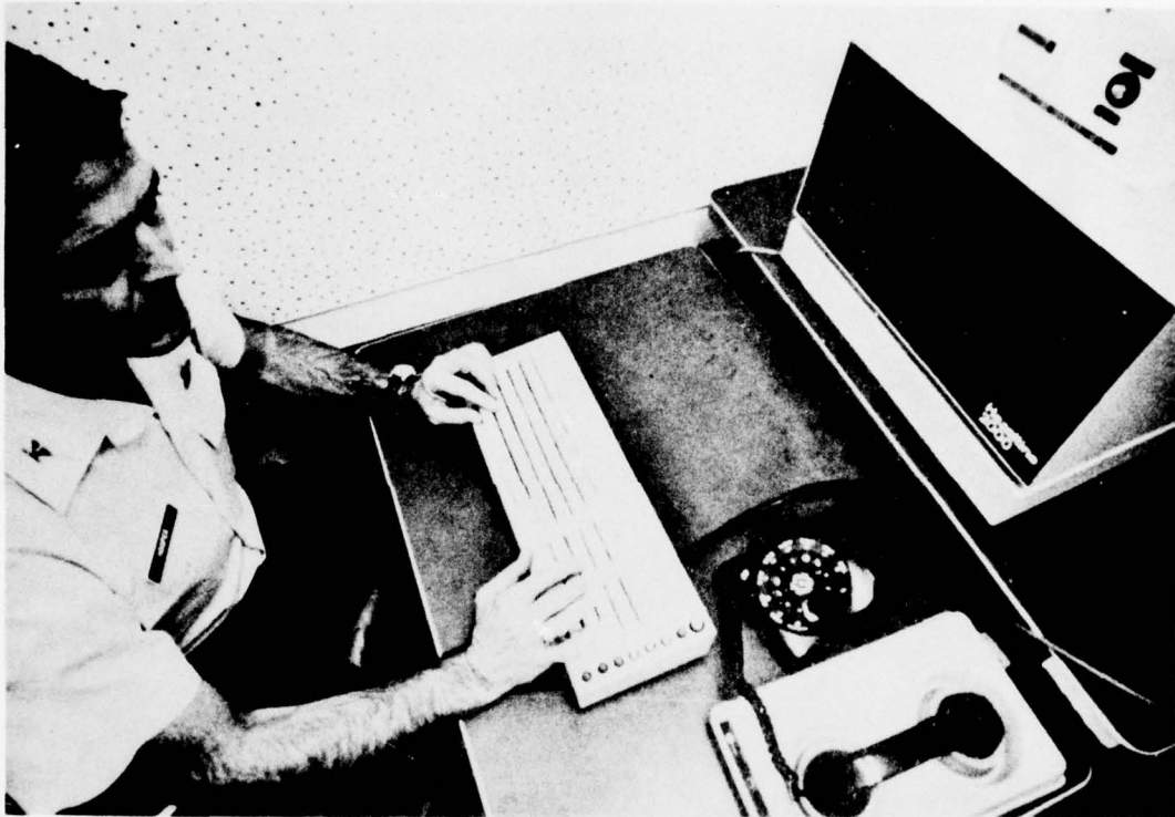
Fig. 20. An Air War College student enters data for the force posture planning model phase of the National Security Study using a Hazeltine 2000 cathode-ray tube terminal which is on-line to a Honeywell 6060 computer.
