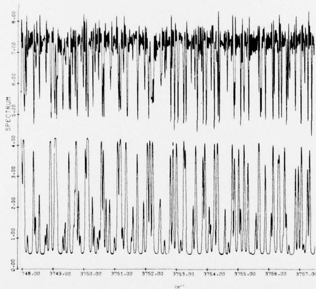
Figure 27. CO<sub>2</sub> Hot Cell Spectrum (upper curve) and Simulated Spectrum (lower curve), 3748 - 3757 cm<sup>-1</sup>
