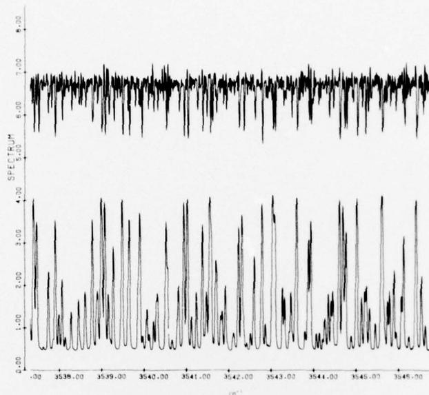
Figure 10. CO<sub>2</sub> Hot Cell Spectrum (upper curve) and Simulated Spectrum (lower curve), 3538 - 3546 cm<sup>-1</sup>
