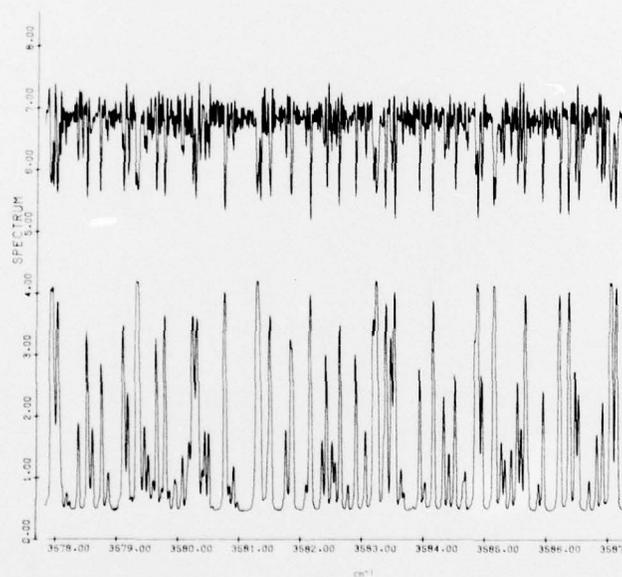
Figure 15. CO<sub>2</sub> Hot Cell Spectrum (upper curve) and Simulated Spectrum (lower curve), 3578 - 3587 cm<sup>-1</sup>
