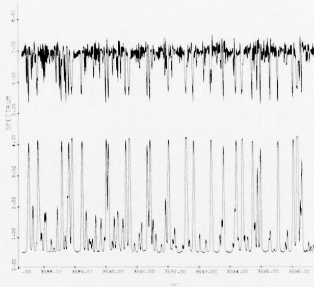
Figure 16. CO<sub>2</sub> Hot Cell Spectrum (upper curve) and Simulated Spectrum (lower curve), 3588 - 3596 cm<sup>-1</sup>
