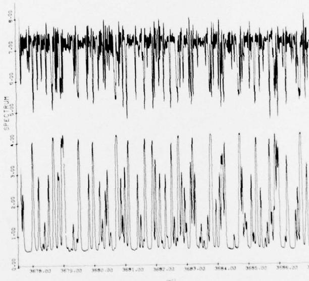
Figure 21. CO<sub>2</sub> Hot Cell Spectrum (upper curve) and Simulated Spectrum (lower curve), 3678 - 3686 cm<sup>-1</sup>
