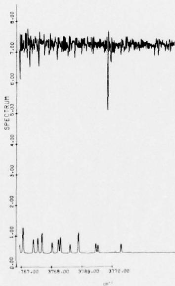
Figure 29. CO<sub>2</sub> Hot Cell Spectrum (upper curve) and Simulated Spectrum (lower curve), 3767 - 3770 cm<sup>-1</sup>
