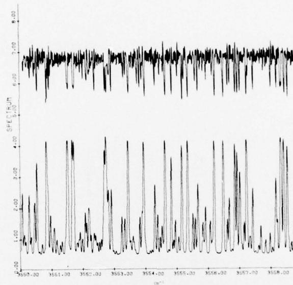
Figure 12. CO<sub>2</sub> Hot Cell Spectrum (upper curve) and Simulated Spectrum (lower curve), 3551 - 3558 cm<sup>-1</sup>
