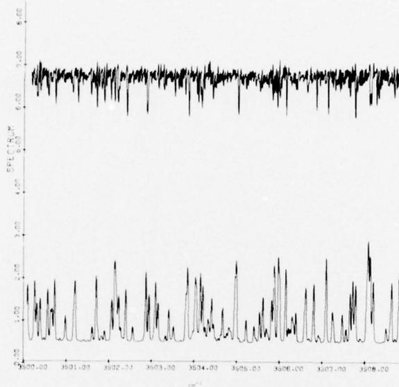
Figure 6. CO<sub>2</sub> Hot Cell Spectrum (upper curve) and Simulated Spectrum (lower curve), 3500 - 3508 cm<sup>-1</sup>
