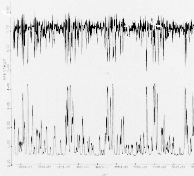
Figure 19. CO<sub>2</sub> Hot Cell Spectrum (upper curve) and Simulated Spectrum (lower curve), 3659 - 3667 cm<sup>-1</sup>
