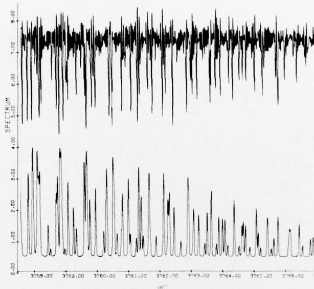
Figure 28. CO<sub>2</sub> Hot Cell Spectrum (upper curve) and Simulated Spectrum (lower curve), 3758 - 3766 cm<sup>-1</sup>
