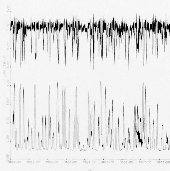
Figure 18. CO<sub>2</sub> Hot Cell Spectrum (upper curve) and Simulated Spectrum (lower curve), 3650 - 3658 cm<sup>-1</sup>
