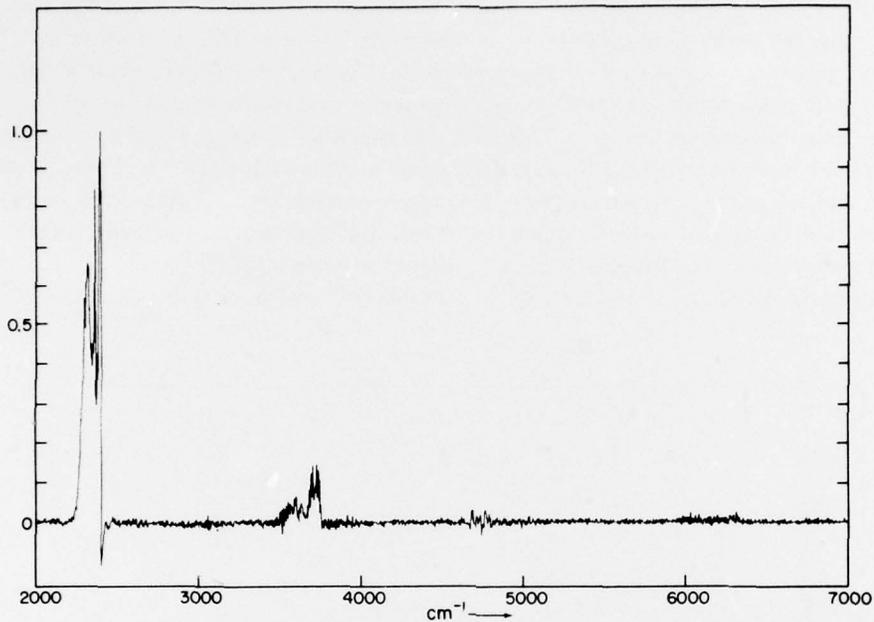
Figure 4. CO<sub>2</sub> Hot Cell Spectrum: Resolution 1.9 cm<sup>-1</sup>, Gas Temperature 625°K, Background Subtracted
