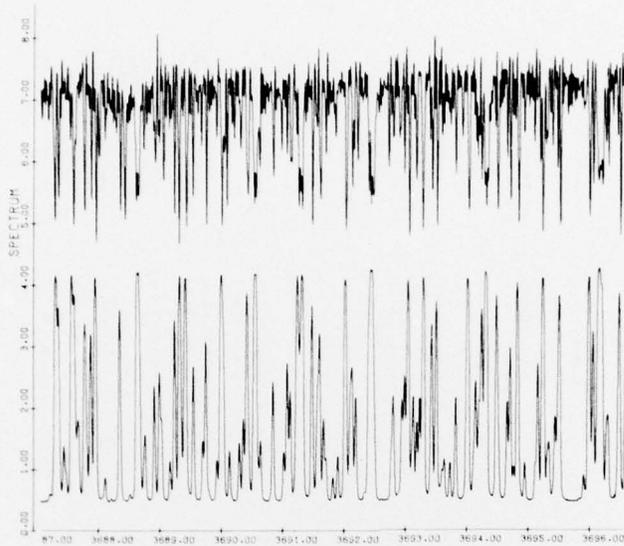
Figure 22. CO<sub>2</sub> Hot Cell Spectrum (upper curve) and Simulated Spectrum (lower curve), 3687 - 3696 cm<sup>-1</sup>
