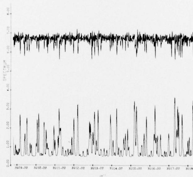
Figure 7. CO<sub>2</sub> Hot Cell Spectrum (upper curve) and Simulated Spectrum (lower curve), 3509 - 3518 cm<sup>-1</sup>
