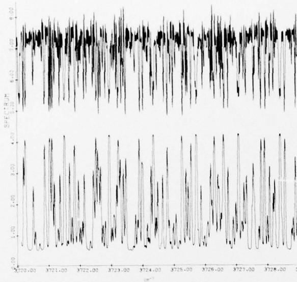
Figure 24. CO<sub>2</sub> Hot Cell Spectrum (upper curve) and Simulated Spectrum (lower curve), 3720 - 3728 cm<sup>-1</sup>
