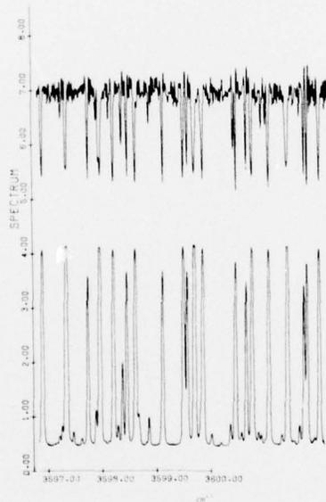
Figure 17. CO<sub>2</sub> Hot Cell Spectrum (upper curve), and Simulated Spectrum (lower curve), 3597 - 3600 cm<sup>-1</sup>
