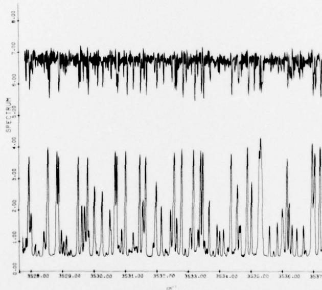
Figure 9. CO<sub>2</sub> Hot Cell Spectrum (upper curve) and Simulated Spectrum (lower curve), 3528 - 3537 cm<sup>-1</sup>
