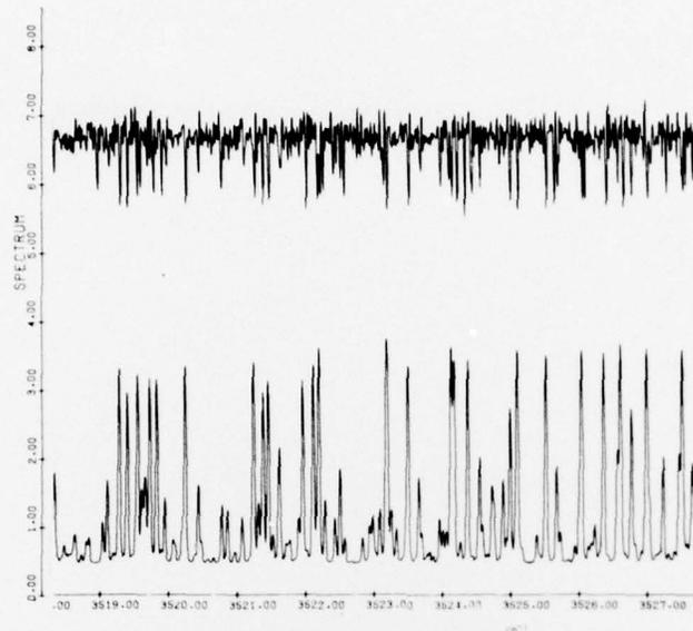
Figure 8. CO<sub>2</sub> Hot Cell Spectrum (upper curve) and Simulated Spectrum (lower curve), 3519 - 3527 cm<sup>-1</sup>
