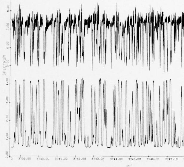
Figure 26. CO<sub>2</sub> Hot Cell Spectrum (upper curve) and Simulated Spectrum (lower curve), 3739 - 3747 cm<sup>-1</sup>
