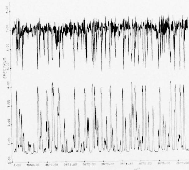
Figure 20. CO<sub>2</sub> Hot Cell Spectrum (upper curve) and Simulated Spectrum (lower curve), 3668 - 3677 cm<sup>-1</sup>
