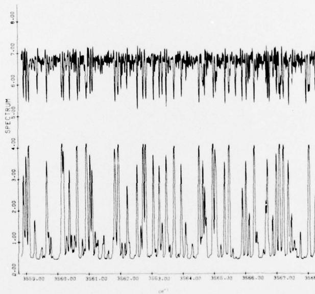
Figure 13. CO<sub>2</sub> Hot Cell Spectrum (upper curve) and Simulated Spectrum (lower curve), 3559 - 3568 cm<sup>-1</sup>
