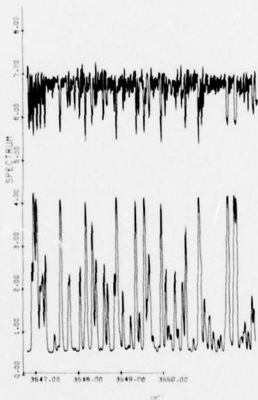
Figure 11. CO<sub>2</sub> Hot Cell Spectrum (upper curve) and Simulated Spectrum (lower curve), 3547 - 3550 cm<sup>-1</sup>
