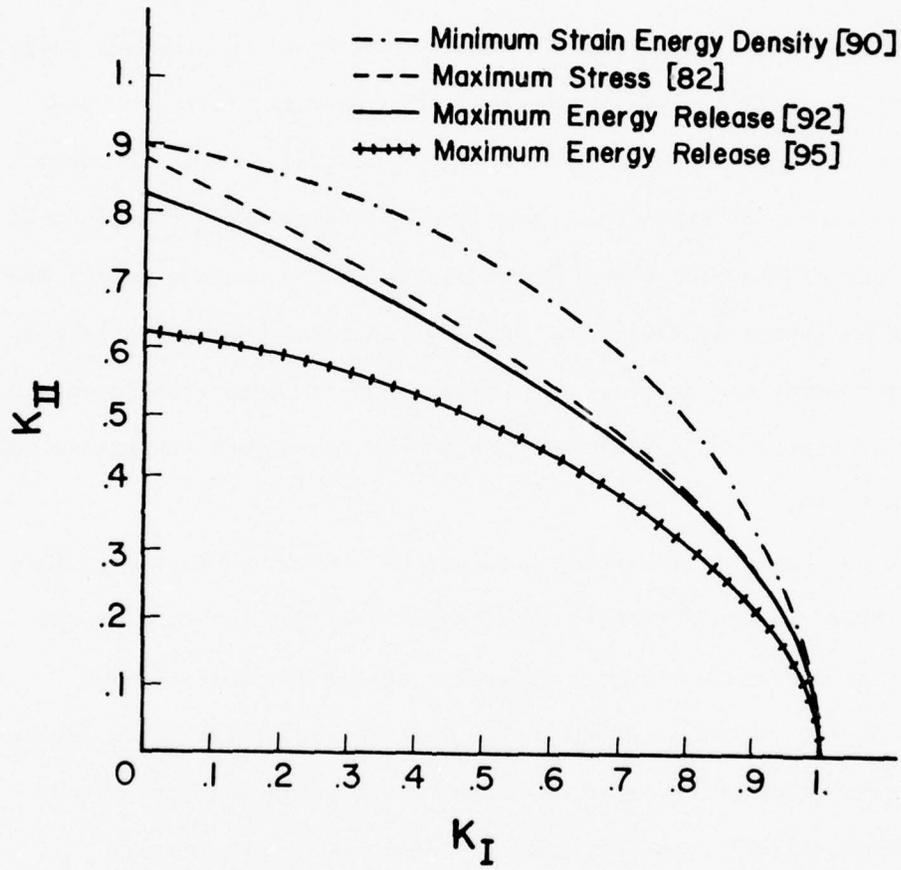
Figure 6. Interaction of  $K_I$  and  $K_{II}$  for various criteria.
