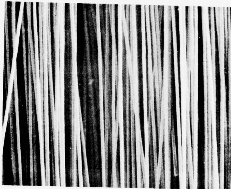
Figure 1. Fibrous composite, HT-S/ERLA 2256 (300X).
