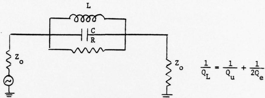
Figure 7. Equivalent Circuit for a Single Resonator Bandstop Filter.
