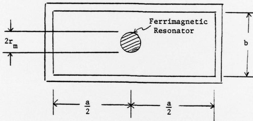
Figure 5.  $TE_{10}$  Waveguide
