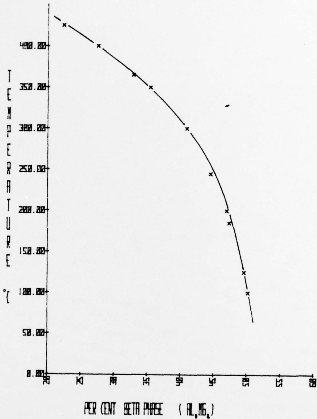
Figure 26 - TEMPERATURE VS. PERCENTAGE BETA PHASE INTERMETALLIC.
