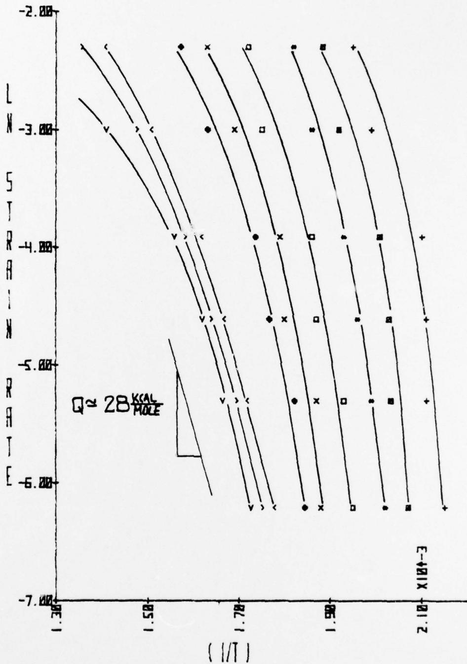
Figure 25 - NATURAL LOG OF STRAIN RATE VS. RECIPROCAL ABSOLUTE TEMPERATURE FOR VARIOUS VALUES OF  $(\sigma/E)$ .
