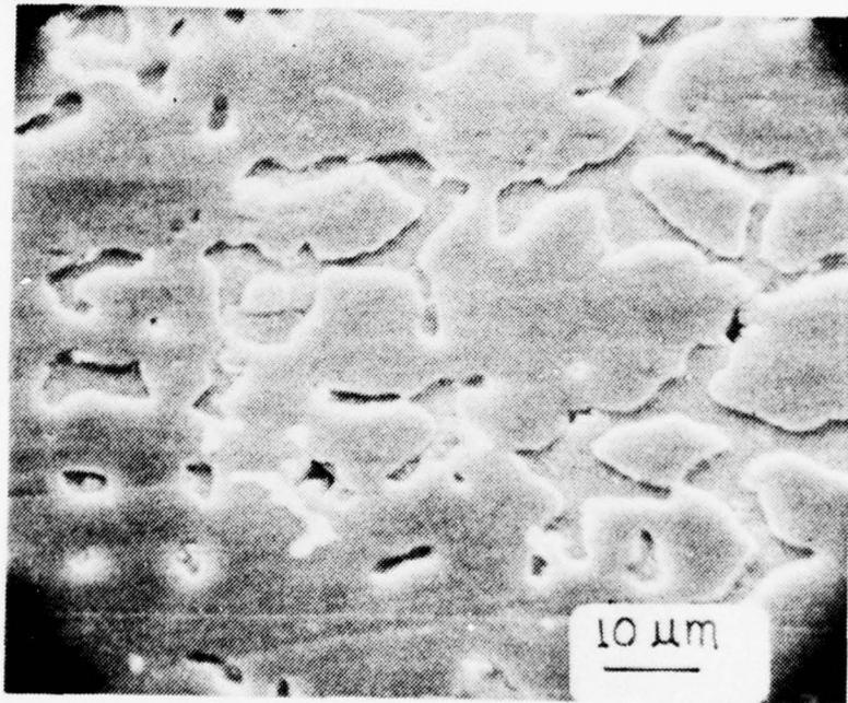
Figure 10 - SEM PHOTOGRAPH #1 OF AS CAST MATERIAL, 1,200X.
