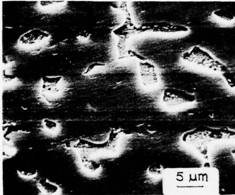
Figure 13 - SEM PHOTOGRAPH #1 OF AS CAST MATERIAL, 2,400X.
