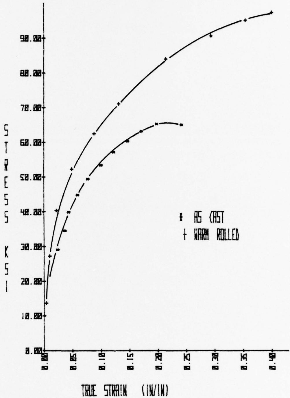
Figure 19 - TRUE STRESS VS. TRUE STRAIN FOR AS CAST (\*) AND WARM ROLLED (+) MATERIAL.
