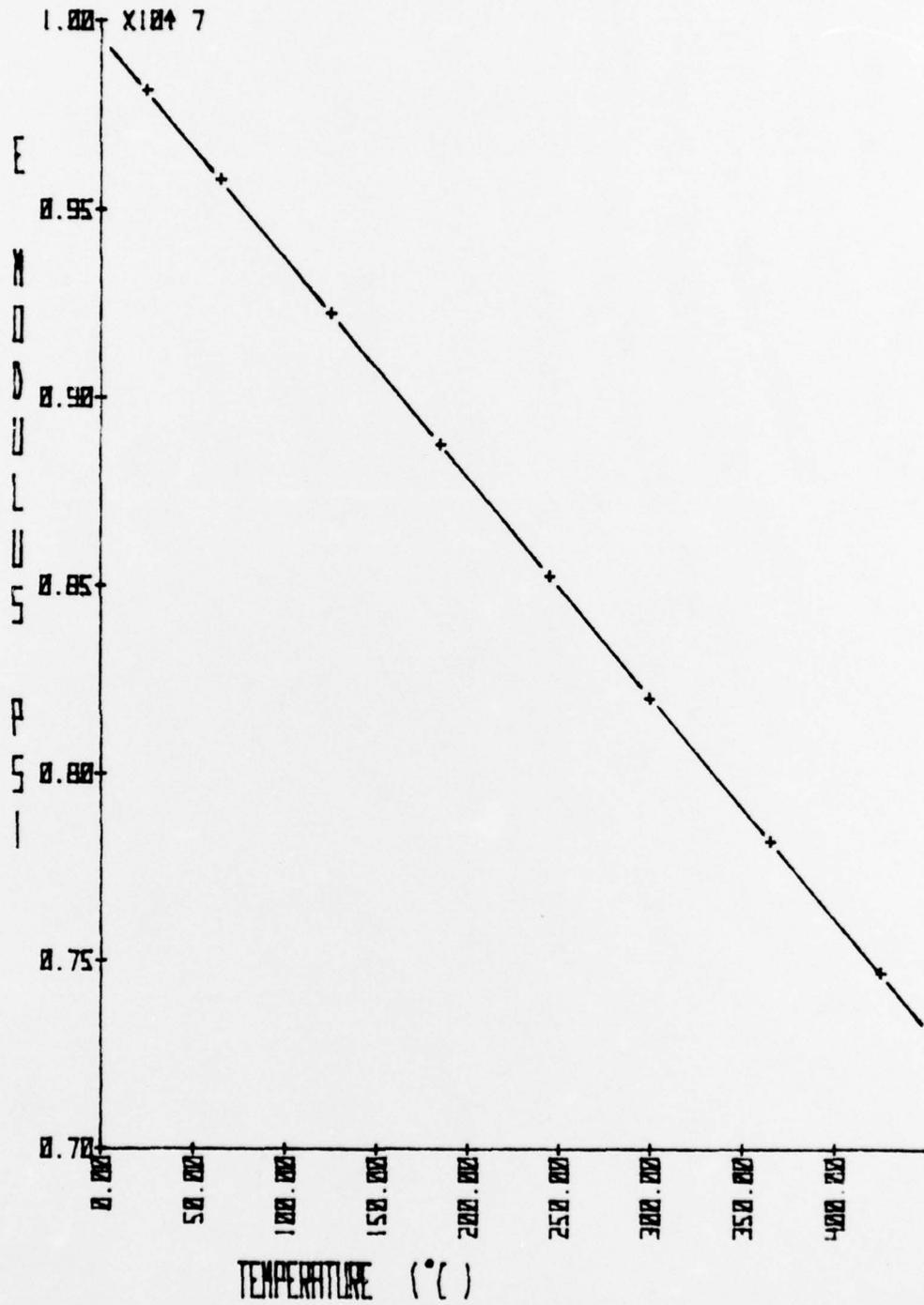
Figure 24 - ELASTIC MODULUS (E) VS. TEMPERATURE, (11).
