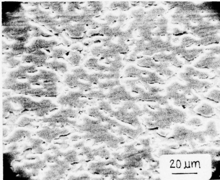
Figure 9 - SEM PHOTOGRAPH OF AS CAST MATERIAL, 610X.
