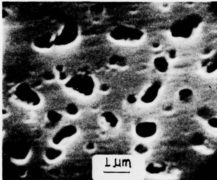
Figure 30 - SEM PHOTOGRAPH OF A WARM ROLLED SPECIMEN
