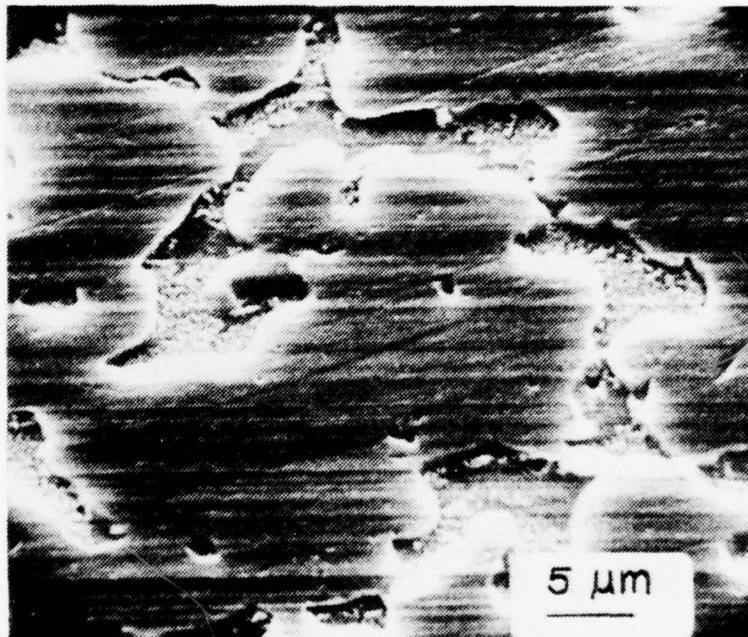
Figure 14 - SEM PHOTOGRAPH #2 OF AS CAST MATERIAL, 2,400X.
