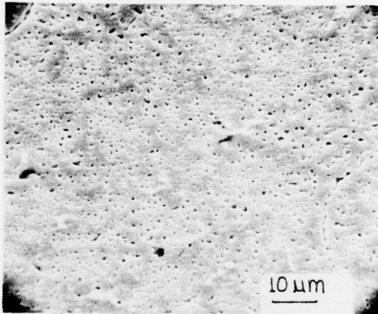
Figure 27 - SEM PHOTOGRAPH OF A WARM ROLLED SPECIMEN
