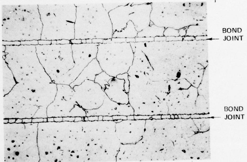
Figure 45. Optical Micrograph of Cylinder M3 Showing Laminate Joint Irregularity at the Periphery of the Large Stack in the As-Bonded Condition. (Kallings Etch) (Mag.: 100X)
