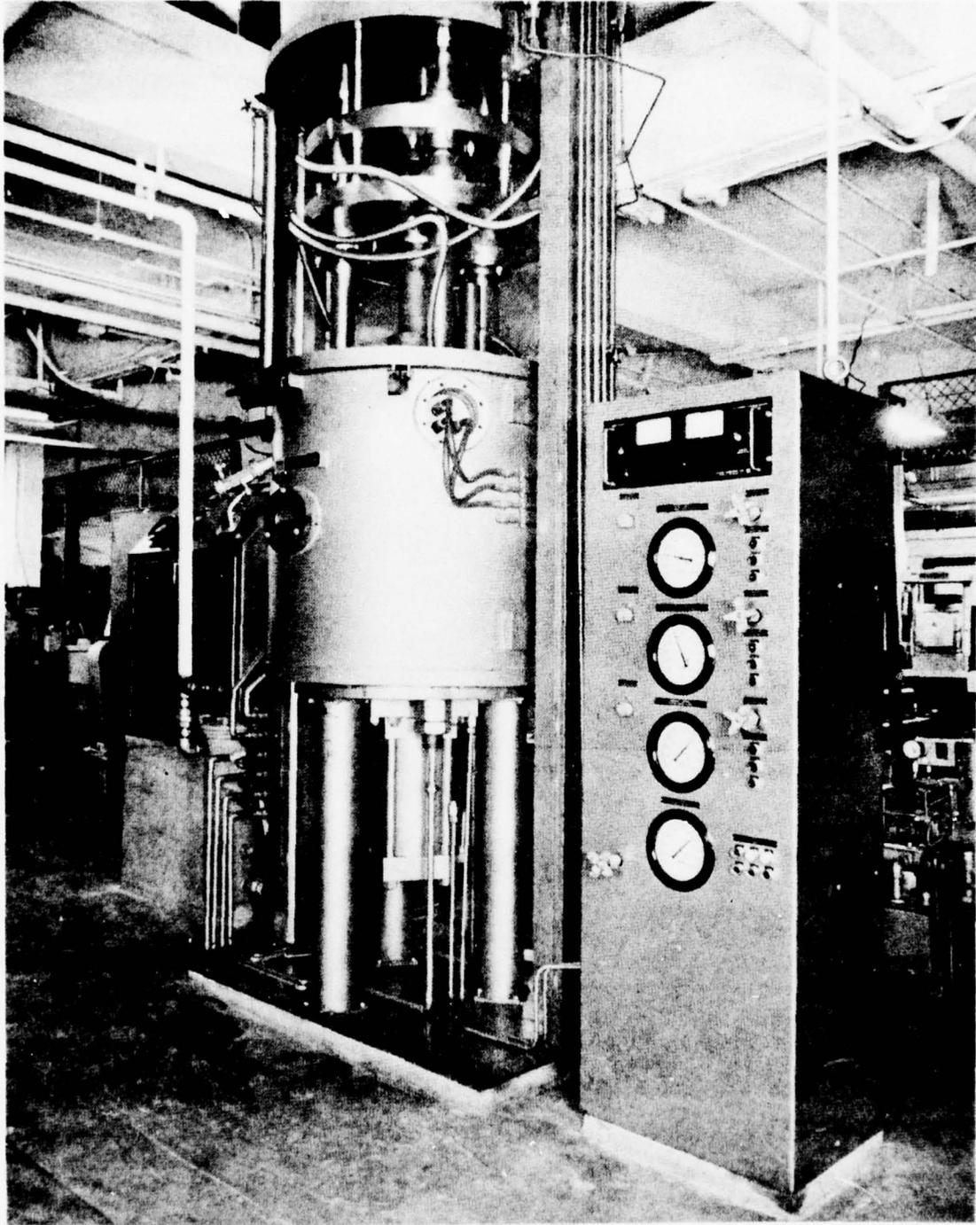
Figure 41. Bonding Facility - 75-Ton Capacity Vacuum Hot-Press Furnace.
