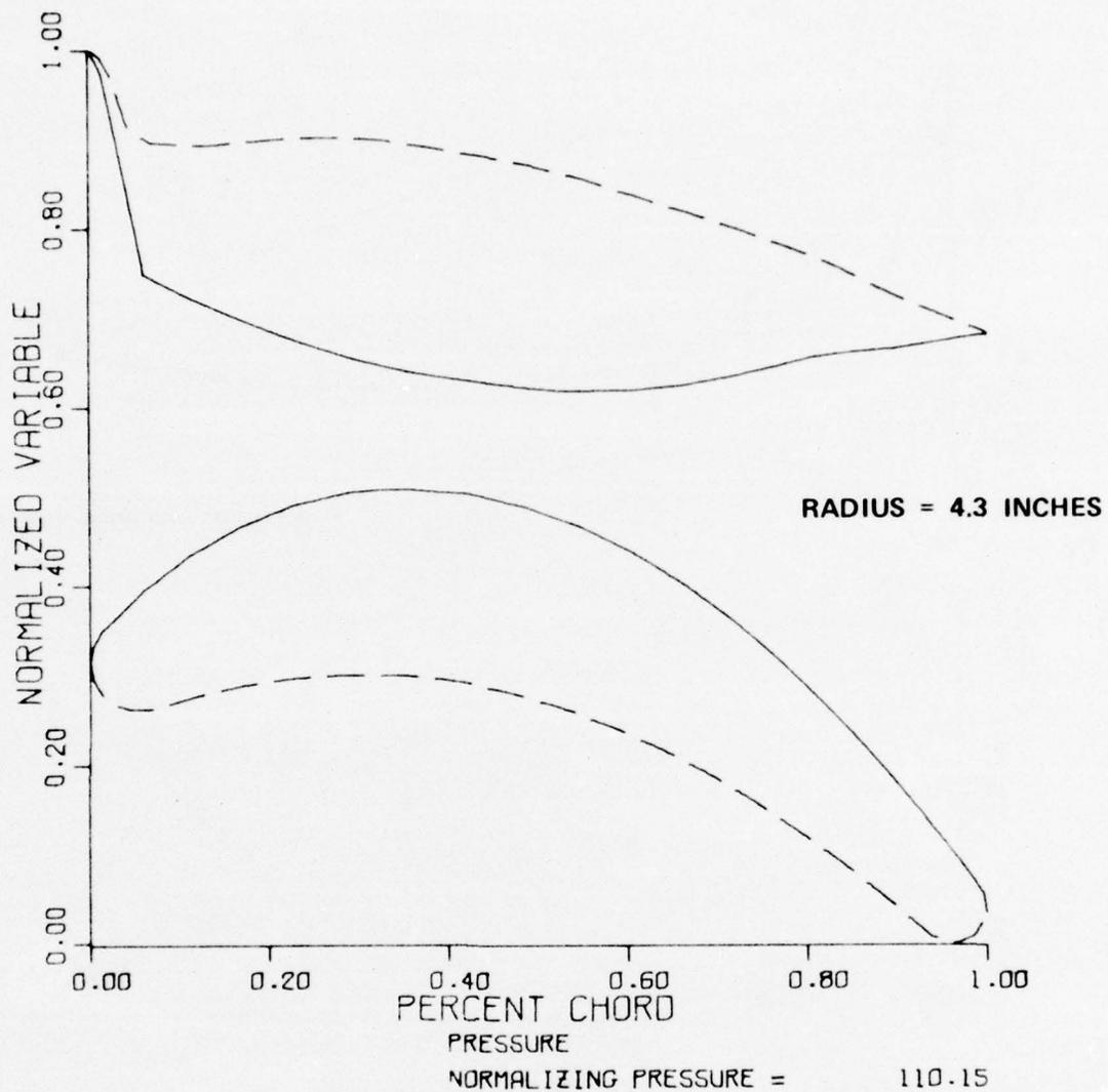
Figure 21. (a) High-Temperature Laminated Blade-Surface Static Pressures for Five Sections. (TIT Average = 2600°F, and  $P_{T_{IN}} = 152.5$  PSIA)
