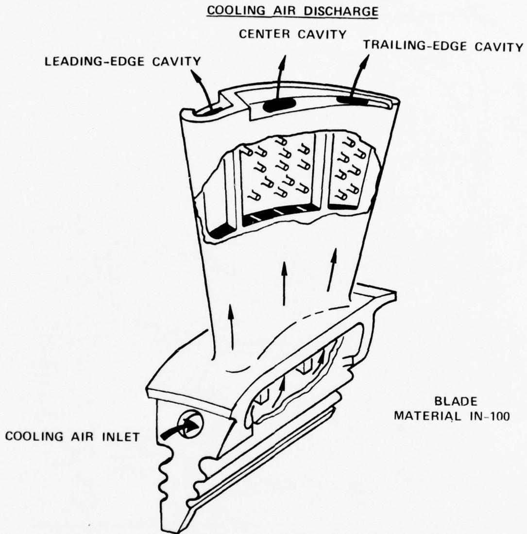
Figure 9. Air-Cooled TFE731-3 High-Pressure Turbine Blade.
