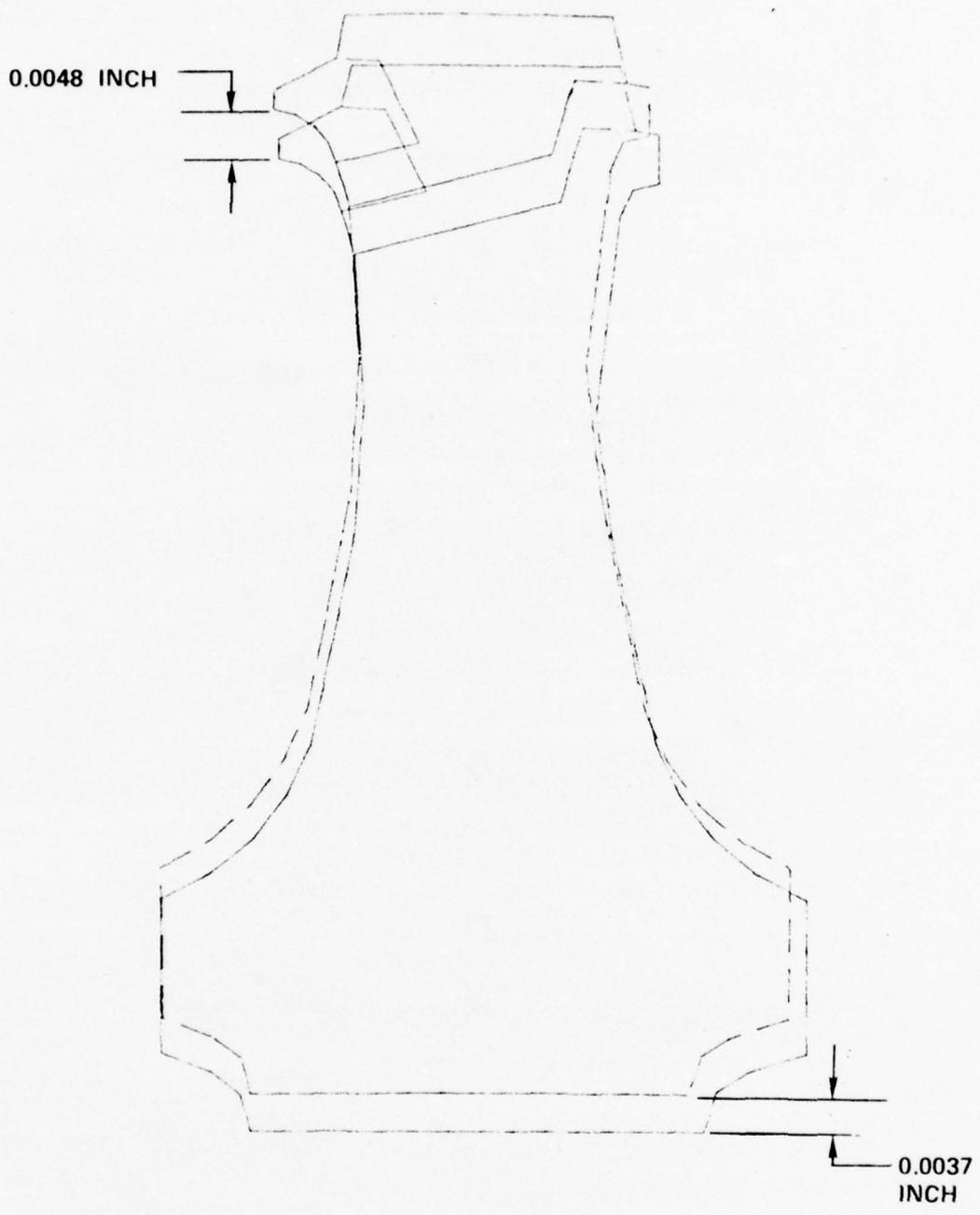
Figure 14. Laminated Turbine Disk Magnified Displacement Due to Centrifugal Loading Only (29,692 RPM).
