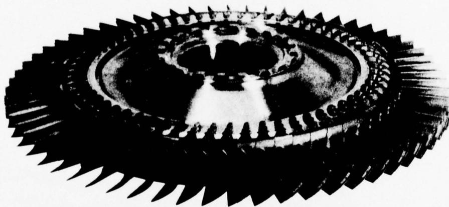
Figure 2. AiResearch Model TFE731-3 Cooled Turbine Wheel
