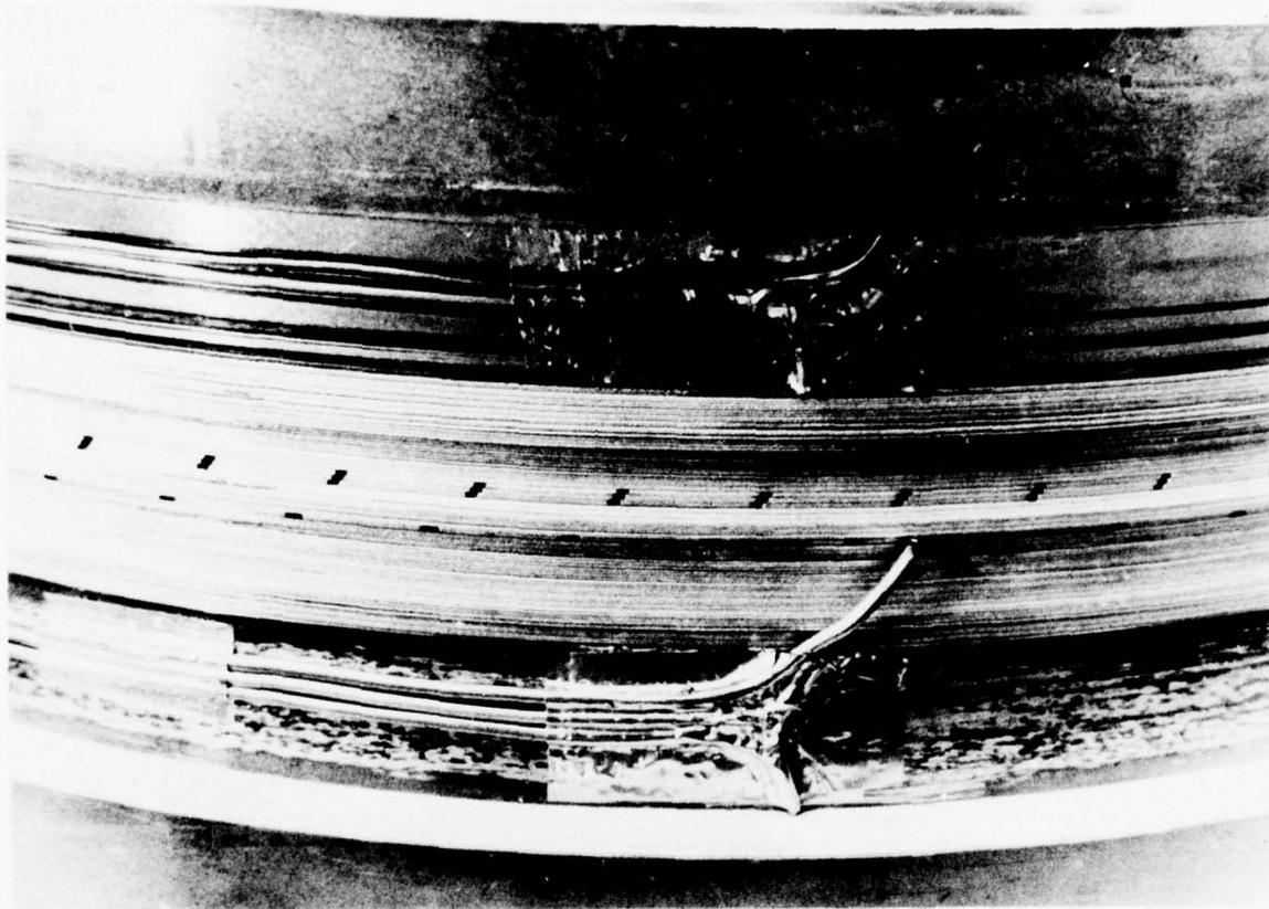
Figure 56. Sequentially Assembled Wheel Blank Laminates on the Bond Fixture with the Thermocouples Installed.
