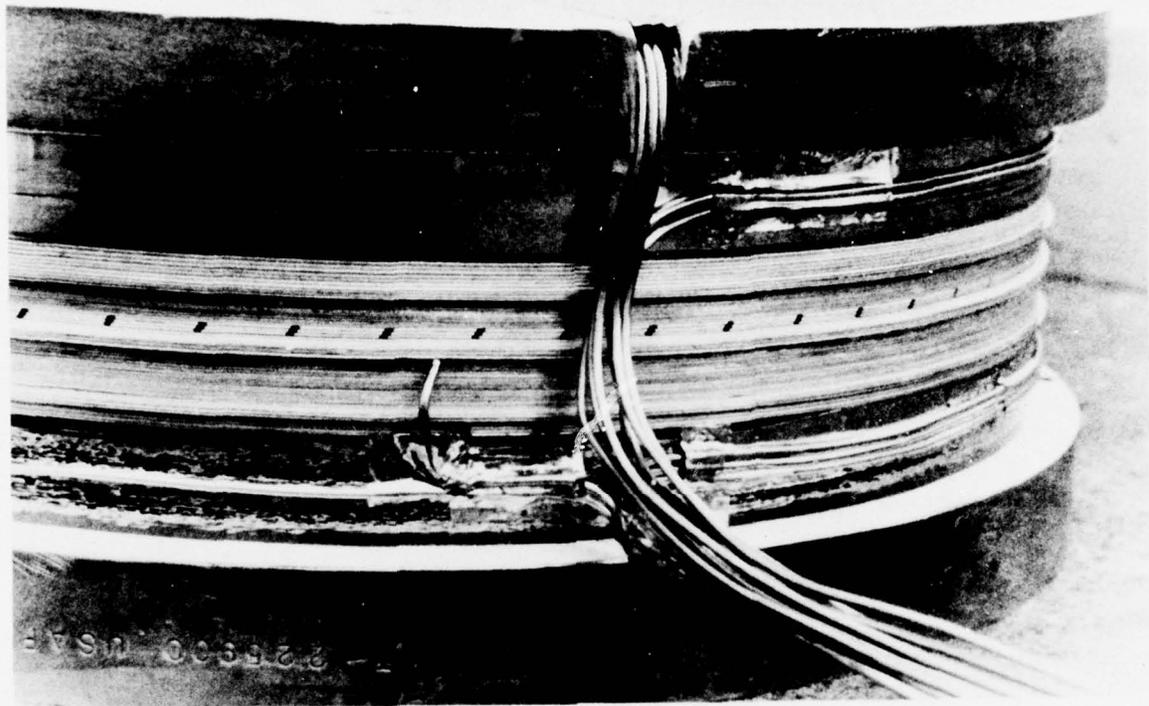
Figure 57. Sequentially Assembled Wheel Blank Laminates on the Bond Fixture with the Thermocouples Installed.
