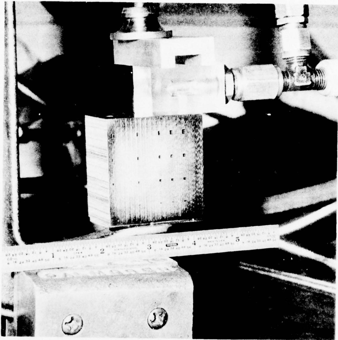
Figure 37. Test Setup for Laminate Sheet Stack Airflow Tests.
