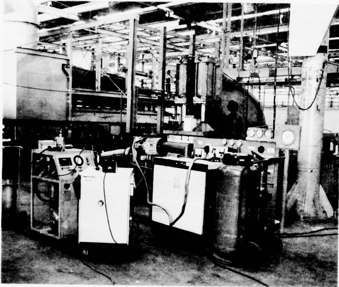
Figure 62. Completed Laminate Wheel Blank Bonding Assembly in the Hot Press, and Connected to the Vacuum System of the Rockwell International Facility.
