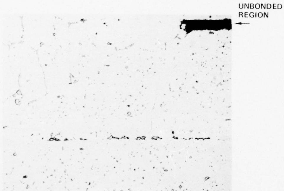
Figure 44. Optical Micrograph of Cylinder M1 Showing an Unbonded Region Between the End Plate and the Adjacent Lamination. This Region Appeared as a Sonic Indication on the C-Scan Recording in Figure 43. (Kallings Etch) (Mag.: 100X)
