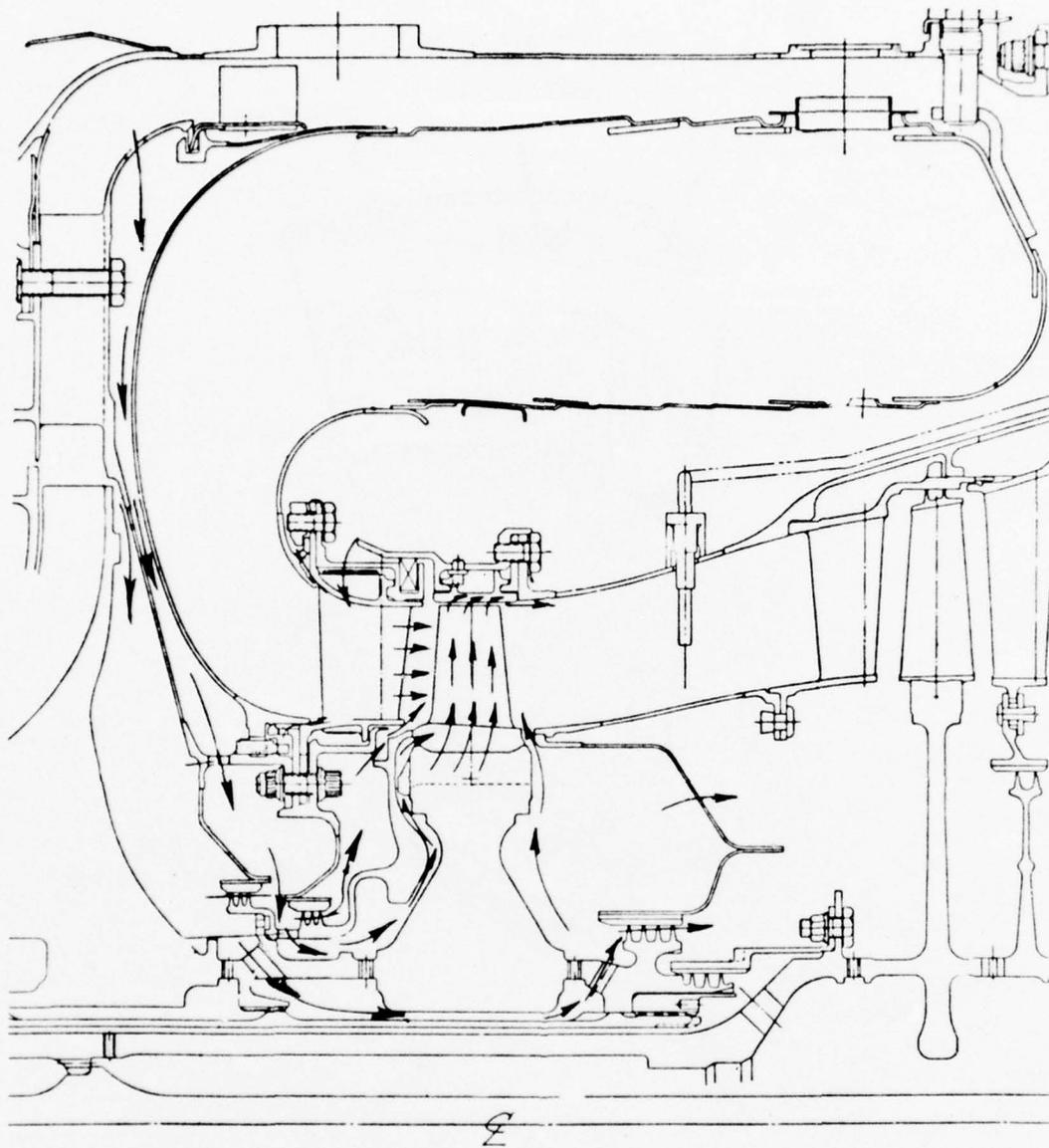
Figure 10. TFE731-3 Secondary Cooling Airflow System
