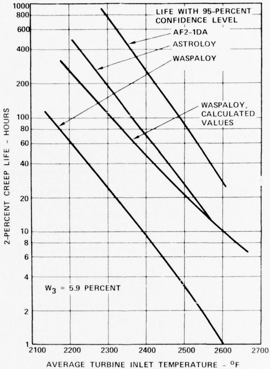
Figure 29. Laminate Turbine Blade Critical Section (R = 4.6095 Inches) 2-Percent Creep Life Versus Average Turbine Inlet Temperature.
