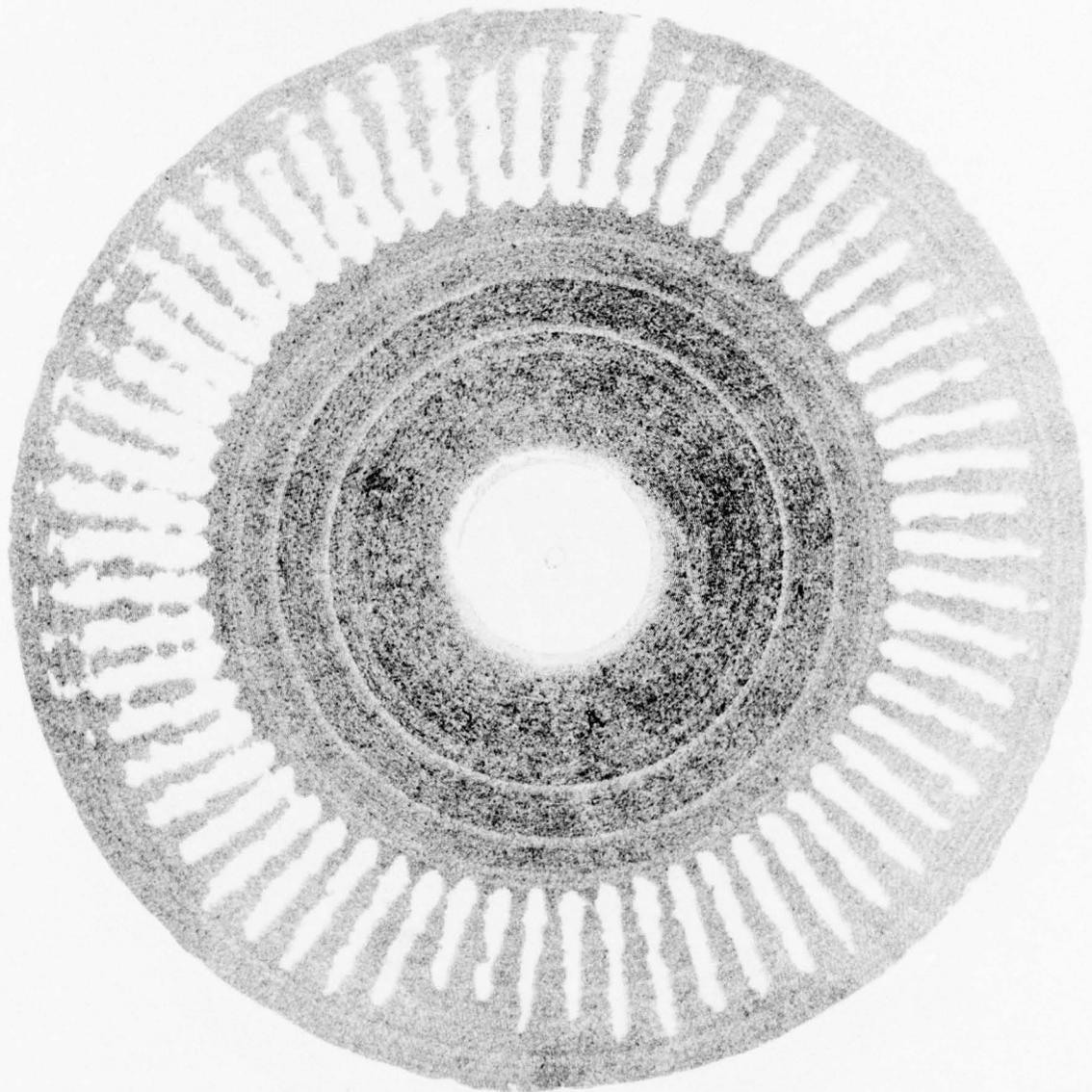
Figure 66. Ultrasonic Inspection Results of the Second Laminated Wheel Blank (Top View).
