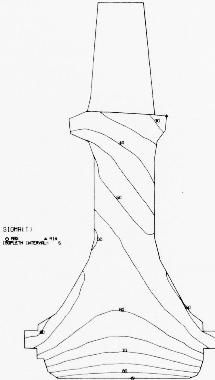
Figure 80. Laminated Turbine Wheel Tangential Stress Distribution (KSI) at a Speed of 29,692 RPM.
