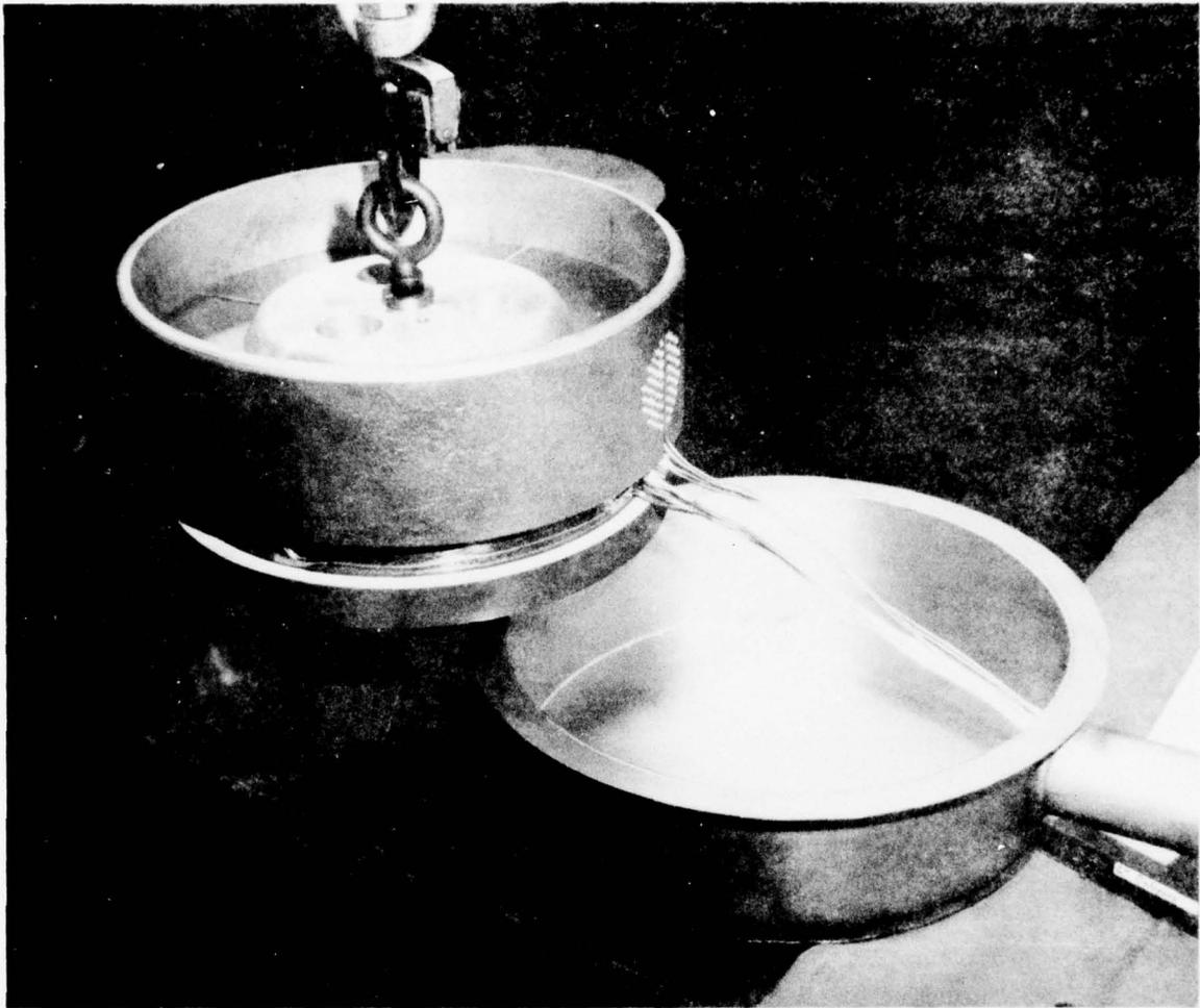
Figure 59. Unbonded Laminated Wheel Blank Being Placed Into the Retort.
