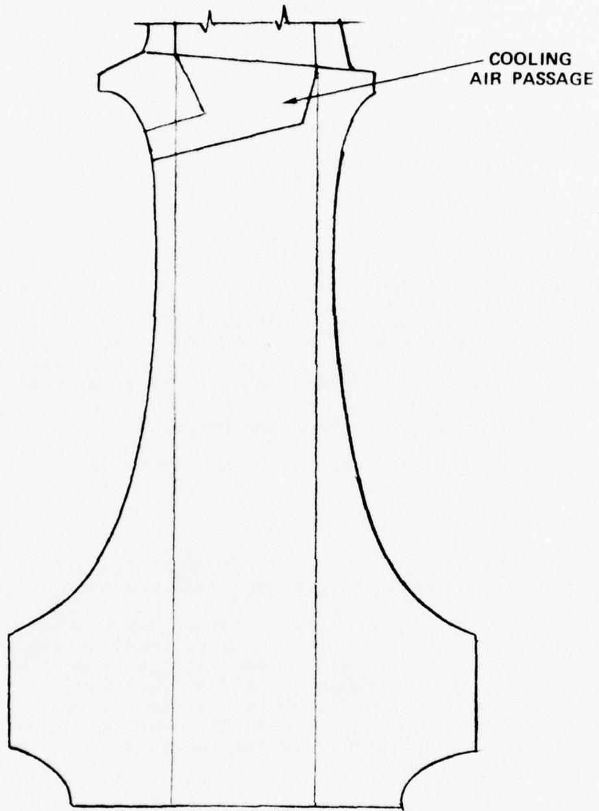
Figure 76. Preliminary Laminated Turbine Disk Geometry.
