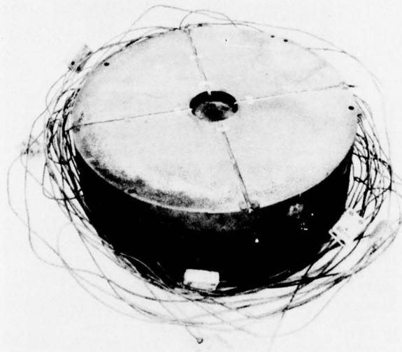
Figure 39. The Large Stack Laminated Wheel Blank, and the Waspaloy End Plates on the Bonding Fixture.
