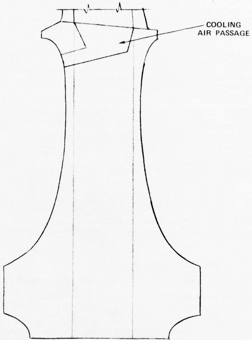
Figure 13. Preliminary Laminated Turbine Disk Geometry.
