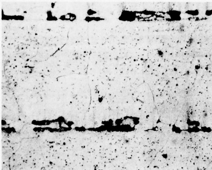
Figure 47. Optical Micrograph Showing Joint Microstructure in Stack 9 Following the Standard 2140°F Bond Cycle. The Double-Interface Condition is Clearly Evident. (Kallings Etch) (Mag.: 100X).
