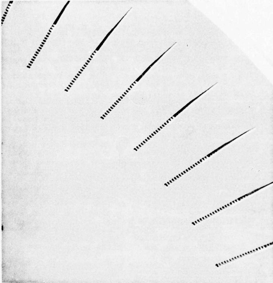
Figure 55. Laminate Trailing-Edge Orifices, and Pin Fins.
