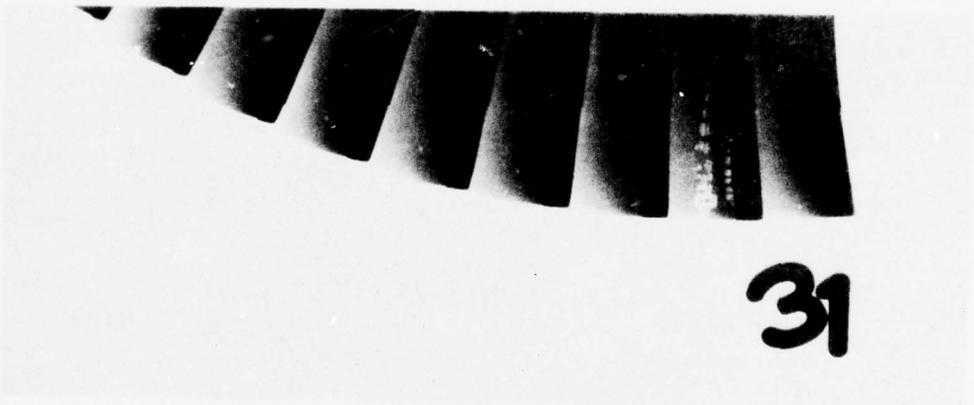
Figure 74. Radiographic Results from the Laminated Turbine Wheel.
