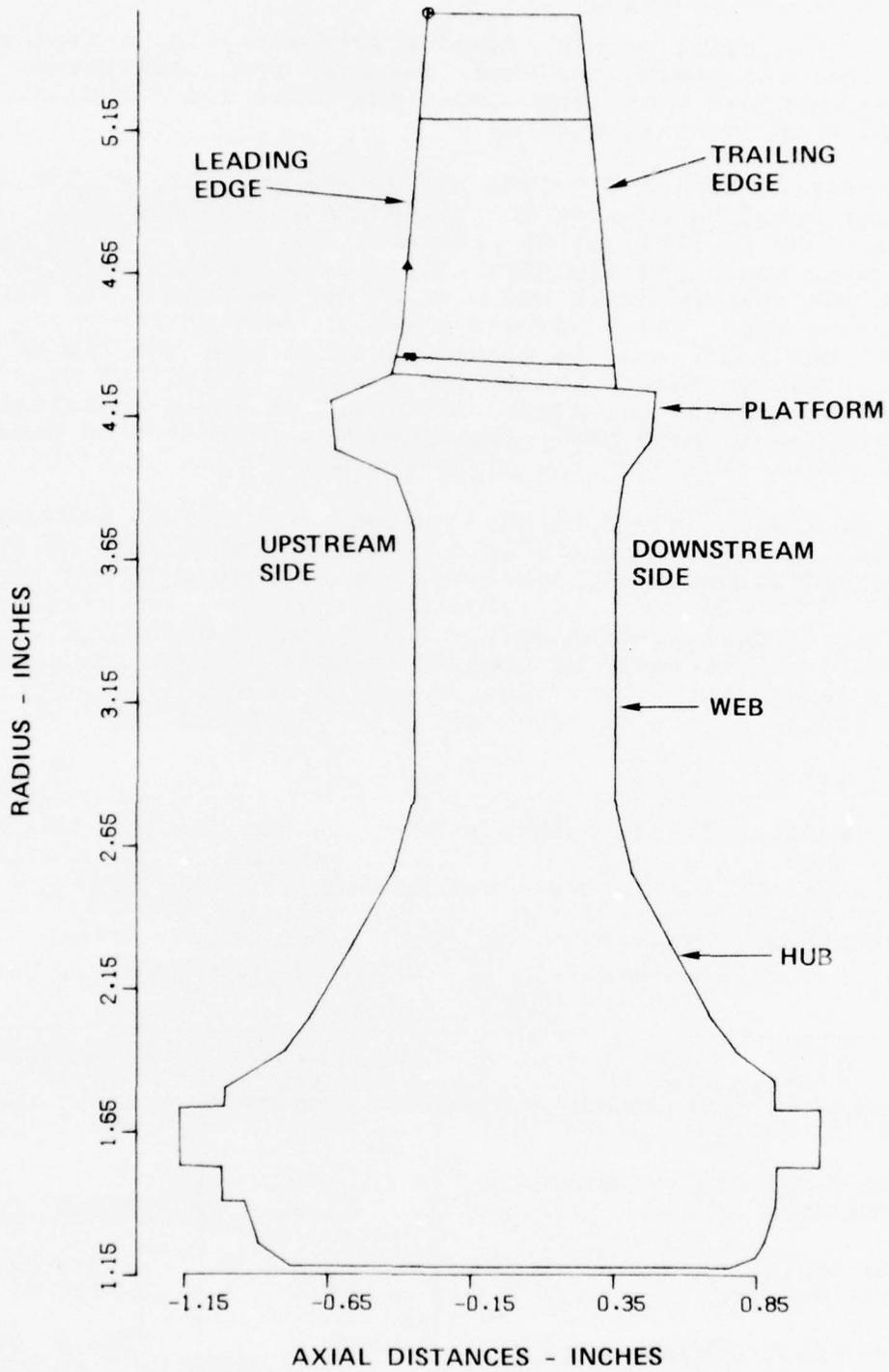
Figure 77. Laminated Turbine Disk Stress Analysis Geometry.
