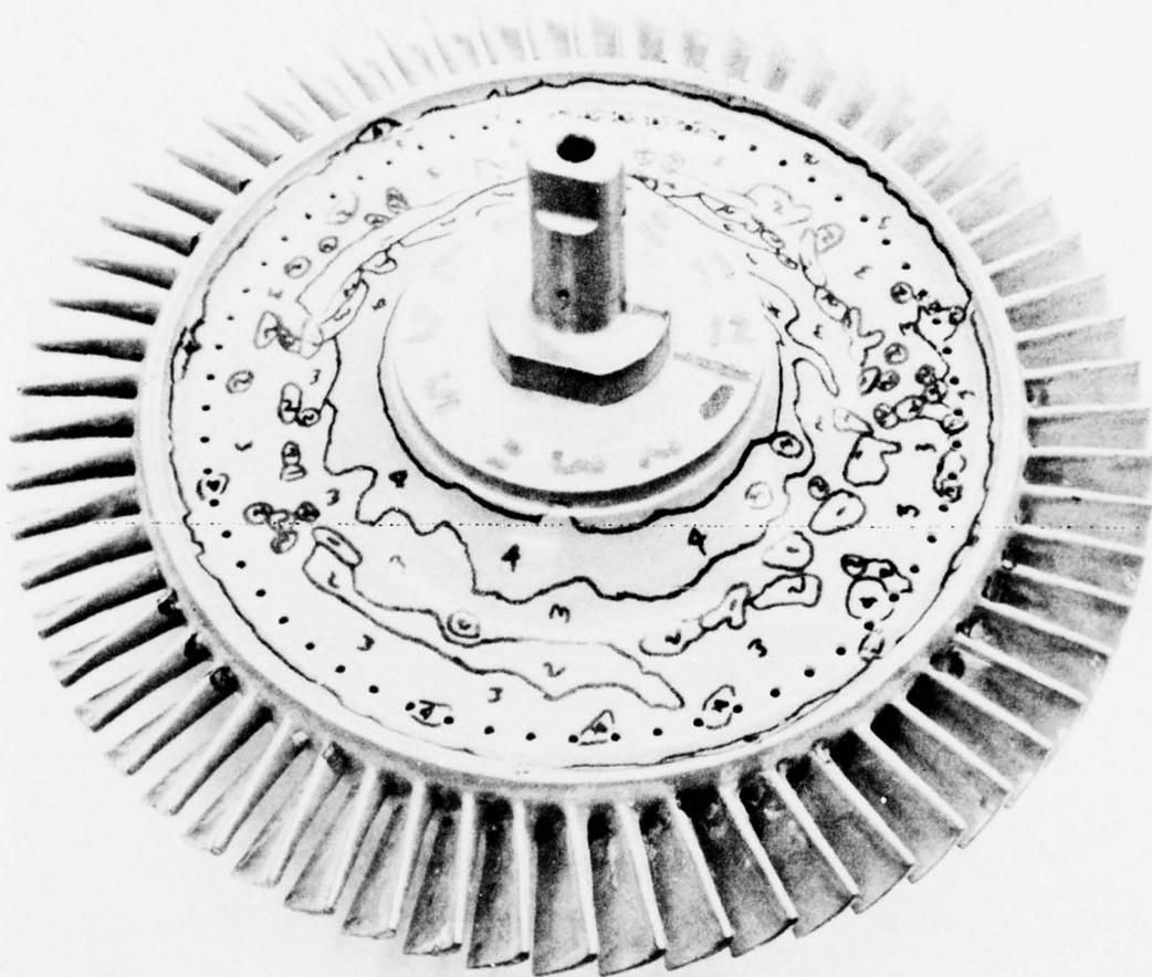
Figure 88. Laminated Turbine Wheel Leading-Edge Side
