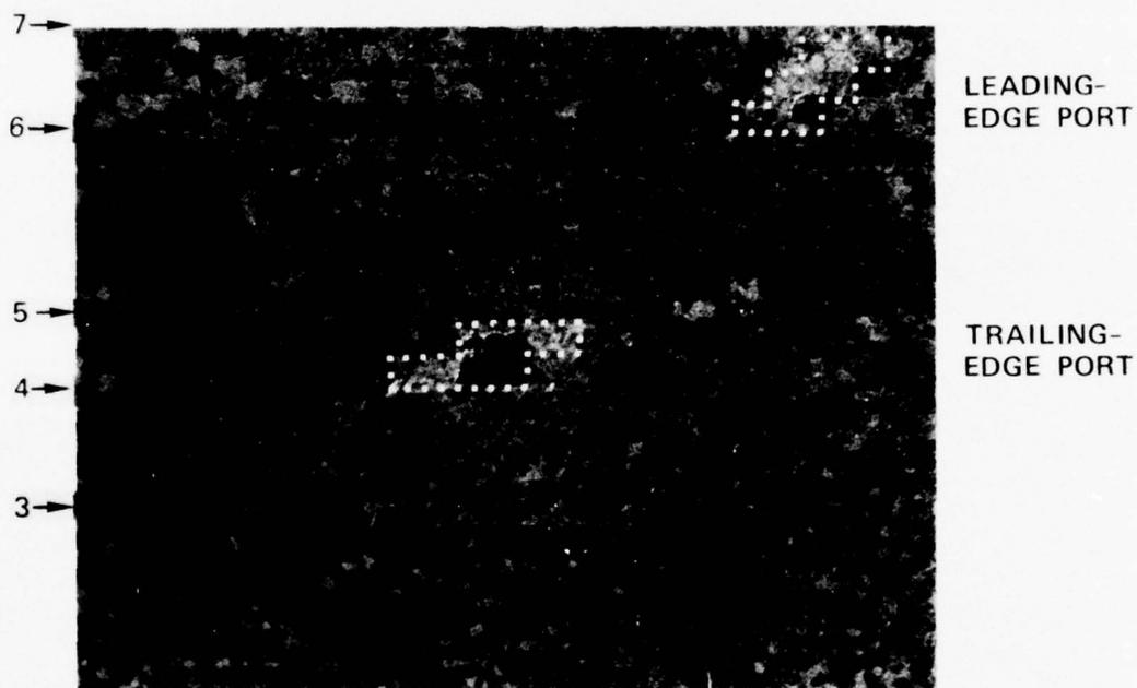
Figure 68. Metallographically Prepared Surface of the Second Wheel Blank Outside Diameter Showing the Extent of Flow of Bond Alloy Liquid into the Tip Passages. Dotted Lines Show the Approximate Passage True Size. Numbers at Left Edge Give Locations of Some of the Axial Points Used in the Dimensional Analysis. (Mag.: 10X)
