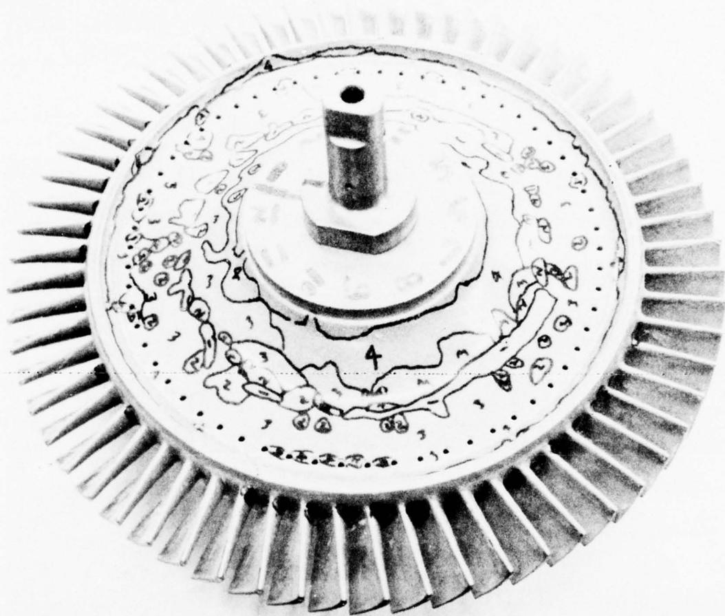
Figure 89. Laminated Turbine Wheel Leading-Edge Side After Stresscoat Testing (Wheel Rotated 180°).
