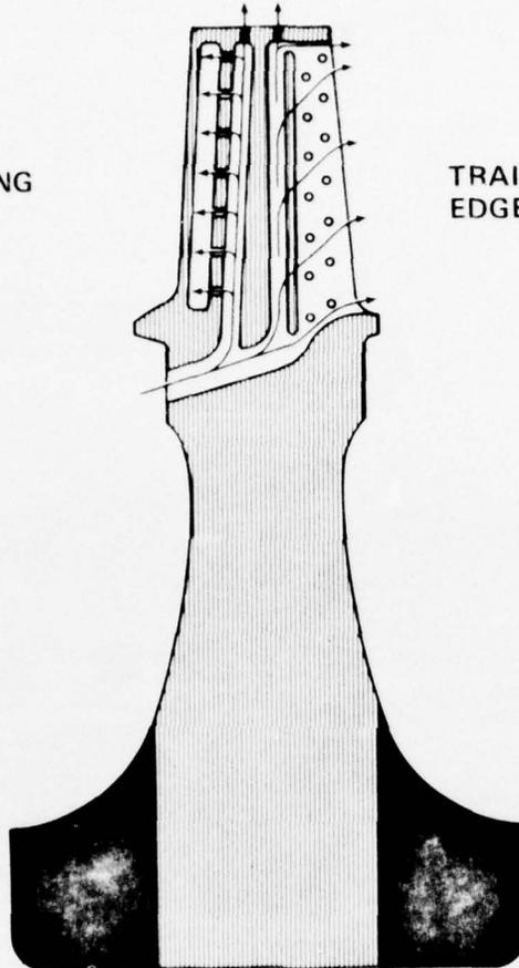
Figure 3. Cooling Concept Selected for Final Detail Design of the Laminated Axial Turbine Wheel.
