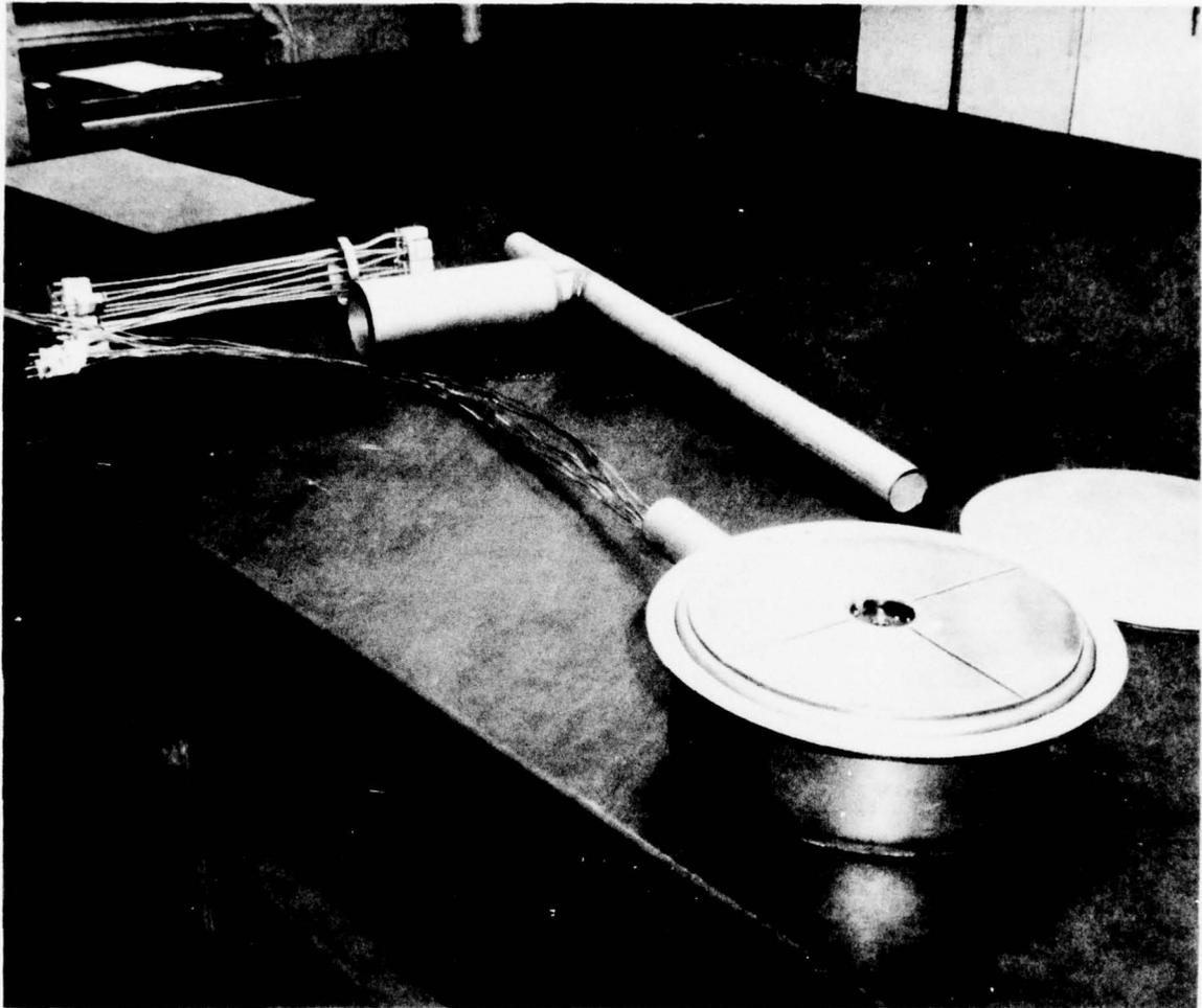
Figure 60. Thermocouple Leads and the Feedthrough for the Bonding Retort.
