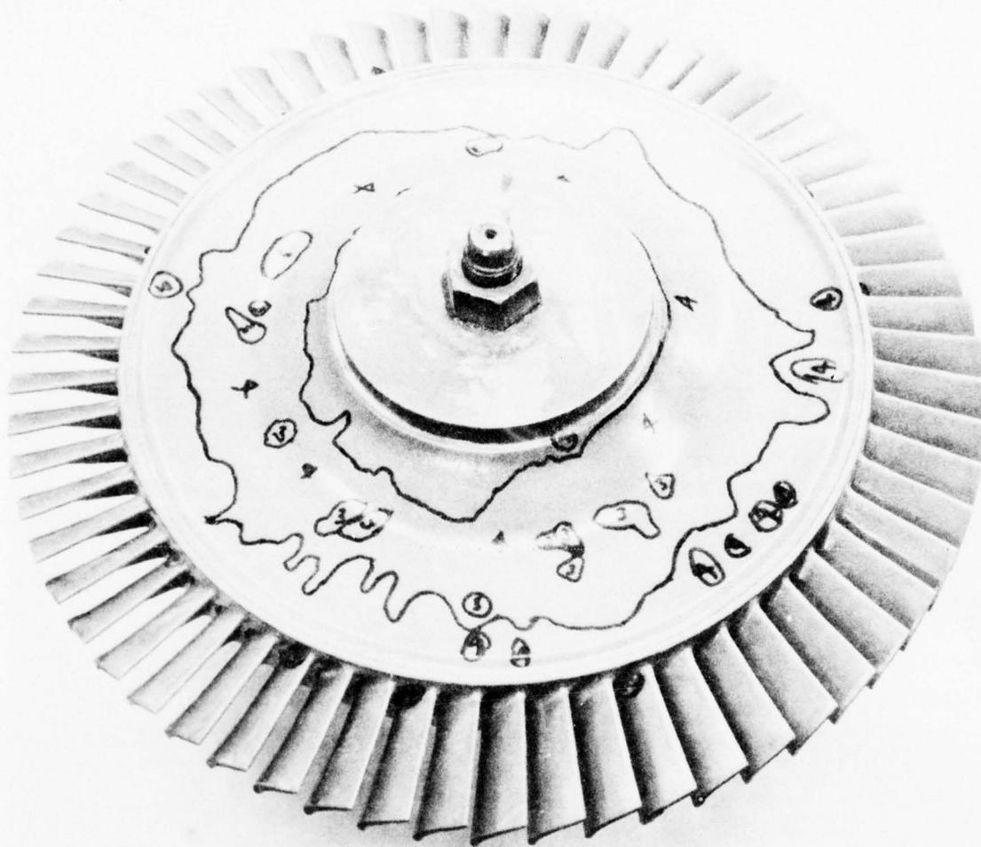
Figure 91. Laminated Turbine Wheel Trailing-Edge Side
