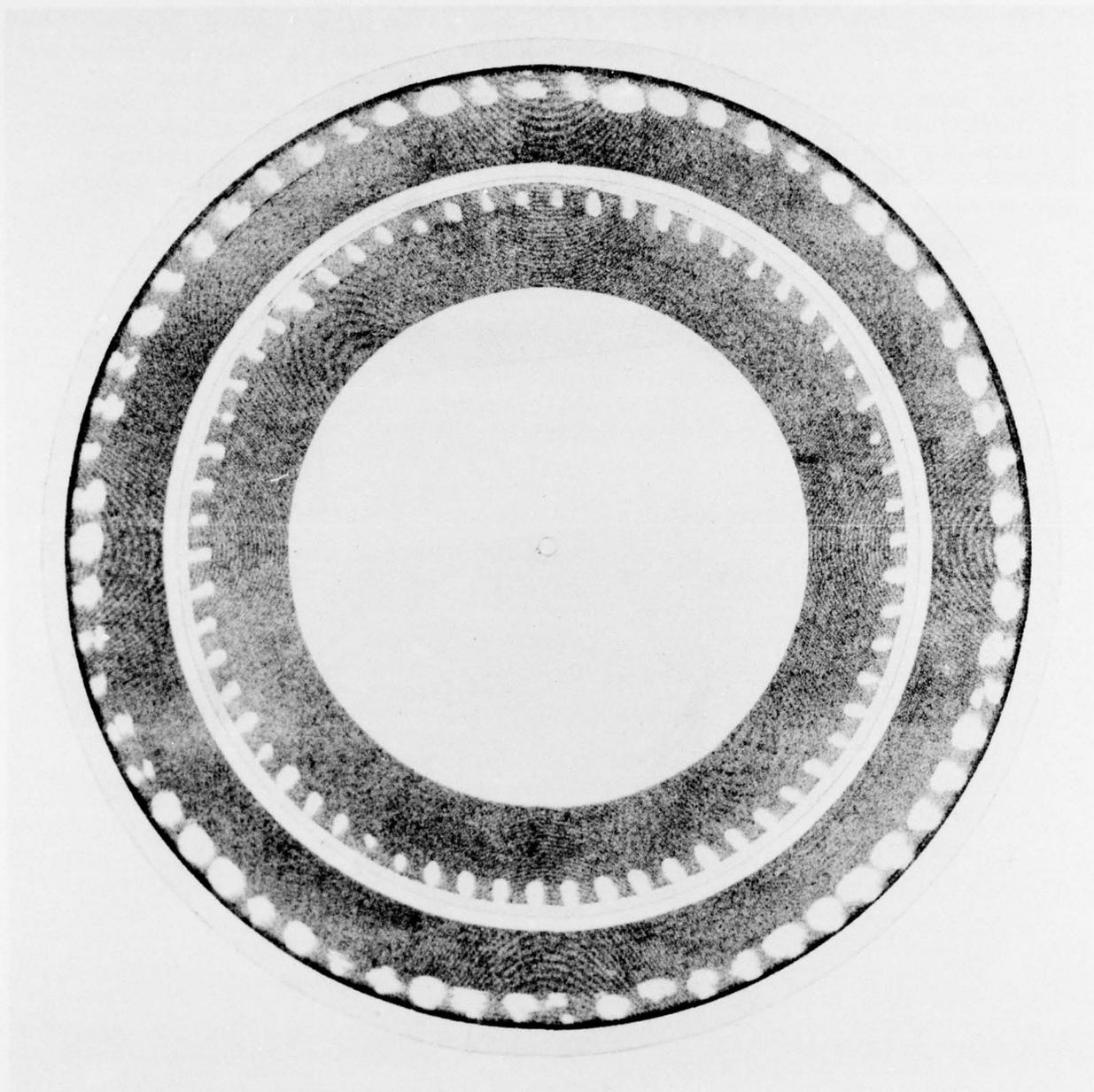
Figure 95. Ultrasonic C-Scan of the Laminated Turbine Wheel after Spin-Pit Testing.
