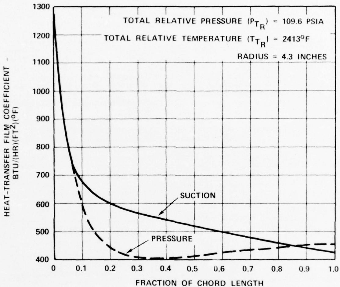
Figure 20. (a) High-Temperature Laminated Blade Turbulent Heat-Transfer Coefficients for Five Sections. (TIT Average = 2600°F, and  $P_{TIN}$  = 152.5 PSIA).
