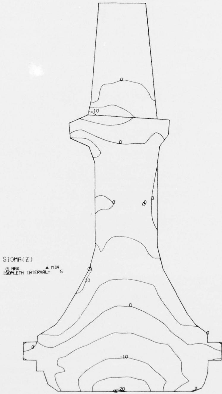
Figure 84. Laminated Turbine Wheel Axial Stress Distribution (KSI) at a Speed of 35,630 RPM.
