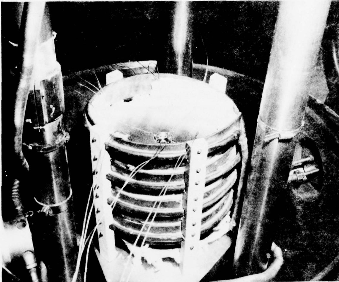
Figure 42. View of the Furnace Induction Coil with the Bonding Assembly Placed Inside, and the Placement of the Fiberfrax-Felt Insulation.
