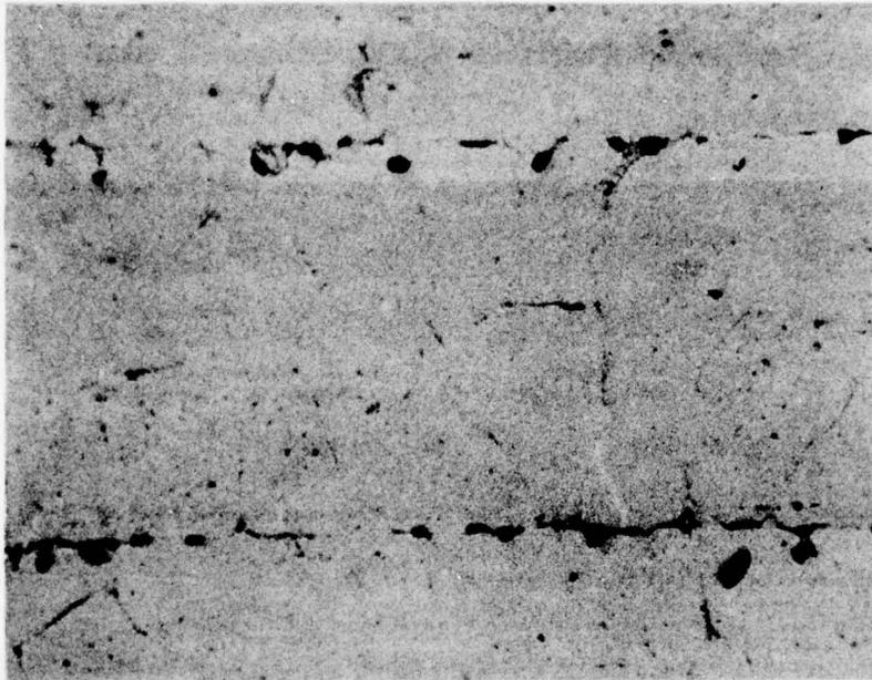
Figure 49. Photomicrograph Showing the Microstructure Near to the Bottom Edge of Stack 10. Note the Eutectic Film at the Lamination Interfaces and Along the Grain Boundaries. The Bonds are Quite Porous. (Unetched) (Mag.: 100X)
