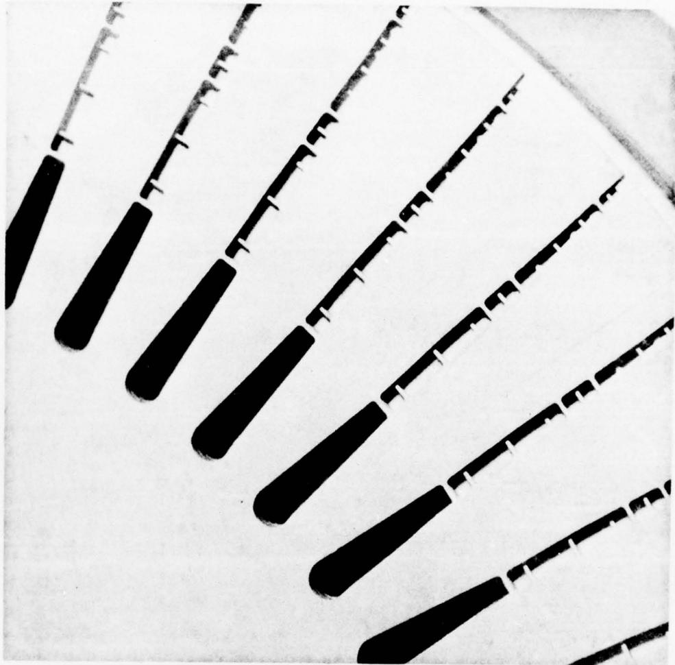
Figure 5. Completed Final Wheel Blank Laminate Showing Center Section Convection Cooling Passages.
