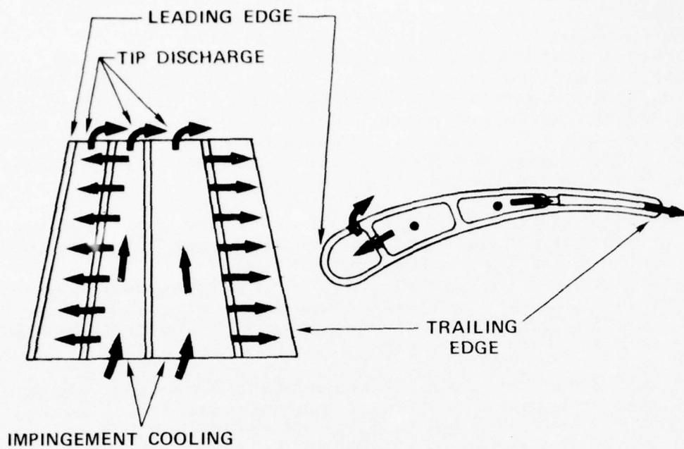
Figure 12. Impingement-Cooled Leading-Edge, Tip, and Trailing-Edge Discharge Cooling Scheme for the TFE731-3 Laminated Turbine Wheel.
