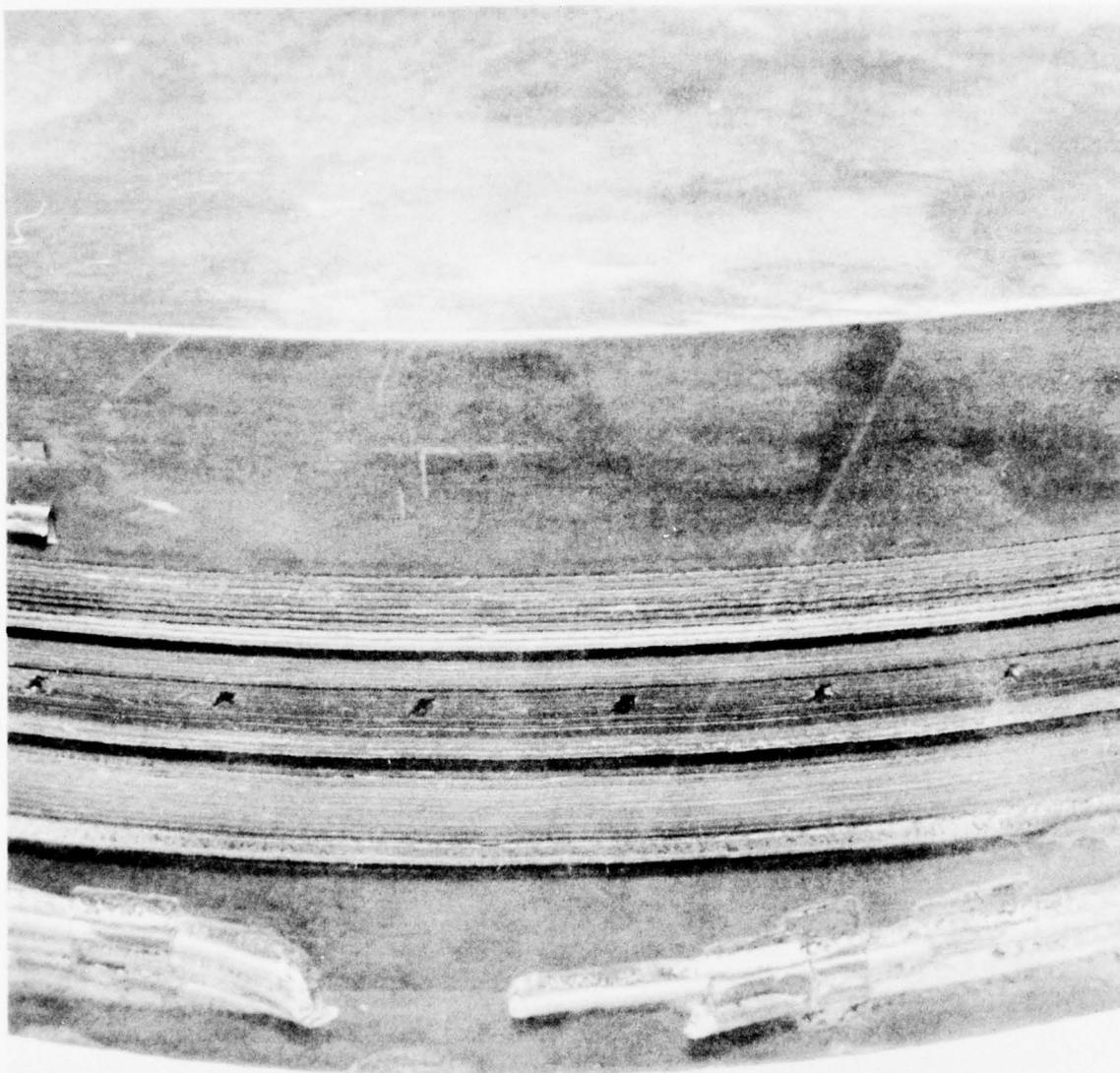
Figure 65. View of the As-Bonded Second Wheel Blank. Flow of the Bond Alloy is Visible as Fillets on Thermocouples and on the Lower Trailing-Edge Dimension Land. Note Erosion of the Land at the Far Right of the Photograph.
