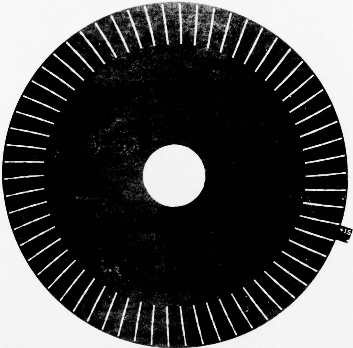
Figure 4. Completed Final Wheel Blank Laminate Showing Cooling Passages
