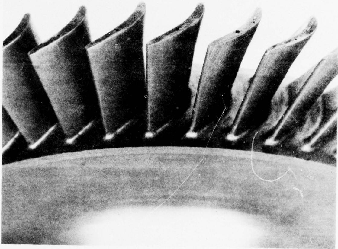
Figure 73. Close-up of the Blade Tips on the Finish-Machined Laminated Turbine Wheel.
