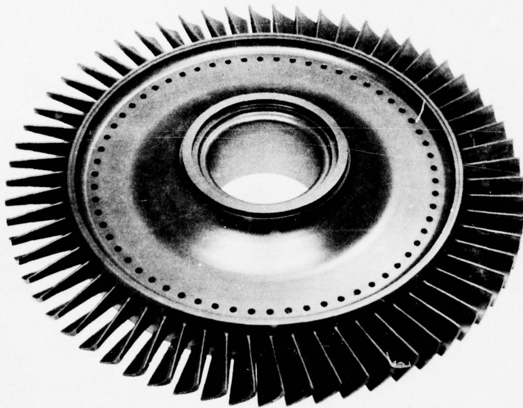
Figure 72. Fully-Machined Laminated Turbine Wheel.
