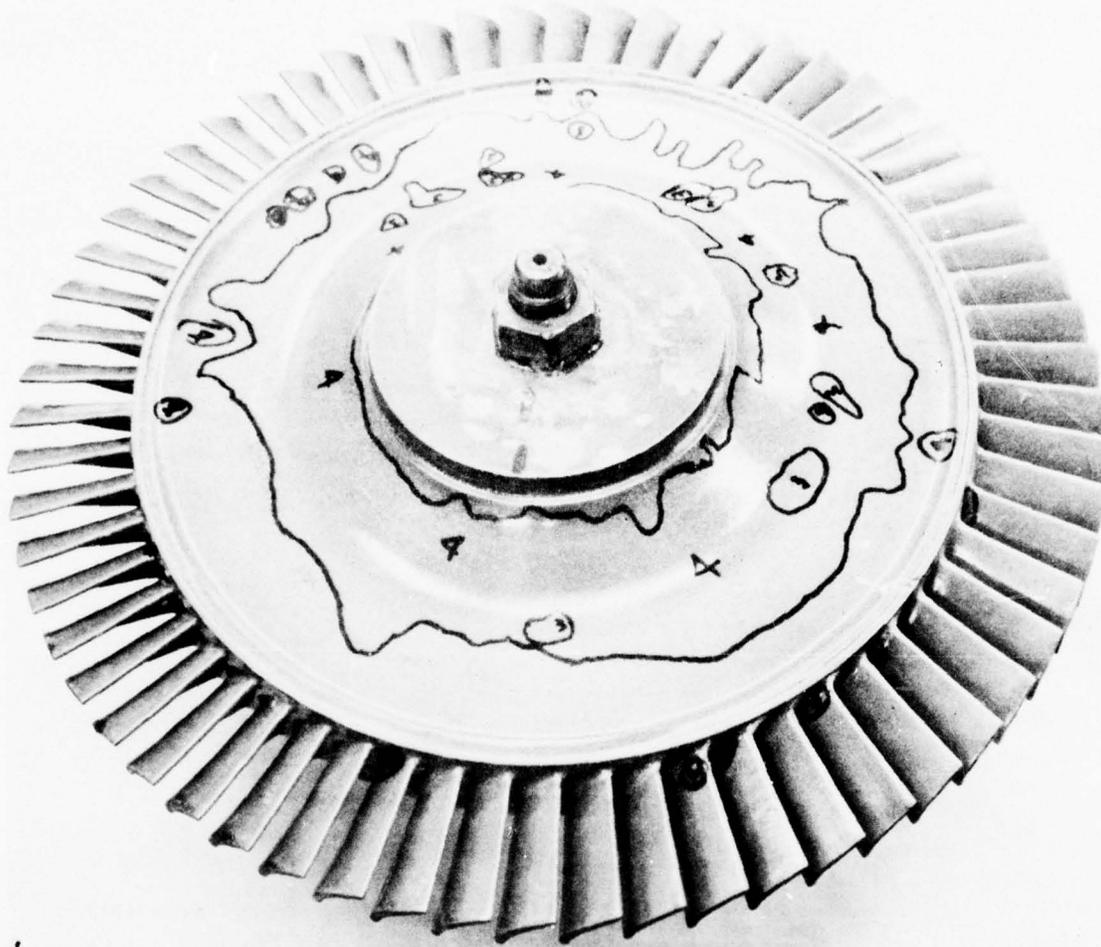
Figure 90. Laminated Turbine Wheel Trailing-Edge Side
