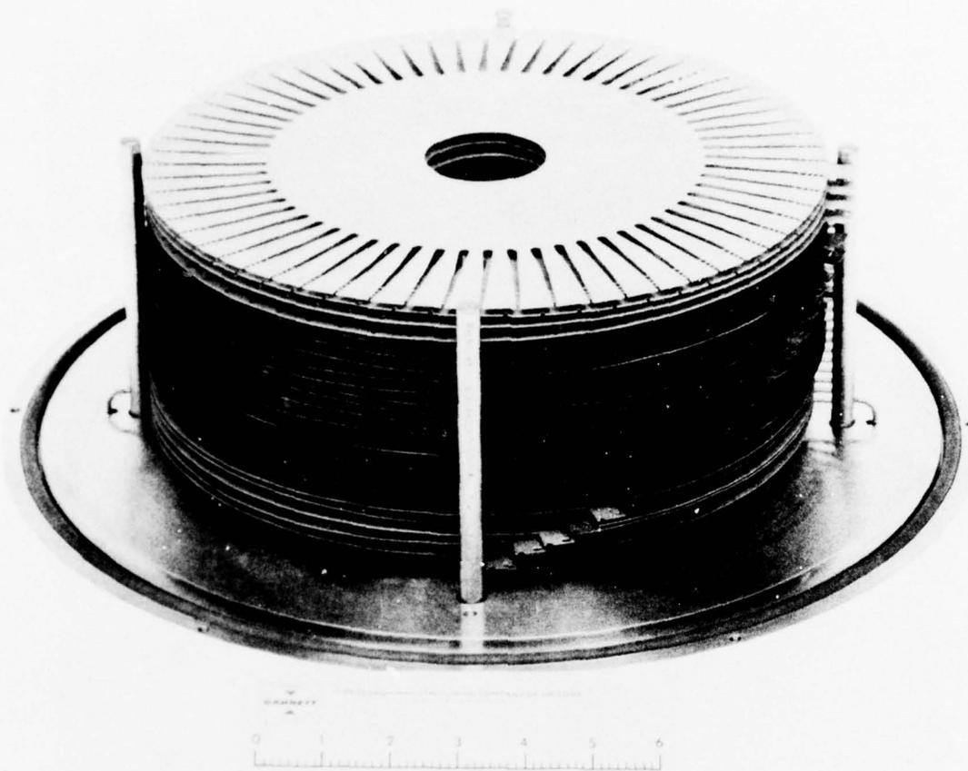
Figure 52. Laminates Racked on the Outgass Tooling.
