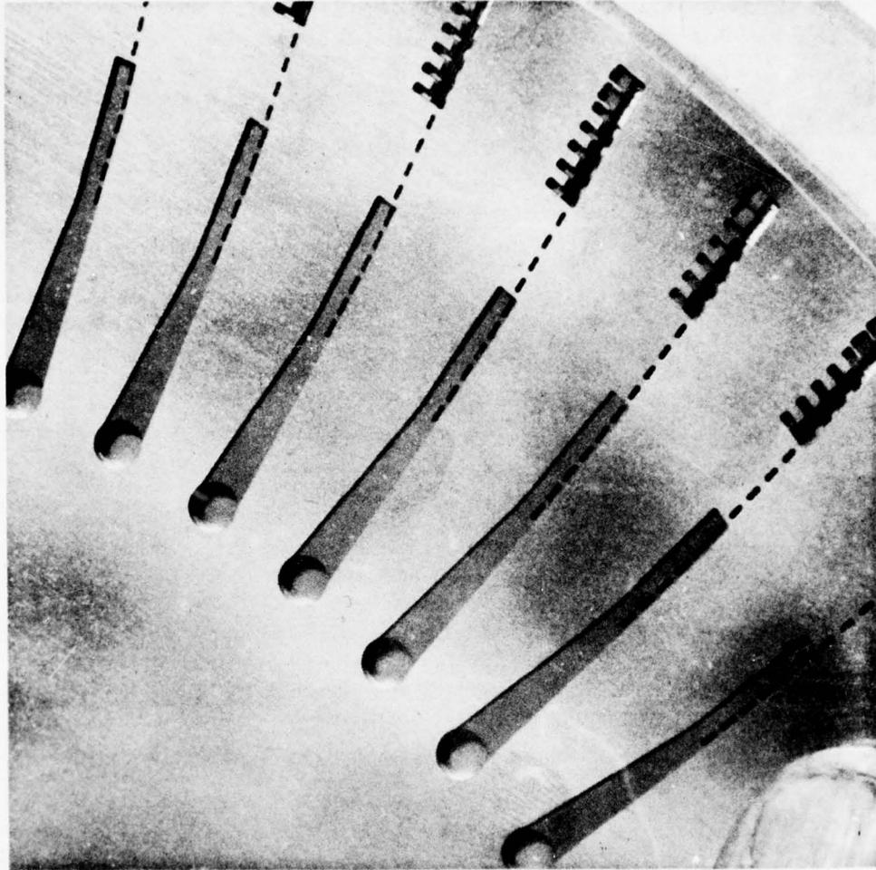
Figure 54. Laminate Leading-Edge Area Impingement Plus Film Cooling.
