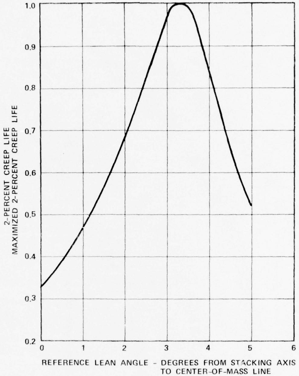
Figure 23. Laminated Turbine Blade Lean Angle Creep-Life Optimization.
