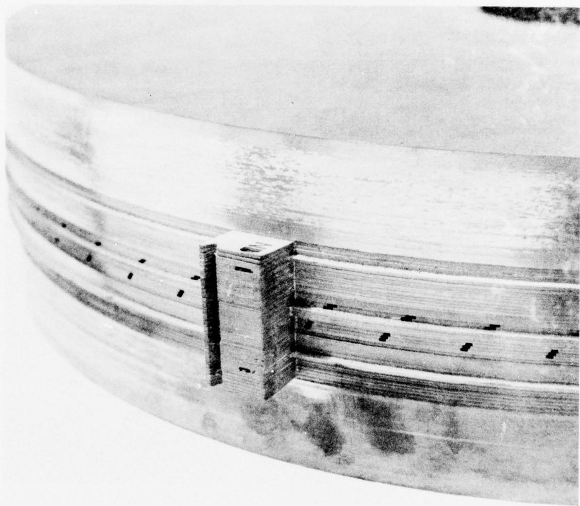
Figure 63. Completed Laminated Wheel Stack at the Blank Outer Diameter Tab Area.
