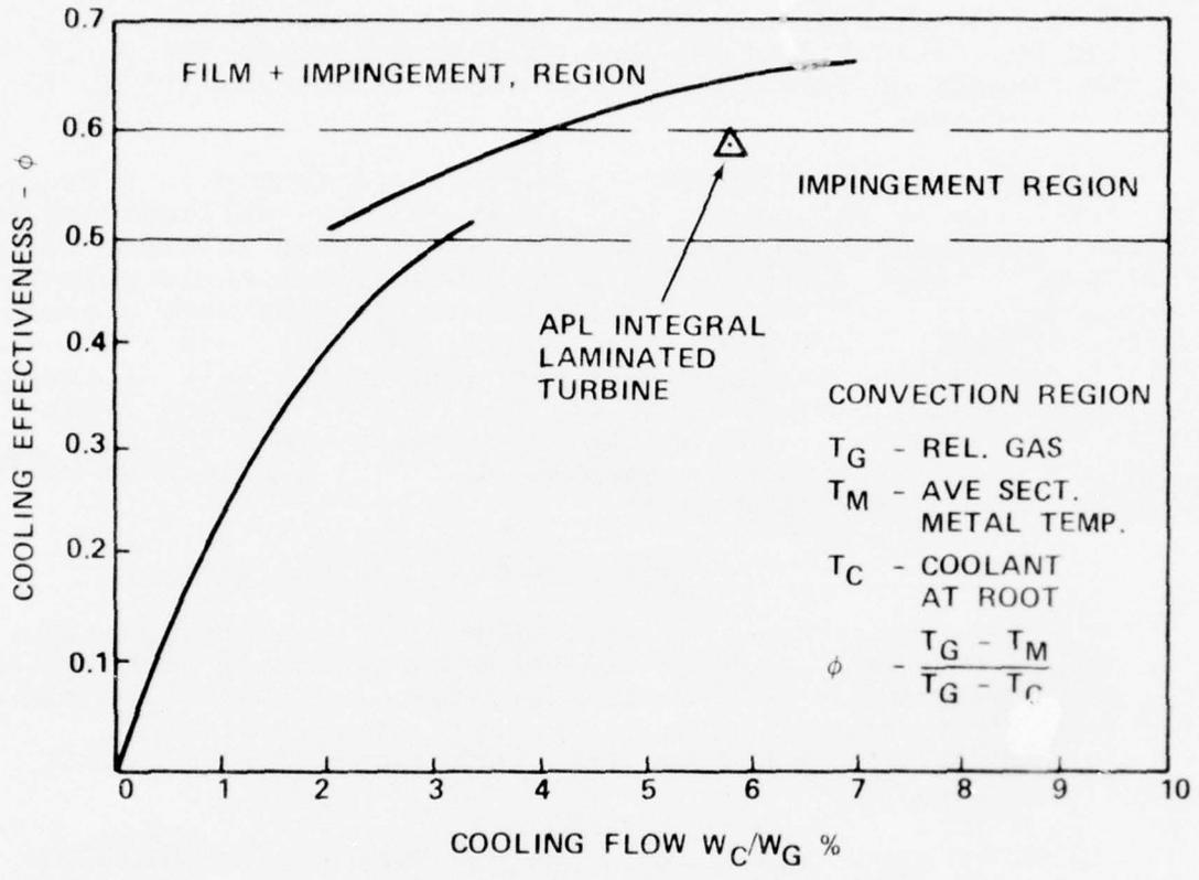
Figure 22. Laminated Turbine Blade Airfoil Cooling Effectiveness.
