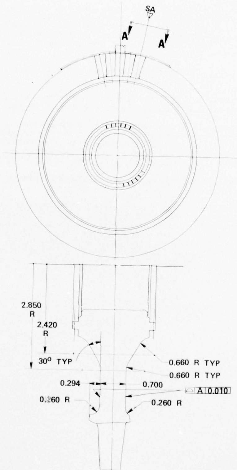
Figure 34. (a) Final Laminated Turbine Rotor Detail Design.
