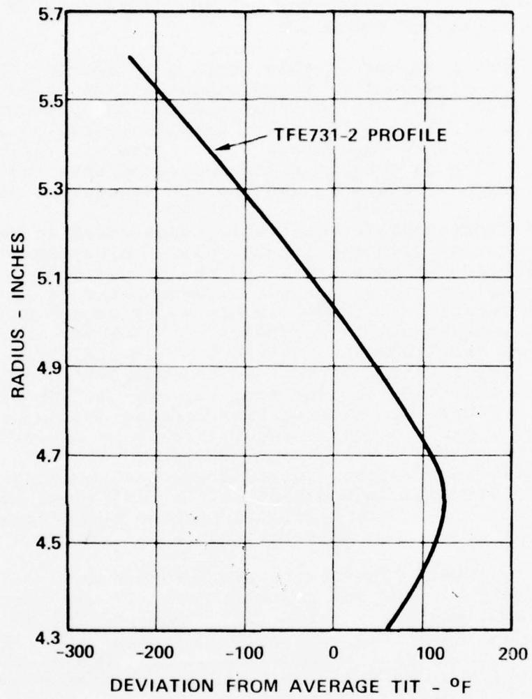
Figure 19. High-Temperature Laminated Turbine Blade Inlet Temperature Profile.
