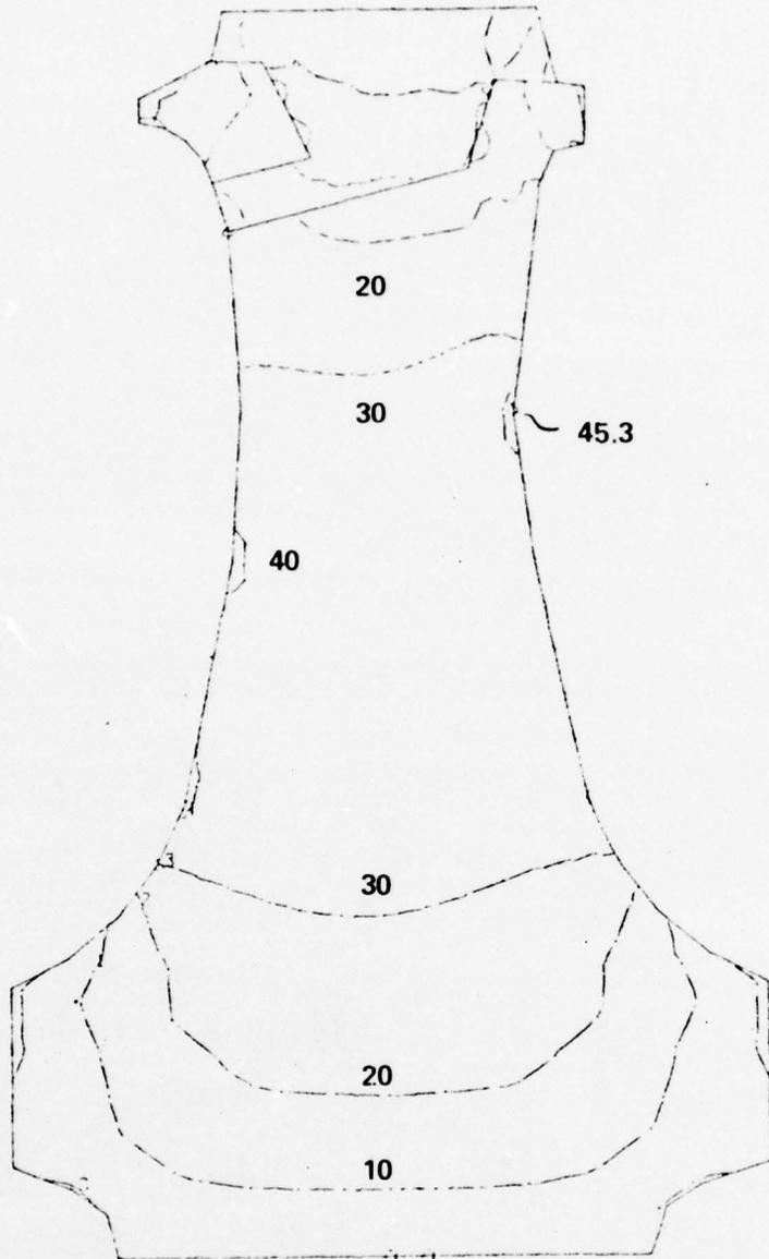
Figure 15. Laminated Turbine Disk Radial Stress Distribution (KSI) Due to Centrifugal Loading Only (29,692 RPM).
