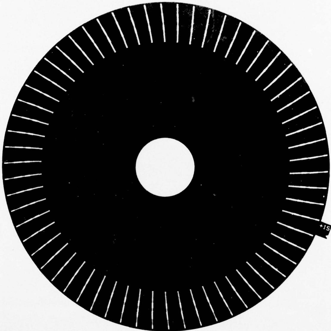
Figure 50. Completed Final Wheel Blank Laminate Showing Cooling Passages.
