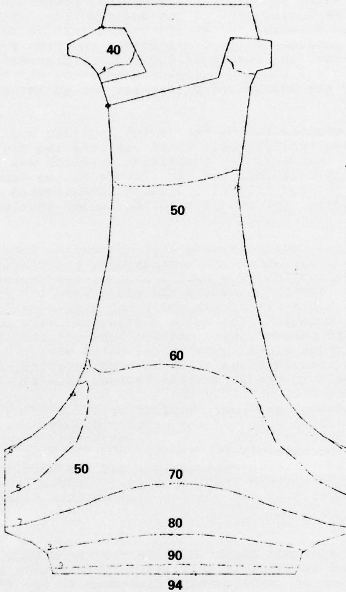
Figure 16. Laminated Turbine Disk Tangential Stress Distribution (KSI) Due to Centrifugal Loading Only (29,692 RPM).
