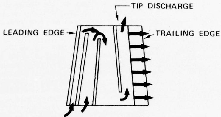
Figure 11. Three-Pass, Two-Passage, Tip and Trailing-Edge Discharge Cooling Scheme for the TFE731-3 Laminated Turbine Wheel.
