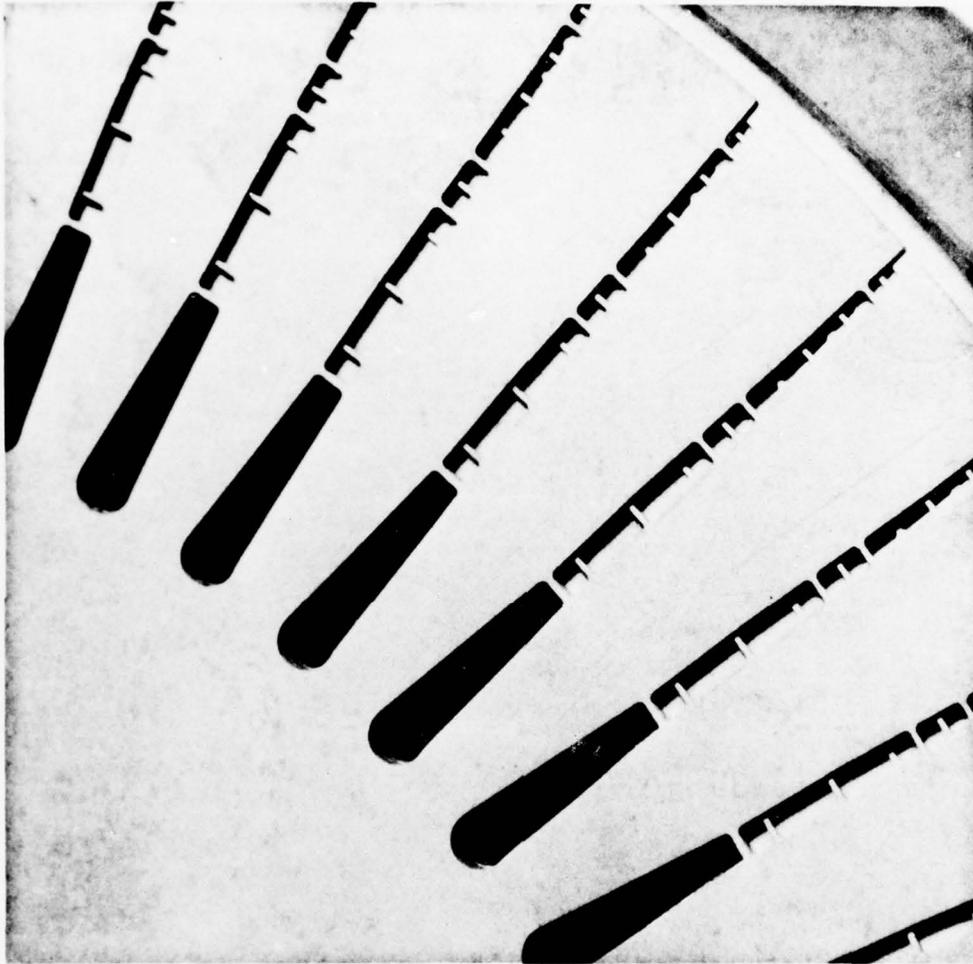
Figure 51. Completed Final Wheel Blank Laminate
