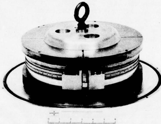
Figure 38. Large Stack Laminates, End Plates, and the Bonding Fixture.
