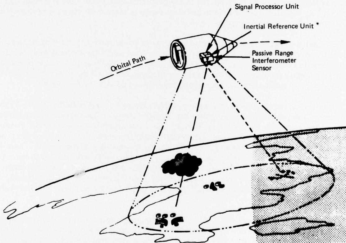
\*This function can be provided by PRAIS in orbits where at least two landmarks are continuously visible or on spacecraft with independent local vertical-oriented attitude control systems.
