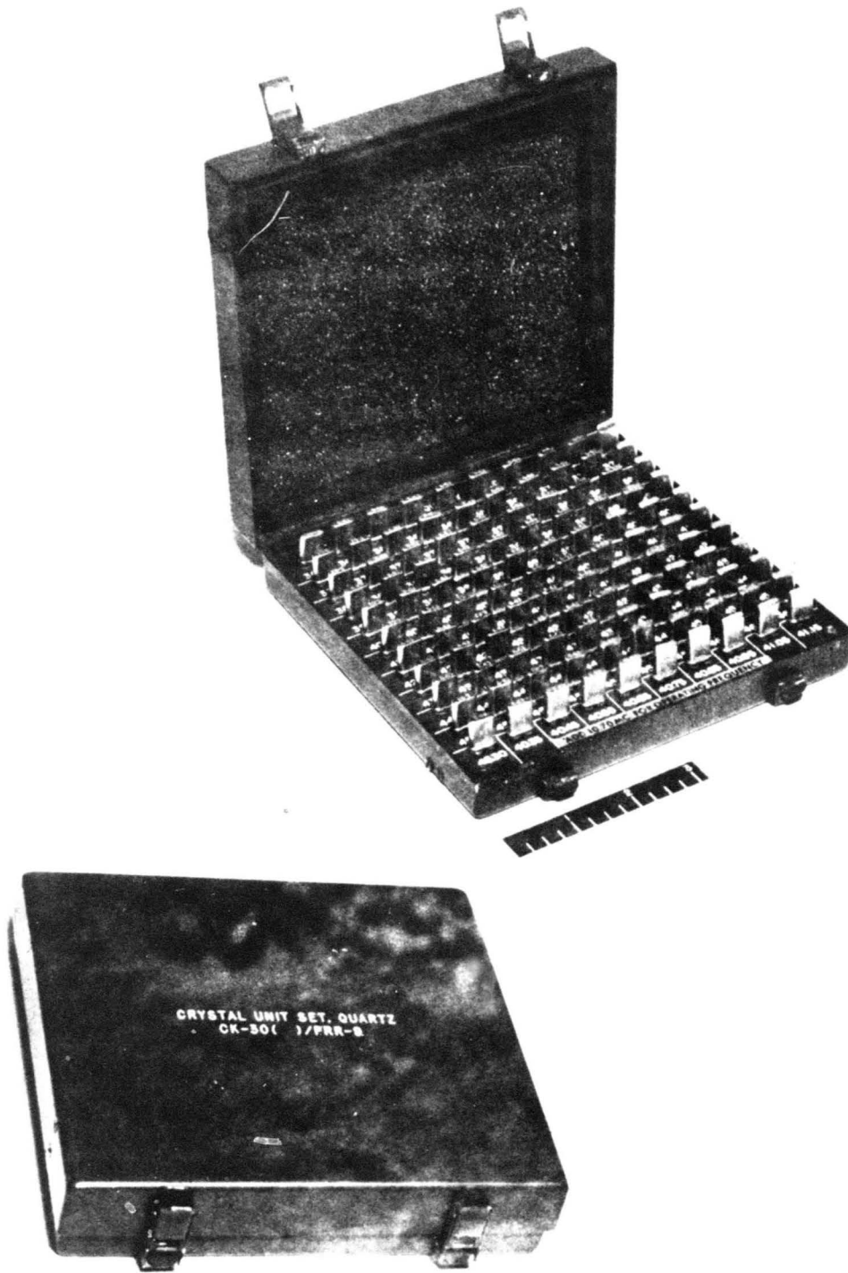
Figure 36. Crystal kit for final models of Radio Transmitter AN/PRT-4 and Radio Receiver AN/PRR-9.
