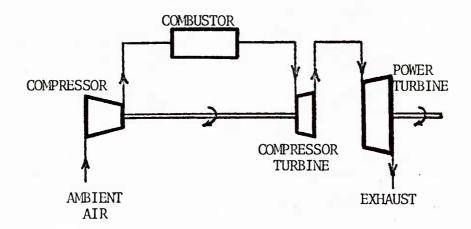
The Gatric was rated for 2500 hp and replaced the center of three gasoline-powered engines, all with separate power trains and propellor shafts. The engine was designed for only 300-hrs operating life, its overall pressure ratio was 3.5, the compressor turbine entry temperature (TET) at maximum power was 750°C, and it had a specific weight of 2.8 lb/shp.
