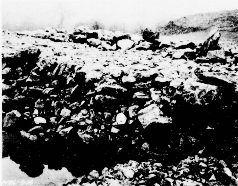
a. Section of rock test fill 1 (6- to 18-in. weathered rock)
