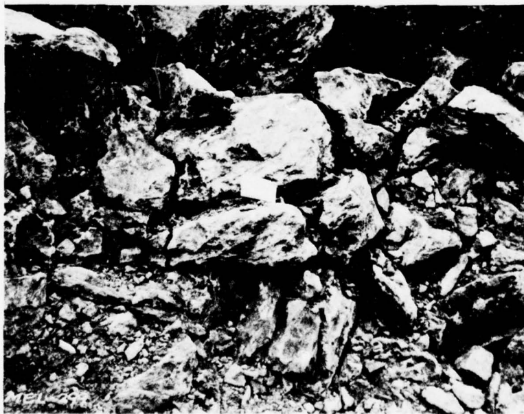
b. Closeup view of rock test fill 4 (6- to 18-in. unweathered rock)
