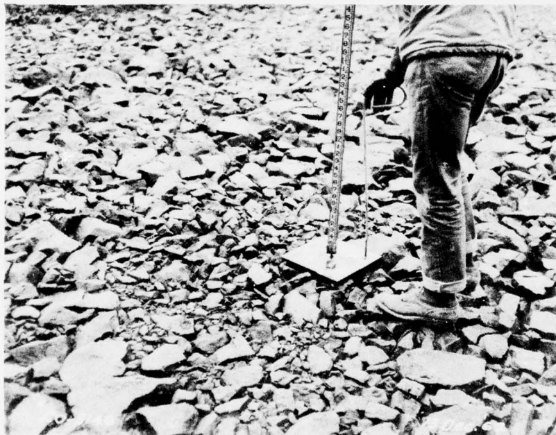
Fig. 27. Apparatus for taking level readings, Cougar test fill
