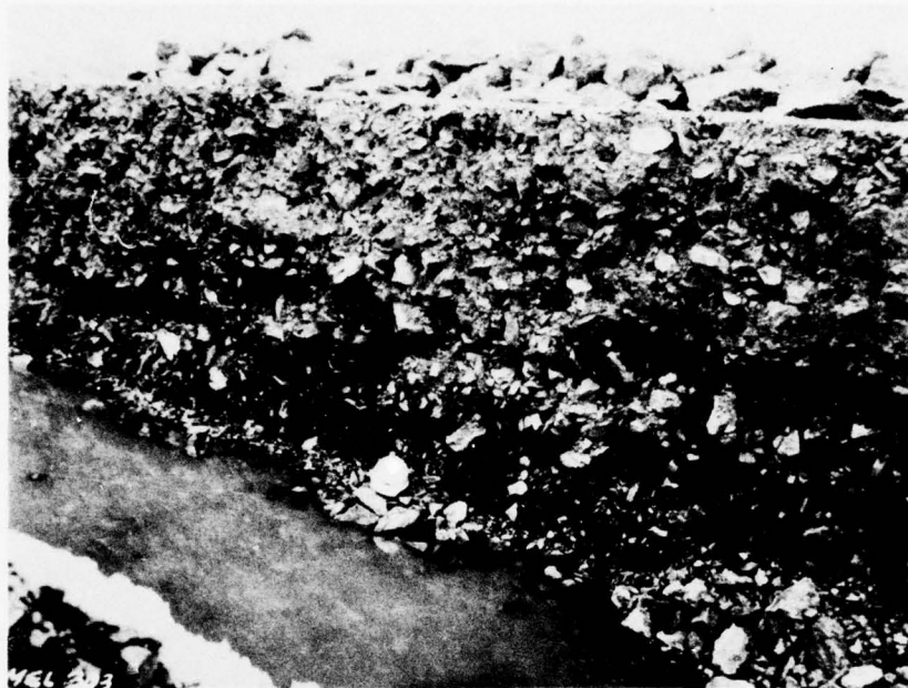
a. Section of rock test fill 3 (minus 6-in. unweathered rock transition)
