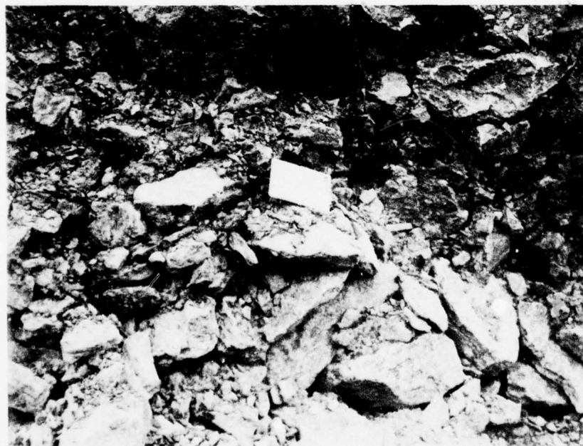
b. Closeup view of rock test fill 3 (minus 6-in. unweathered rock transition)
