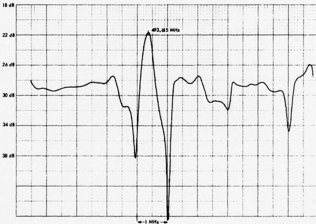
Figure 2-19. SAW Delay Line Insertion Loss S/N 206
