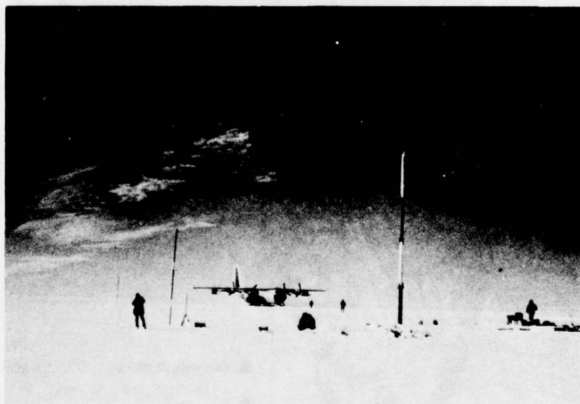
Figure 3. Geoeiver positioning at Crete. EGIG pole T43 is between man at left and Geoeiver antenna.
