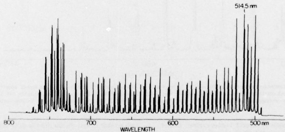
FIG. 4. Photoluminescence spectrum of  $\text{Bi}_2$  excited by the 514.5 nm  $\text{Ar}^+$  laser line obtained with 0.02 nm resolution. This spectrum extends over the whole Franck-Condon distribution including both maxima; it is not corrected for instrumental response.
