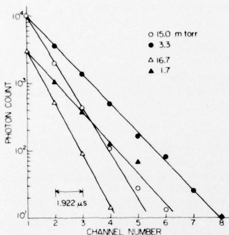
Fig. 2. Observed decay of fluorescence intensity. Circles represent single band detection (1 nm) and triangles represent single rotational line detection (0.015 nm). The delay time per channel is 1.922  $\mu$ s.
