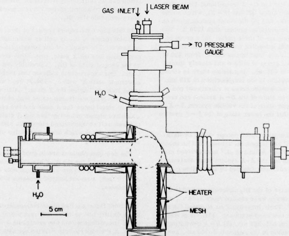
FIG. 1. Heat-pipe oven used for production of  $\text{Bi}_2$ .
