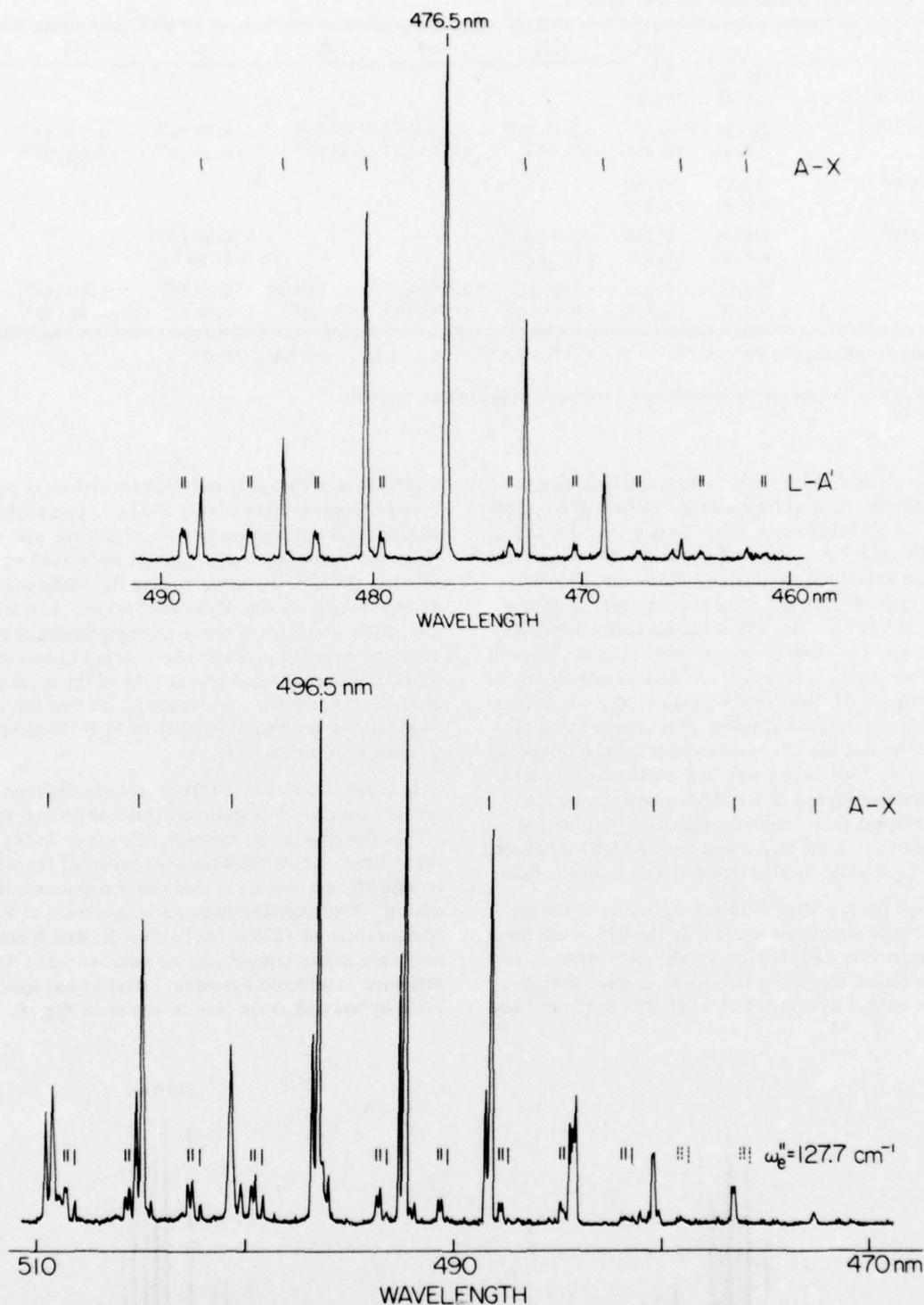
FIG. 5. Photoluminescence spectra of  $\text{Bi}_2$  excited by the 496.5 nm (lower spectrum) and the 476.5 nm (upper spectrum)  $\text{Ar}^+$  laser lines. Both excitation lines excite vibrational-rotational transitions of the  $A-X$  system. In addition the 496.5 nm laser lines excite two overlapping doublet photoluminescence series while the 476.5 nm laser line excites one doublet series.
