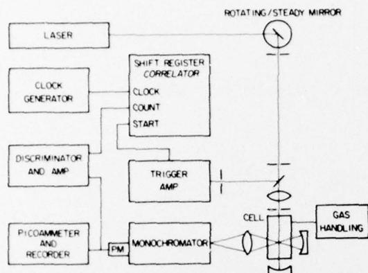
Fig. 1. Experimental arrangement.
