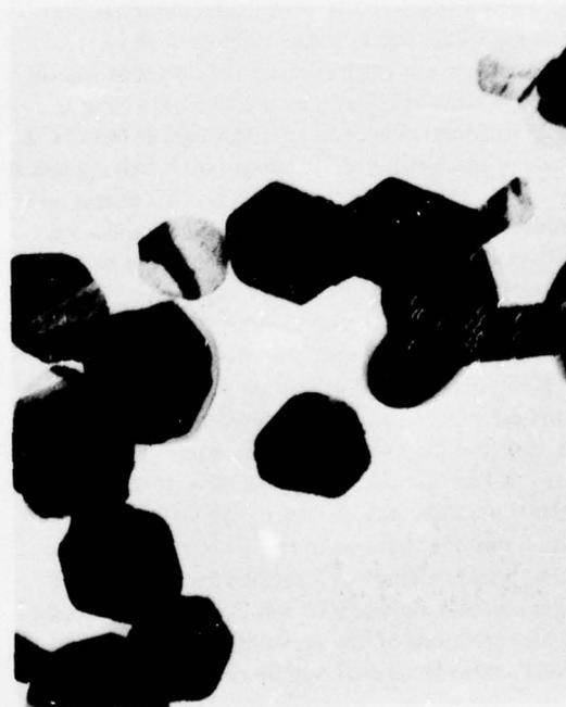
Fig. 4. An example of hexagonal platelets collected from the chamber walls. These hexagons are approximately 130 nm on a side (40,000  $\times$  plus photographic enlargement).
