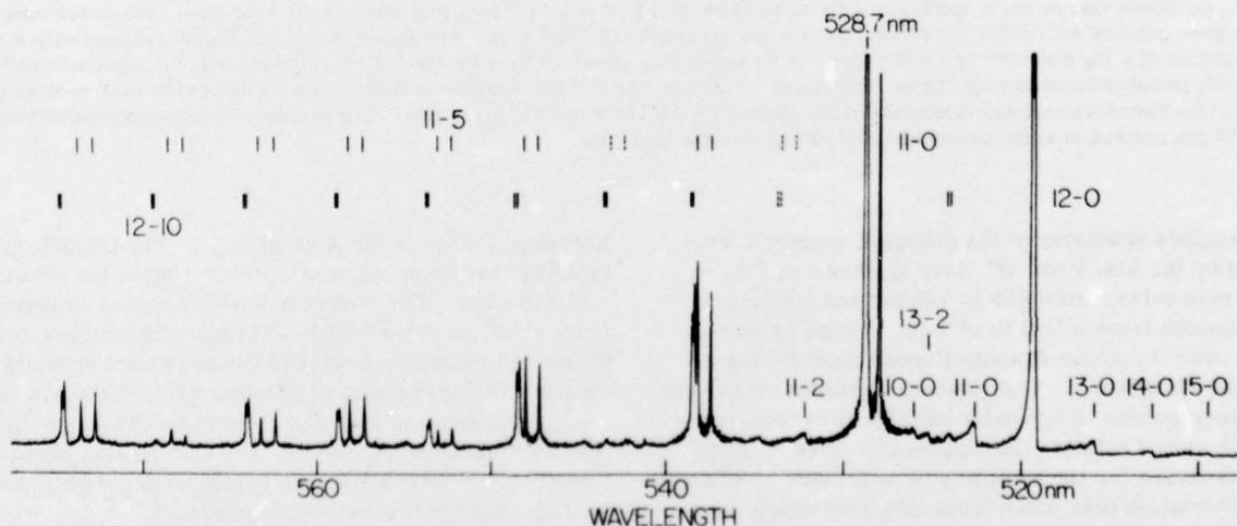
FIG. 2. Photoluminescence spectrum of Bi<sub>2</sub> excited by the 528.7 nm Ar<sup>+</sup> laser line. The spectrum is taken with 0.06 nm resolution in the flow system at an Ar-carrier gas pressure of 1 torr and is not corrected for instrumental response. The two observed doublet series as well as some rotational and vibrational relaxation can be seen.
