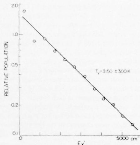
Fig. 3. Vibrational population distribution in the  $A^2\Pi_{1/2}$  state of  $BiO$  produced from the reaction of bismuth and  $N_2O$ . Vibrational populations ( $v'$ ) were obtained by averaging over the observed  $v''$  progression. Franck-Condon factors were calculated by the RKR method using molecular constants obtained by Barrow et al. [4]. The total pressure was 7 torr and the temperature reading of the thermocouple outside the oven was 1350 K.
