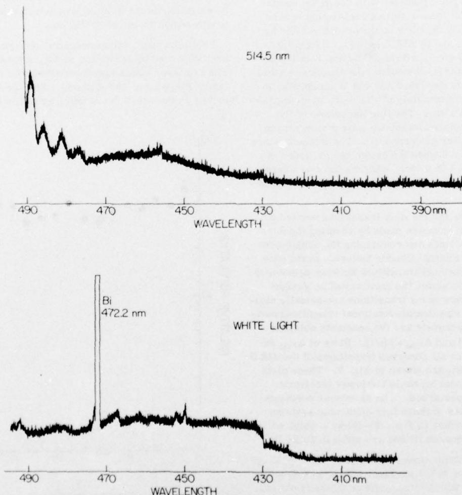
FIG. 11. Continuous spectra are obtained with white light excitation (lower spectrum) and with 514.5 nm Ar<sup>+</sup> laser excitation (upper spectrum) of Bi<sub>2</sub> at a pressure of 0.1 torr and temperature of 1090 K in the heat pipe.
