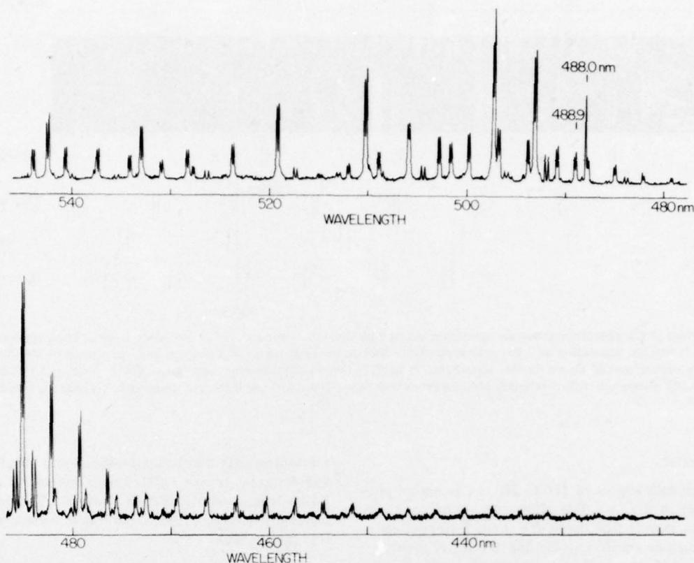
FIG. 6. Photoluminescence spectrum of Bi<sub>2</sub> in the heat pipe excited by 488.0 nm and 488.9 nm Ar<sup>+</sup> laser lines. The 488.0 nm laser line excites four different electronic transitions, one of them consists of a high number of anti-Stokes lines extending to shorter wavelengths.
