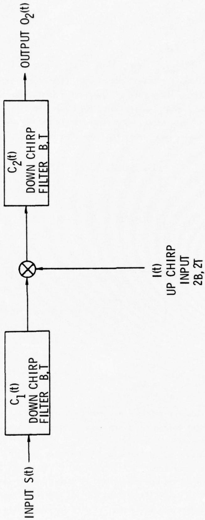
Figure 11 Chirp Transform Dual
