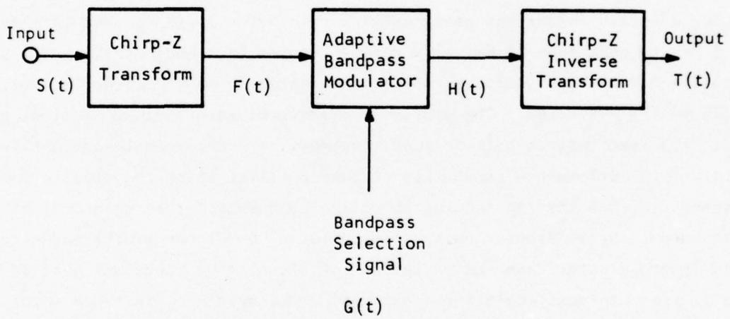
Figure 2 Block Diagram of the Acoustic Adaptive Transversal Filter Using the Transform Adaptable Processing System (TAPS)
