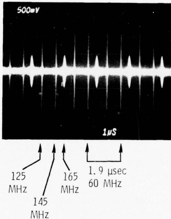
Figure 10 Transform Continuous Operation of the Prototype for the Three-Tone Input Used for Figure 9(a)
