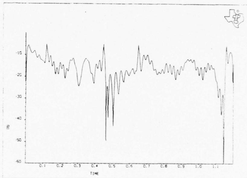
Figure 26(b) Difference Between the Filtered Signal and a Perfect Two-Tone Signal
