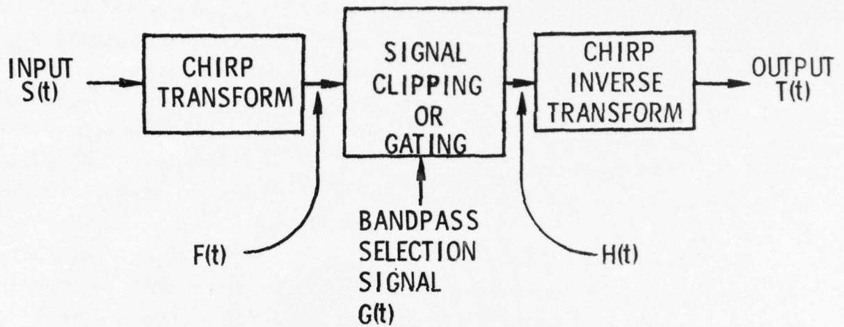
Figure 73 Configuration to Perform Prewhitening (But Not Matched Filtering)
