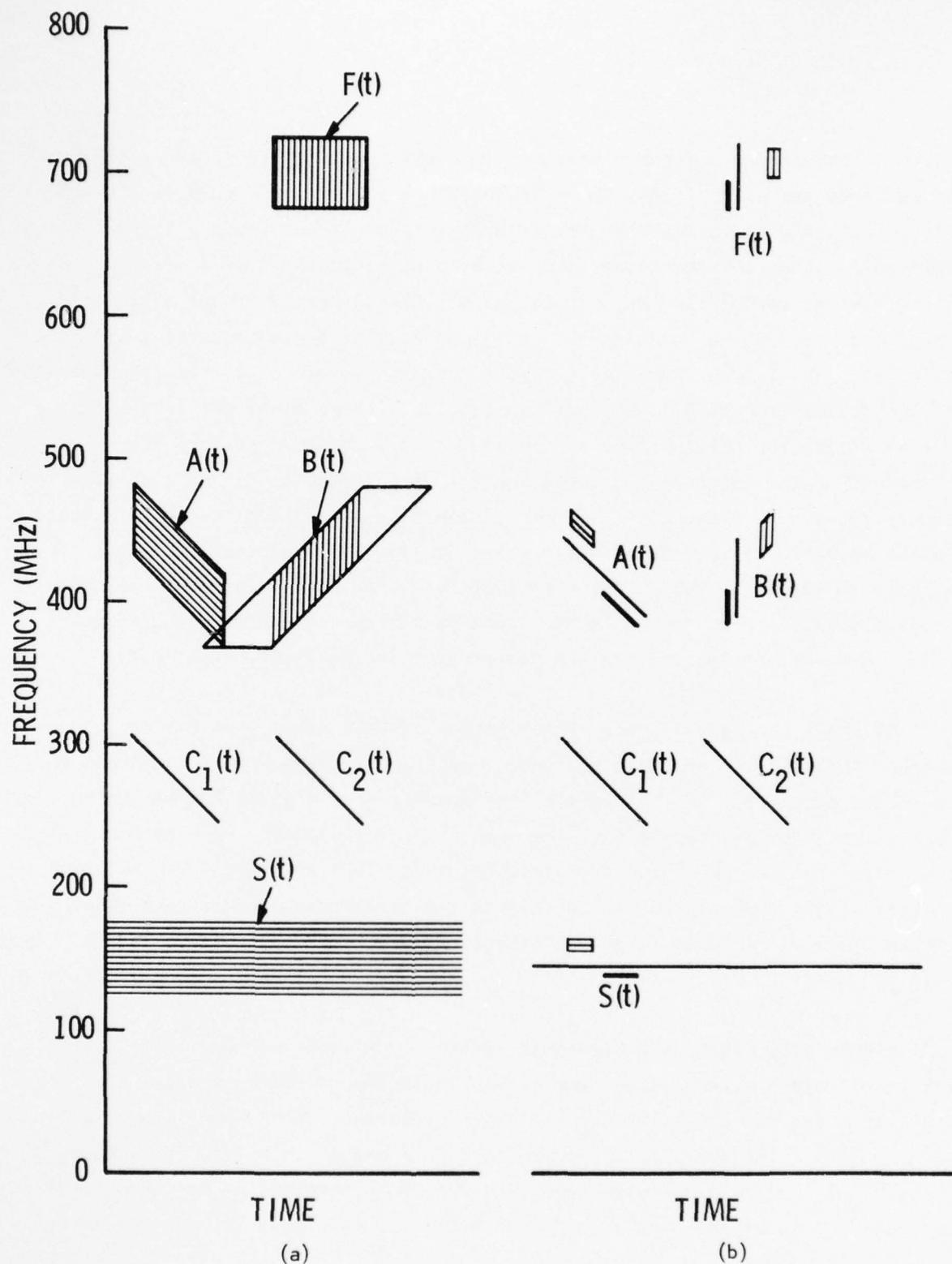
Figure 4 Frequency-Time Diagram of Chirp-Z Transform Unit.
