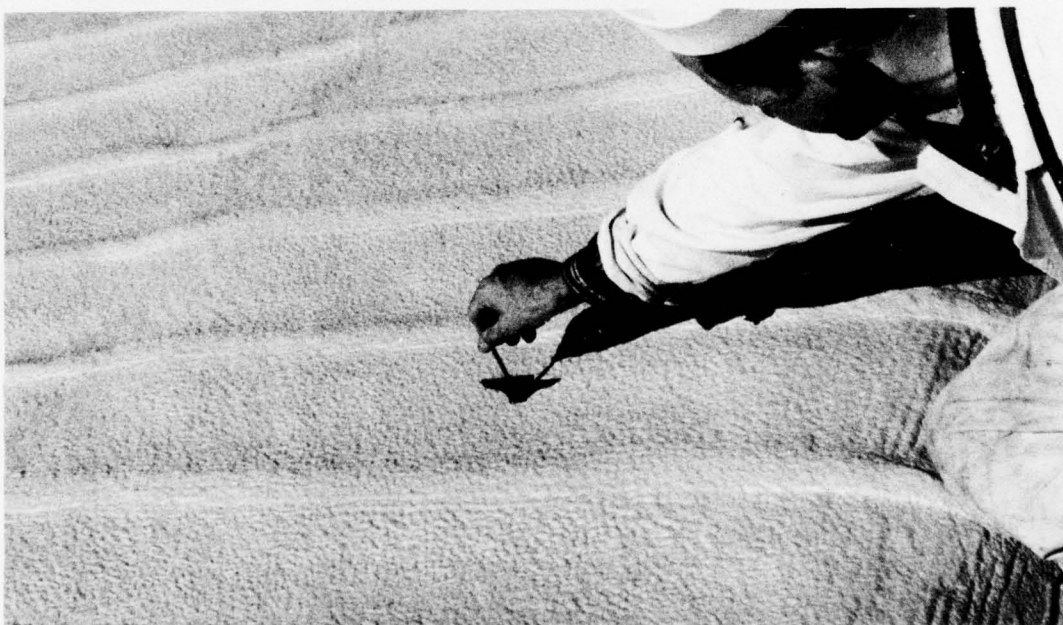
Figure 10. Measurement of Foam Thickness
