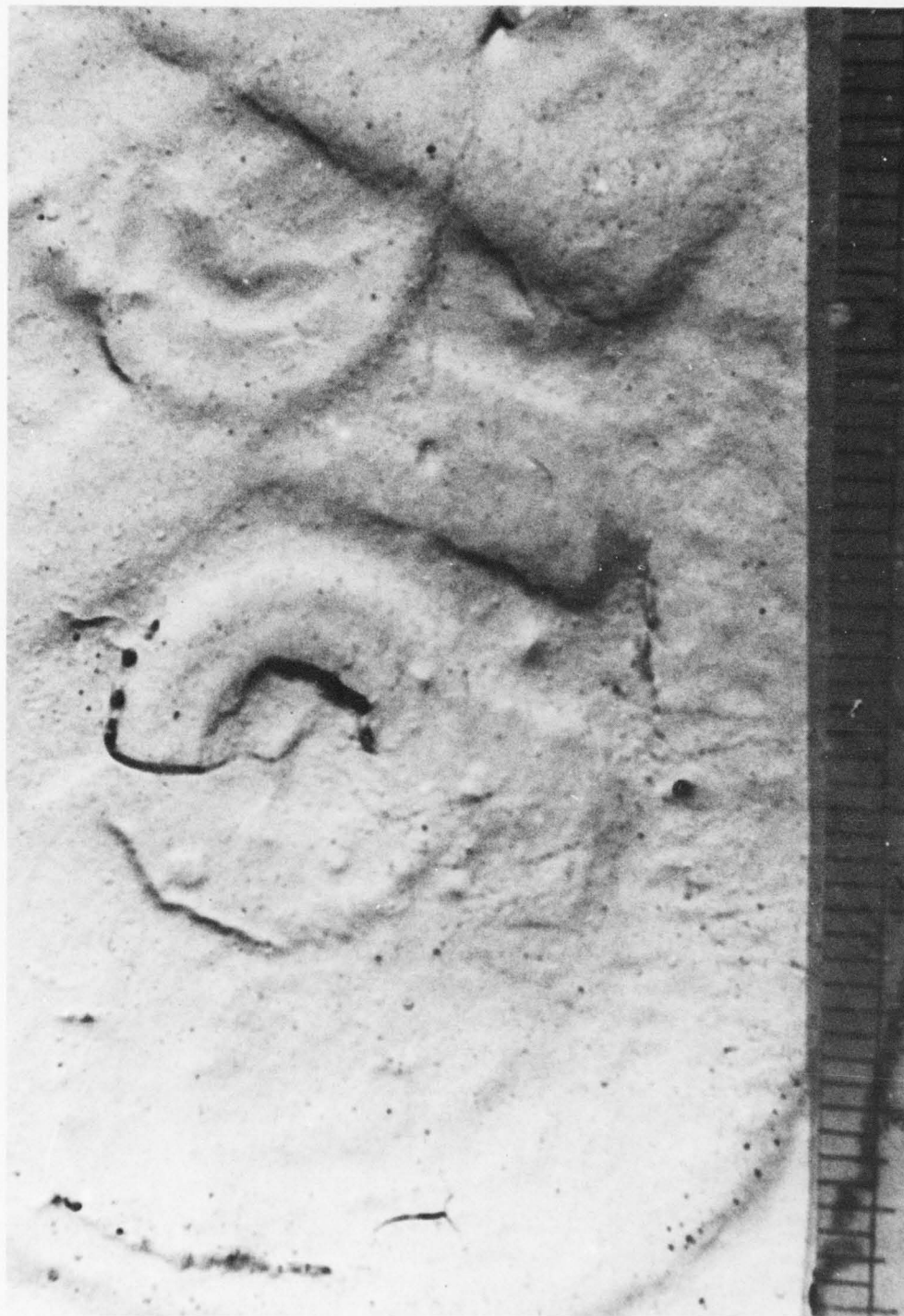
Figure 38. Cracking of Hypalon Mastic (System 4) in Heelprint After 22 Months of Weathering
