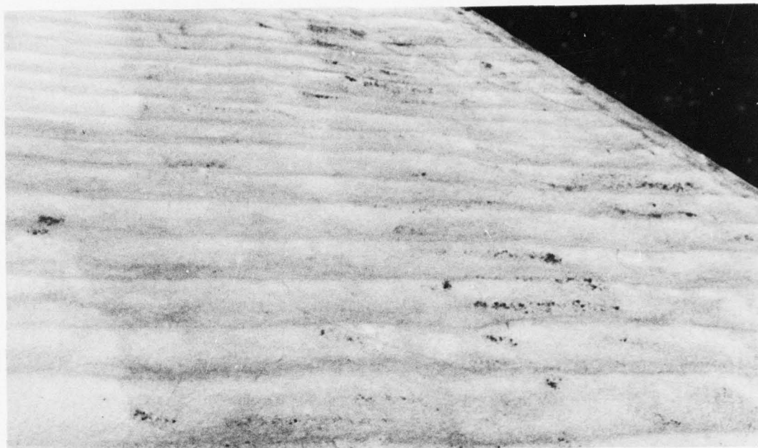
Figure 36. Area of Hypalon Mastic (System 4) Showing Greatest Erosion Damage After 22 Months of Weathering
