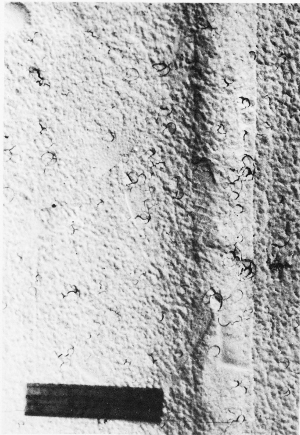
Figure 40. Hailstone Damage to Catalyzed Butyl-Hypalon (System 5) After 22 Months of Weathering
