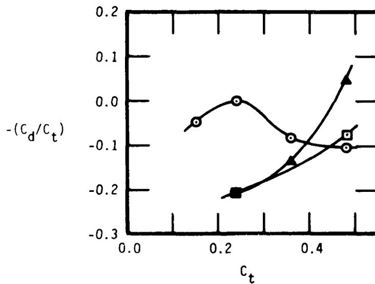
FIGURE 23 - EFFECTS OF FLAP DEFLECTION ON THRUST RECOVERY (WITH HIGH THRUST)
