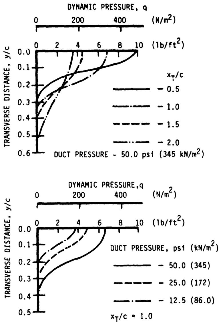
FIGURE 3 - THRUSTOR DYNAMIC PRESSURE PROFILES
