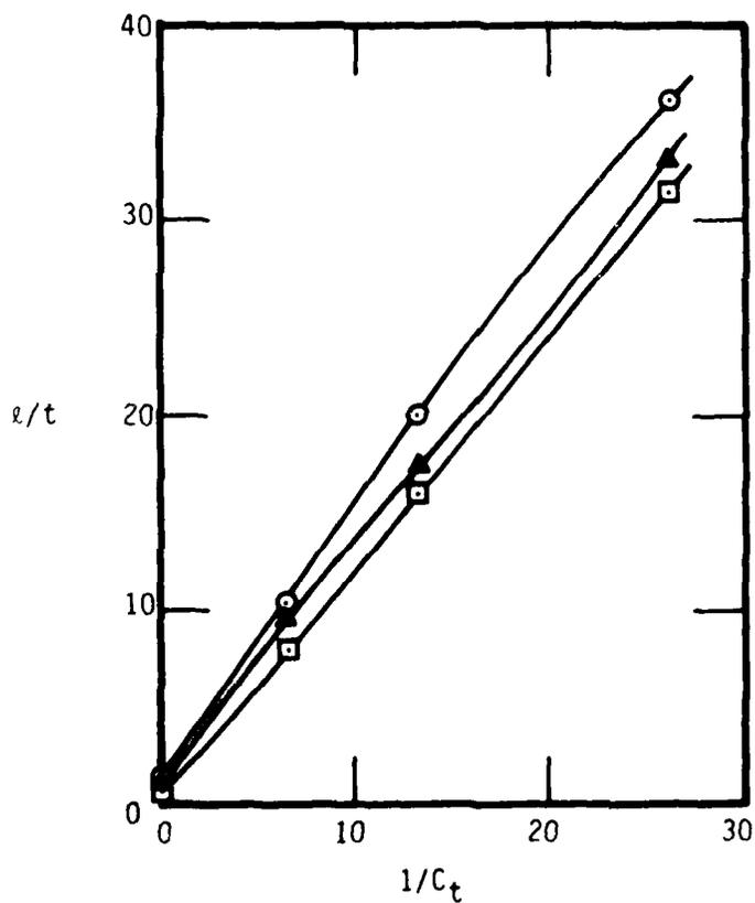
FIGURE 18 - EFFECTS OF WING SPACING ON AUGMENTATION RATIO (WITH MODERATE THRUST)
