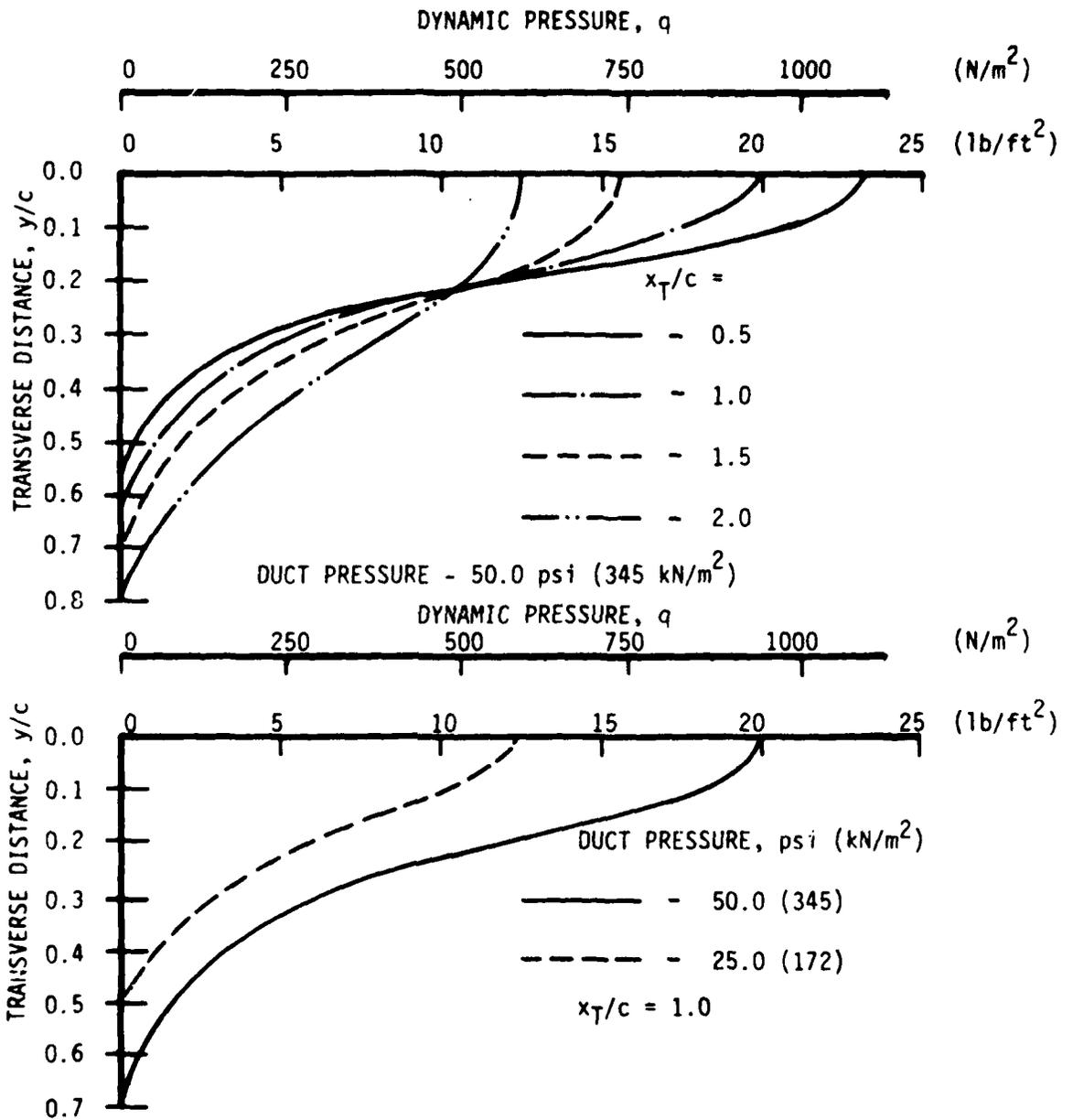
FIGURE 4 - THRUSTOR DYNAMIC PRESSURE PROFILES
