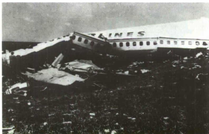
Fig. 93. Post-crash view of Douglas DC-7 aircraft crash-tested by the FAA showing typical extreme buckling of the fuselage (Photo courtesy FAA).
