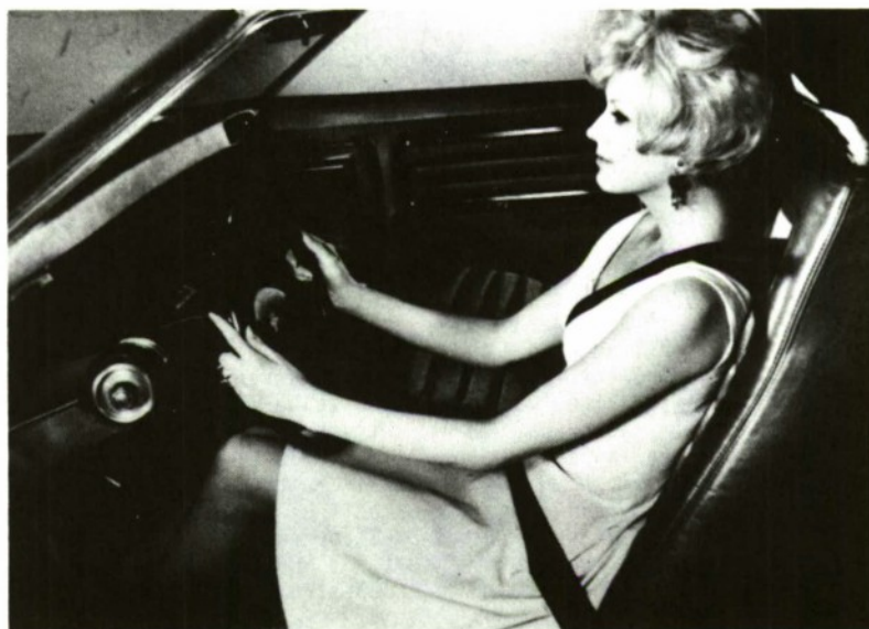
Fig. 43. An integrated harness system in which the upper torso restraint retracts into the seat back as designed for the Ford Techna future idea car (Photo courtesy Ford Motor Company).
