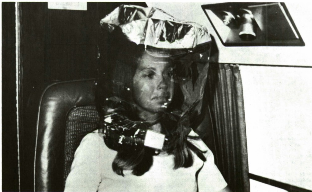
Fig. 25. Once smoke hood is donned it may protect the passenger against toxic fumes and smoke for 4 to 6 minutes, and protect the head and face against the effects of flames exceeding 800^{\circ}\text{C} ( 1,472^{\circ}\text{F} ), providing additional emergency egress capability (Photo courtesy Chrysler Corporation).
