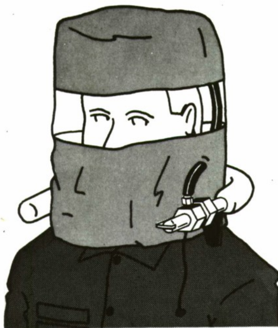
Fig. 37. Experimental FAA/Sheldahl Hood - Self-Contained Air Supply
