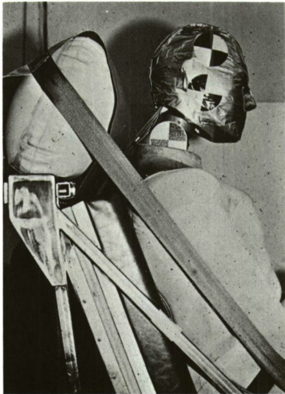
Fig. 68. Instrumented dummy and prototype deployable head restraint (Photo courtesy J. Melvin, HSRI).
