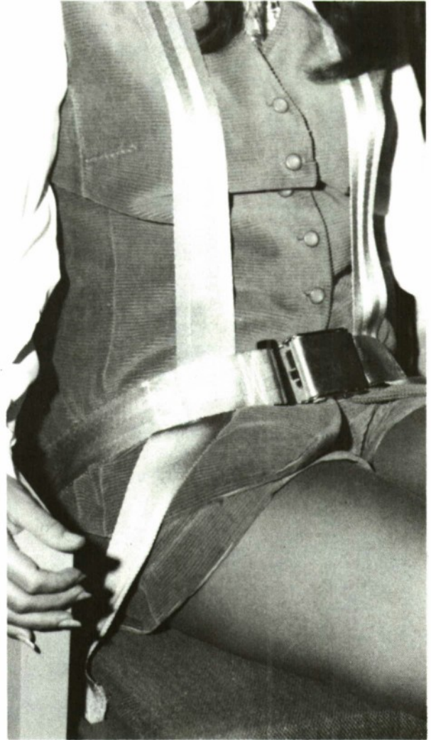
Fig. 49. Details of NASA Ames integrated restraint system in mock-up seat (Photo courtesy C. Kubokawa, NASA Ames).
