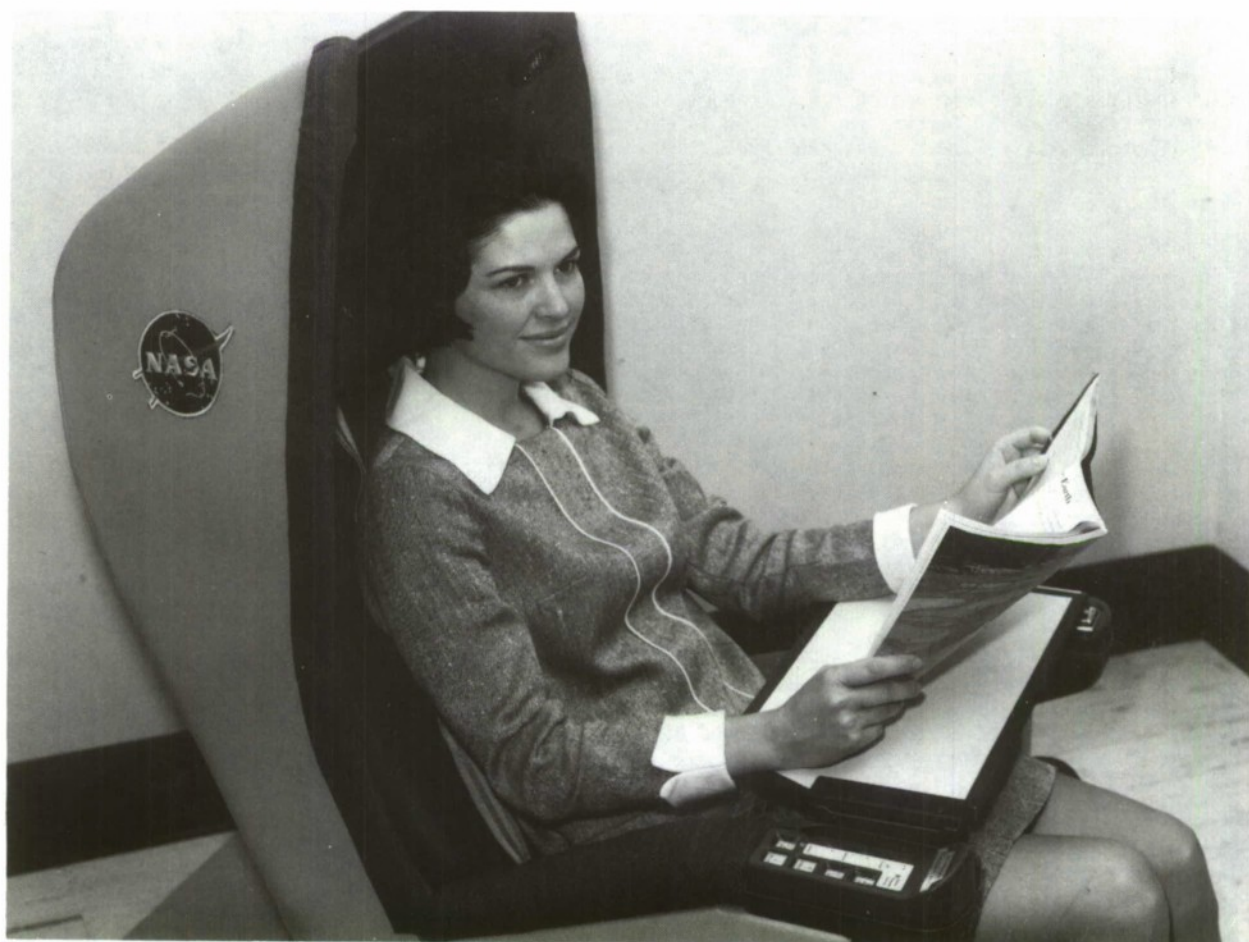
Fig. 47. Unrestrained passenger seated with food tray in place (folds back into side) in final configuration of NASA seat (Photo courtesy C. Kubokawa, NASA Ames).
