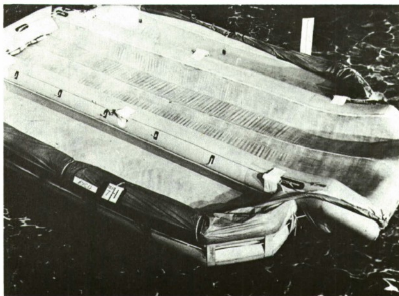
Fig. 85. Combination life raft escape slide recently certified for civil air carrier use on the McDonnell Douglas DC-10 (Photo courtesy E.B. McFadden, FAA).
