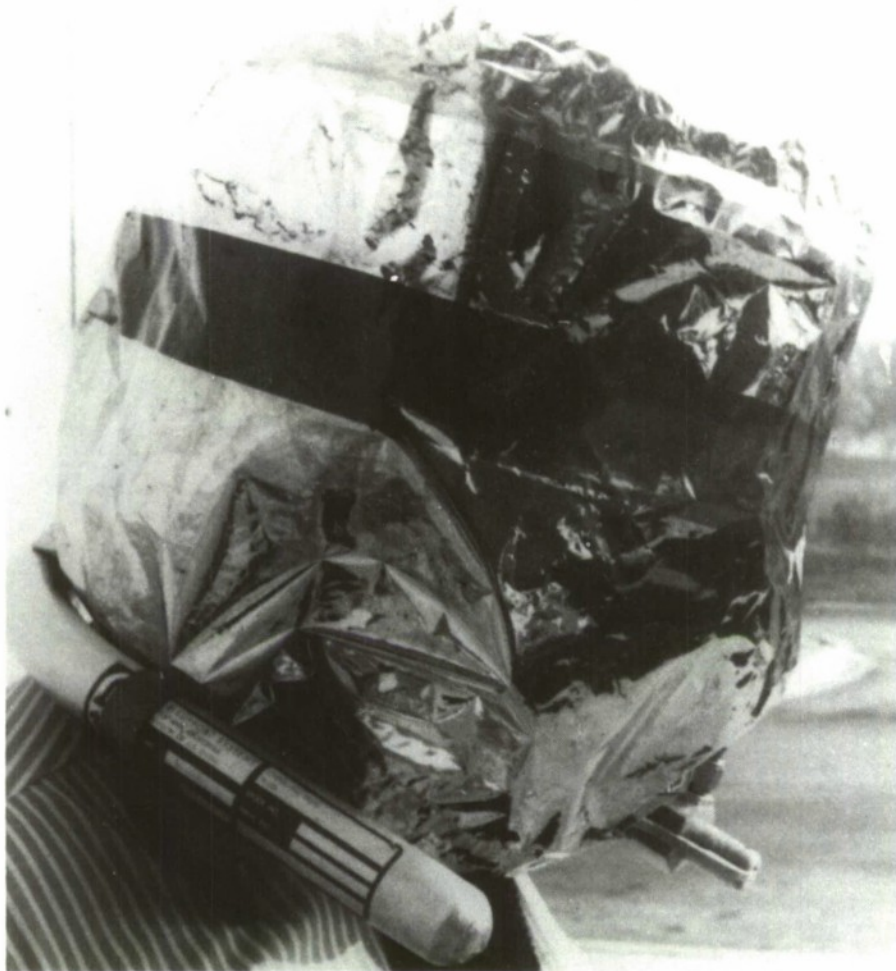
Fig. 42. Experimental FAA/Schjeldahl protective hood of 2 mil Kapton which can provide 4 to 8 minutes of breathing time using a self-contained supply of compressed air.
