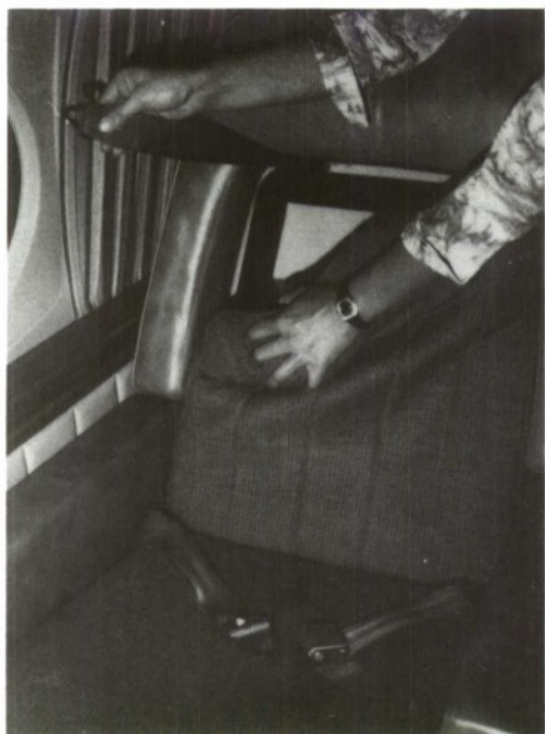
Fig. 50. Integrated seat utilized operationally in Chrysler Corporation's Grumman Gulfstream G-2 jet corporate aircraft.
