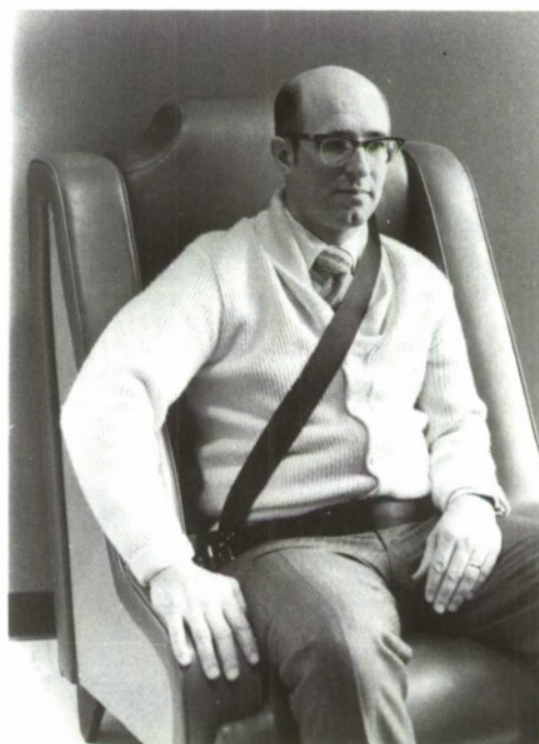
Fig. 53. Integrated restraint system designed and developed by HSRI, The University of Michigan on NHTSA advanced concepts contract (Robbins et al., 1971).
