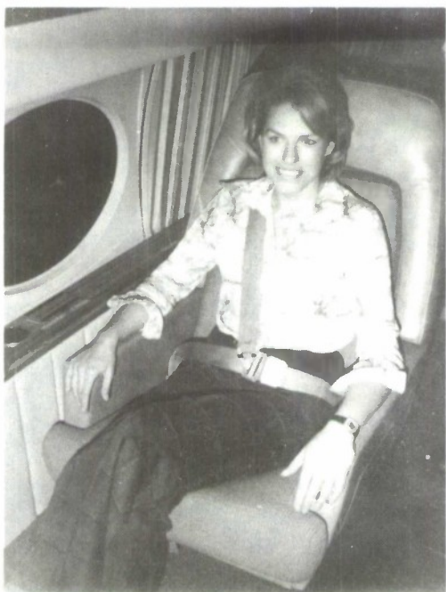
Fig. 52. In this configuration the belt buckles at the center. This seat is also capable of rotating 180° and can be used in a rearward-facing orientation.
