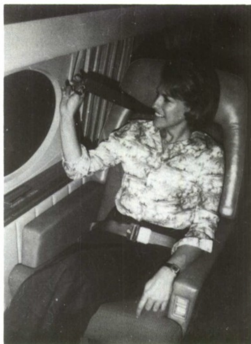
Fig. 51. The upper torso belt is attached to an inertial reel, allowing freedom of motion, but restraint in +2G deceleration.
