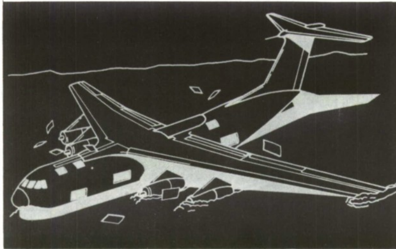
Fig. 99. ELSIE system for instantaneous egress as might be conceived for Lockheed C-141 aircraft.
