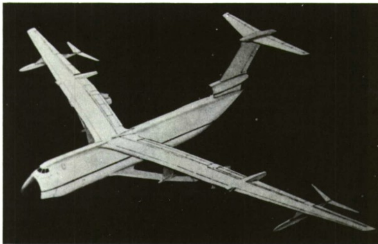
Fig. 6. Boeing concept of high wing air transport braced by struts. After Aviation Week , 1975 (29).
