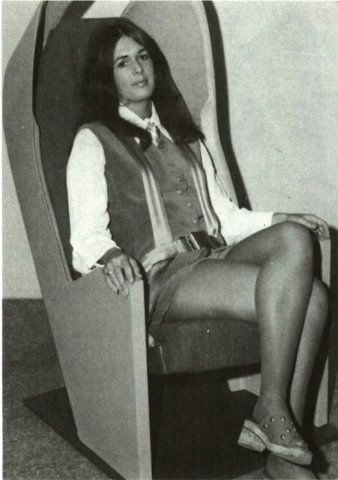
Fig. 48. The restraint system shown in this mock-up seat features upper torso protection. Freedom of movement is allowed by inertia reels in the integrated seat (Photo courtesy C. Kubokawa, NASA Ames).
