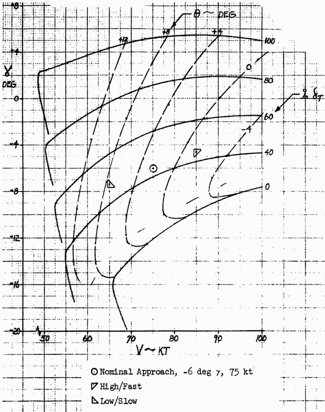
Figure E-3b. Performance Curve for BSL2
