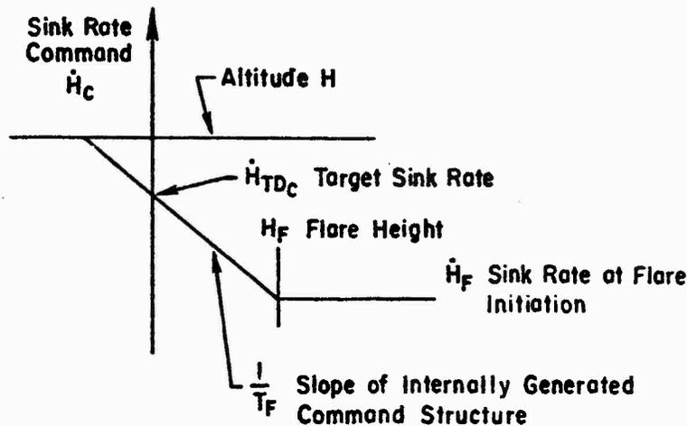
Figure 21. Assumed Command Structure for Closed Loop Flare
