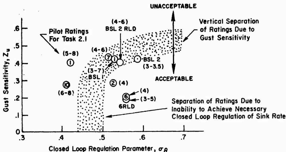
Figure 31. One Possible Way of Using Key Parameters to Correlate Minimum Acceptable Path Control with Aircraft Configuration
