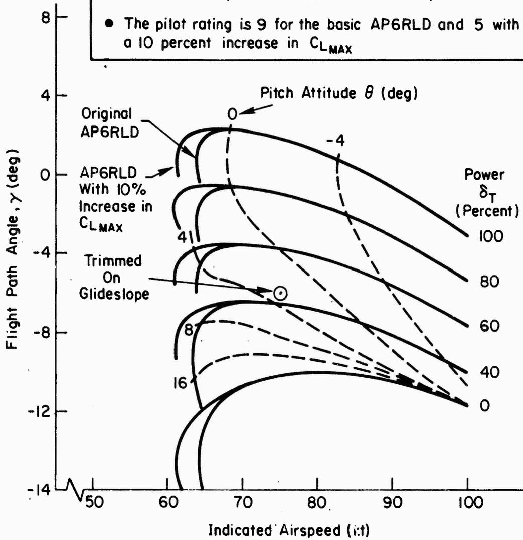
Figure 12. Effect of 10 Percent Increase in  $C_{Lmax}$  on Stall Characteristics
