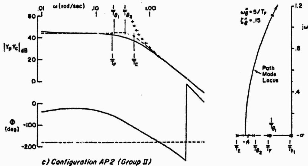
Figure 24. Generic Characteristics of Loop Closure for Attitude Flare
