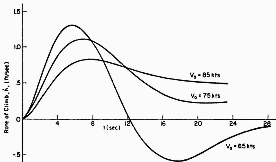
Figure 8. Effect of Speed on Path Response to a Unit Step Power Input (AP10)
