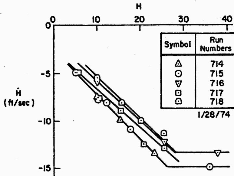
Figure 20. Phase Trajectories for Five Consecutive Flares — No Turbulence — Configuration BSL2, Pilot 7
