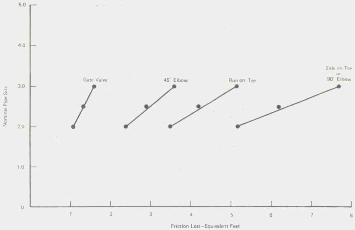
FIGURE 1. FRICTION LOSS FOR SELECTED PIPE FITTINGS—
