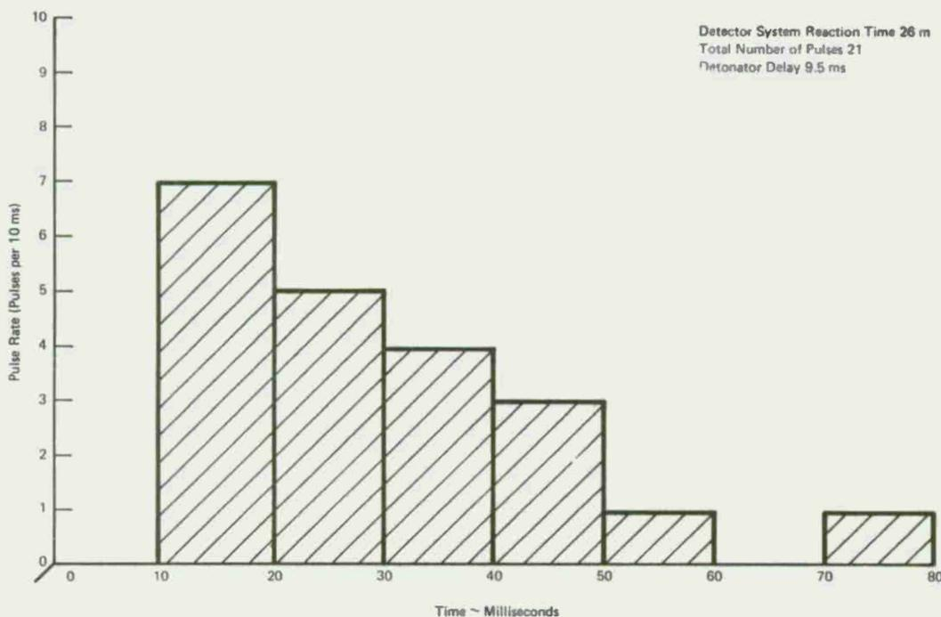
FIGURE 7. DETECTOR RESPONSE FOR 454 (1-LB) C-4 CHARGE
