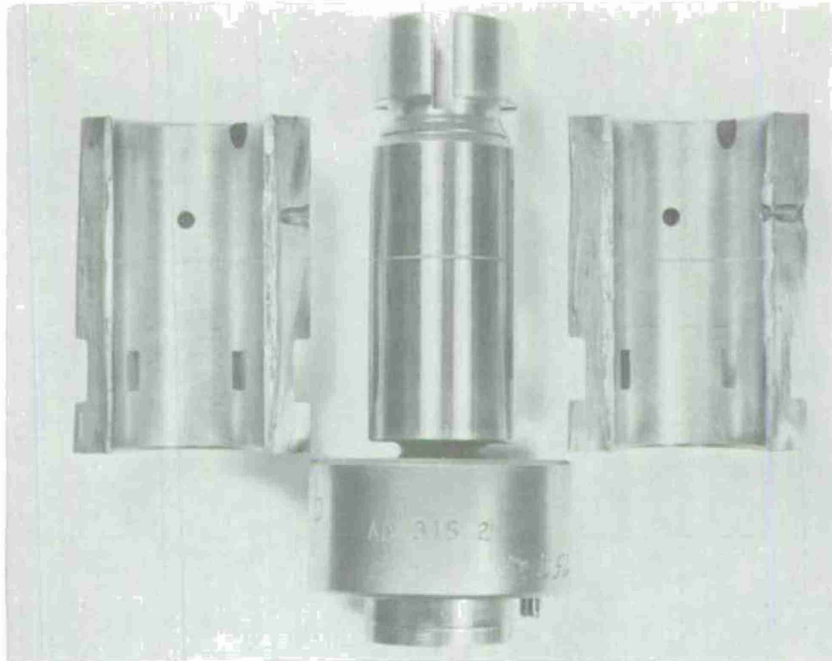
FIGURE 10c. SEIZURE NO. 3 TCCS PUMP OPERATED ON DF-2/WHITE MINERAL OIL BLEND WITH VISCOSITY OF 72 cS AT 38°C
