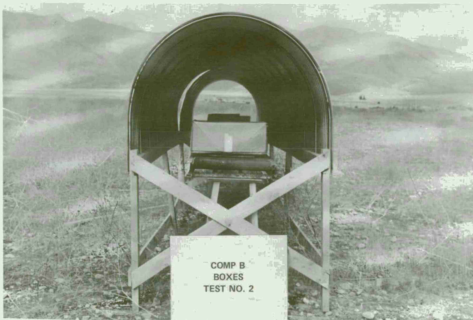
Fig 3 Test setup, 60 lb comp B boxes
