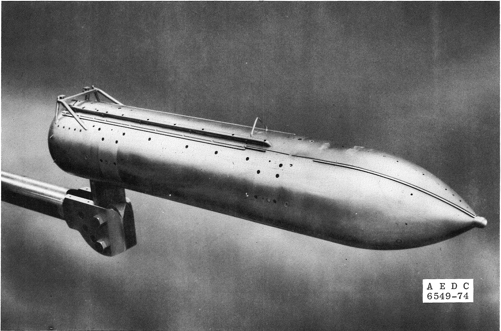
Figure 2. Photograph of the NASA external tank 0.015-scale model.
