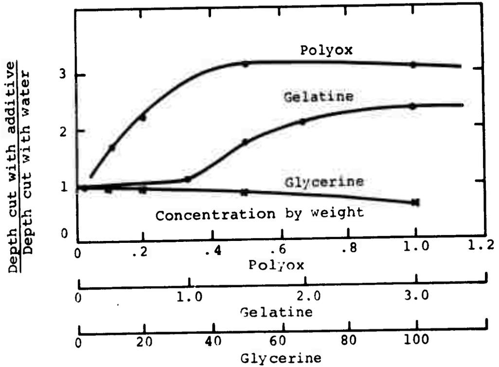
Figure 97. Variation in relative penetration in wood with additive concentration for three additives (after Ref. 39).
