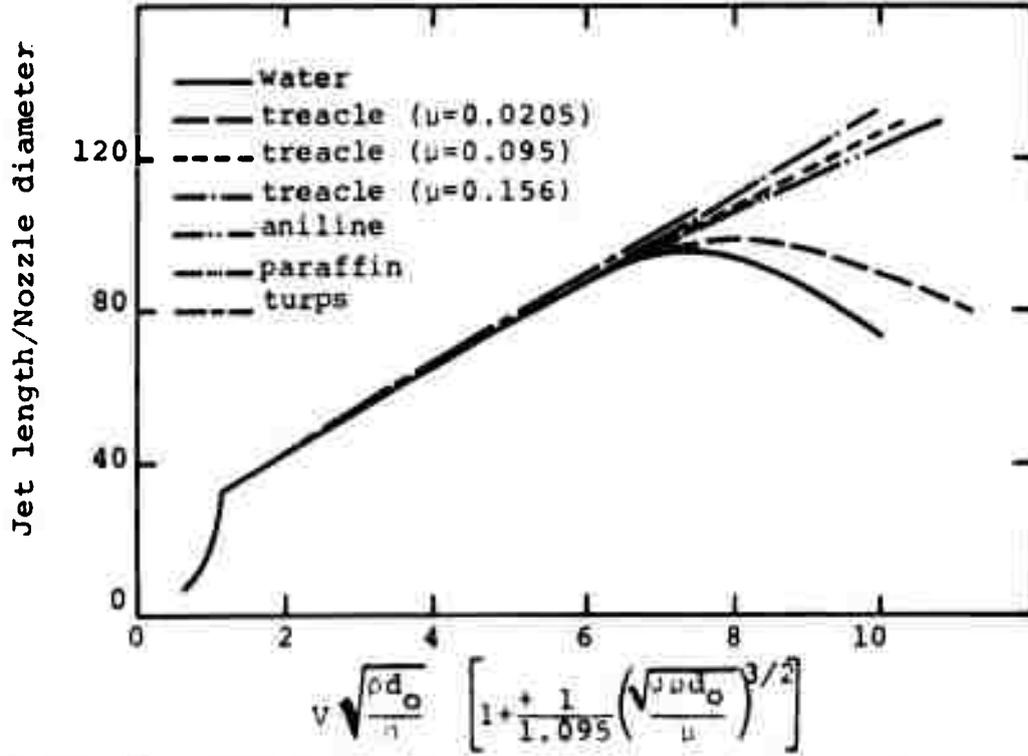
Figure 87. Variation in jet length with fluid properties for various fluids (after Ref. 54).
