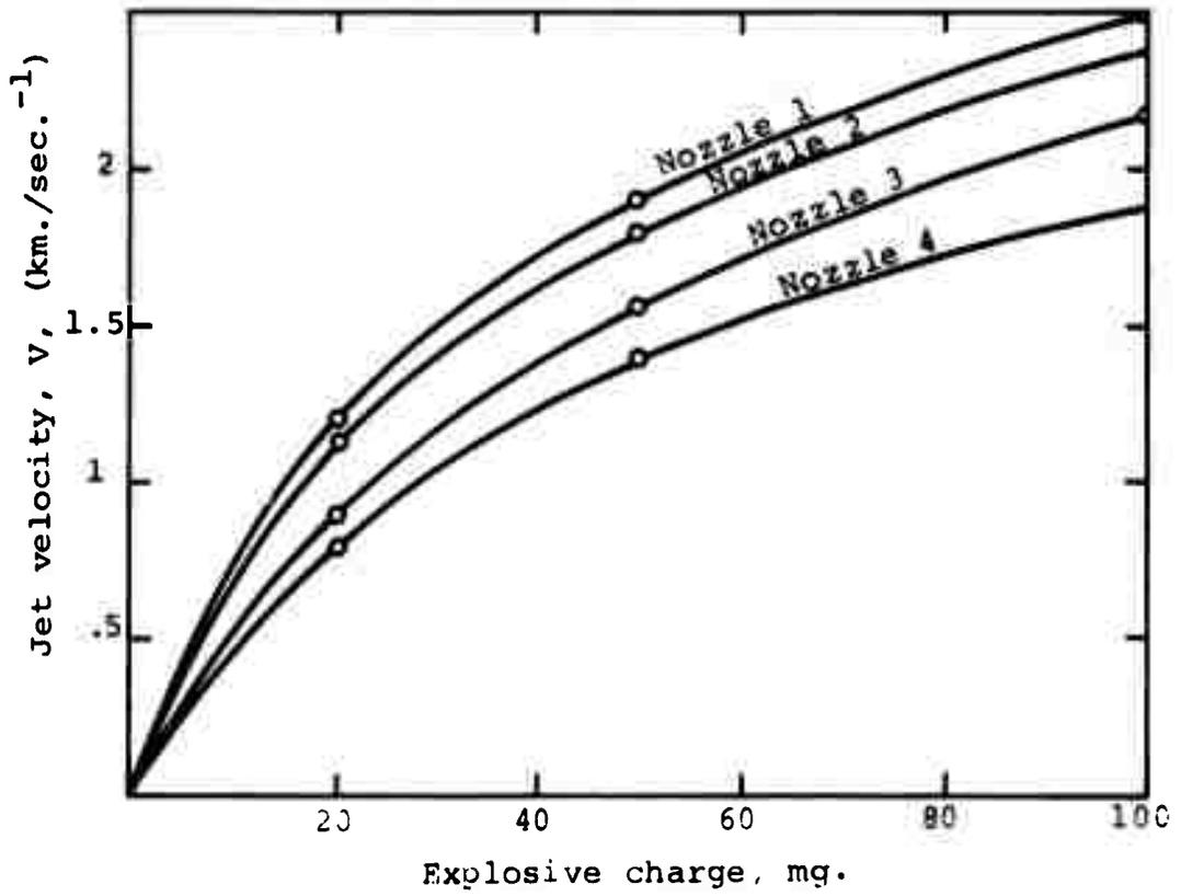
Figure 68. Jet velocity as a function of explosive charge for four different nozzles (after Ref. 46).
