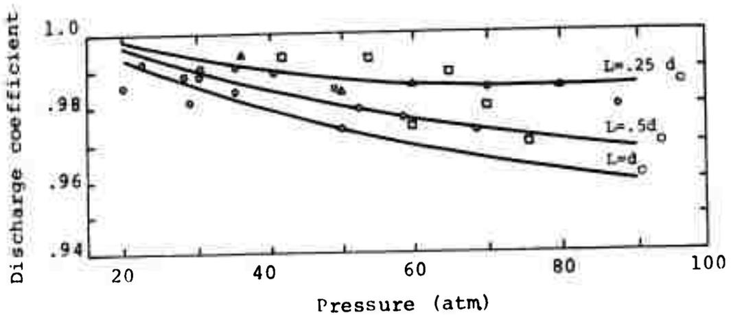
Figure 45. Discharge coefficient as a function of pressure and throat length (after Ref. 32).
