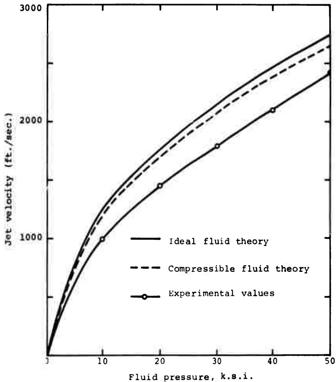
Figure 34. Variation in jet velocity with change in pump pressure (after Ref. 19).
