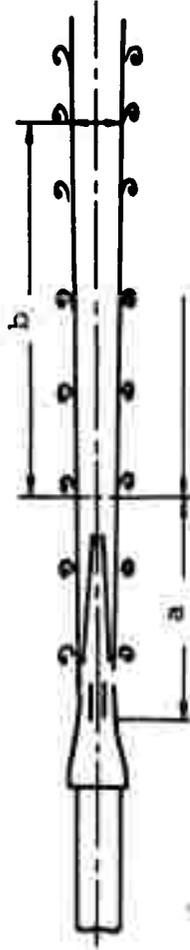
Figure 37. Liquid jet structure at medium and high pressure. Length "a" is the basic length and "b" is the effective length (after Ref. 32).
