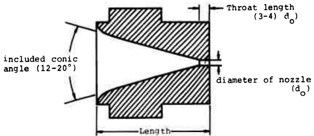
Figure 54. Typical nozzle geometry.
