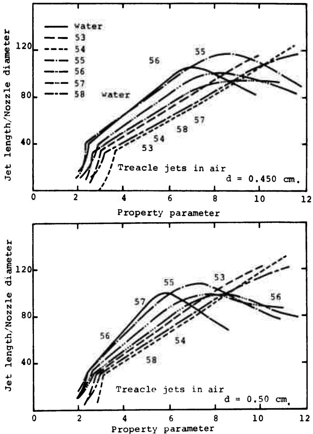
Figure 85. Variation in jet length with fluid properties for various treacle solutions at two nozzle diameters (after Ref. 53).
