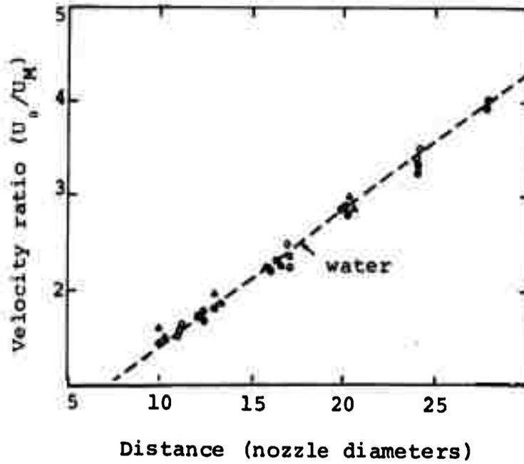
Figure 104. Centerline velocities for 75 p.p.m. Guar Gum, ● ; 150 p.p.m. Guar Gum, ○ ; and 200 p.p.m. HEC, ▲ with distance (after Ref. 66).
