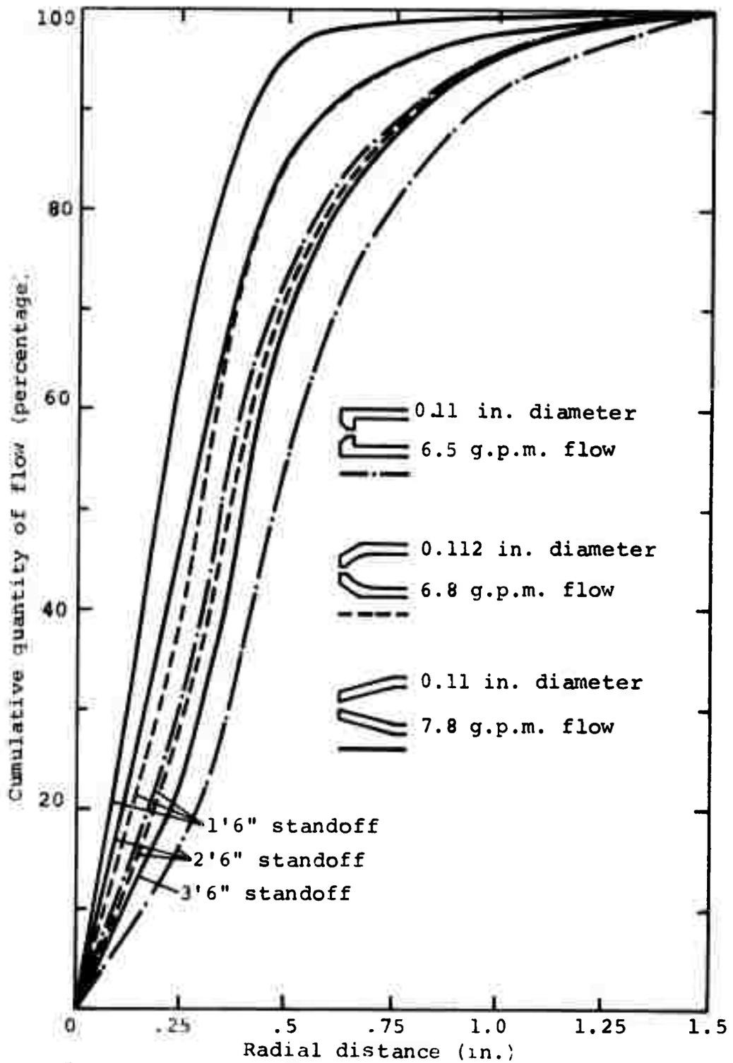
Figure 76. Jet volume distribution for various nozzle shapes at 1000 p.s.i. for three standoff distances (after Ref. 48).
