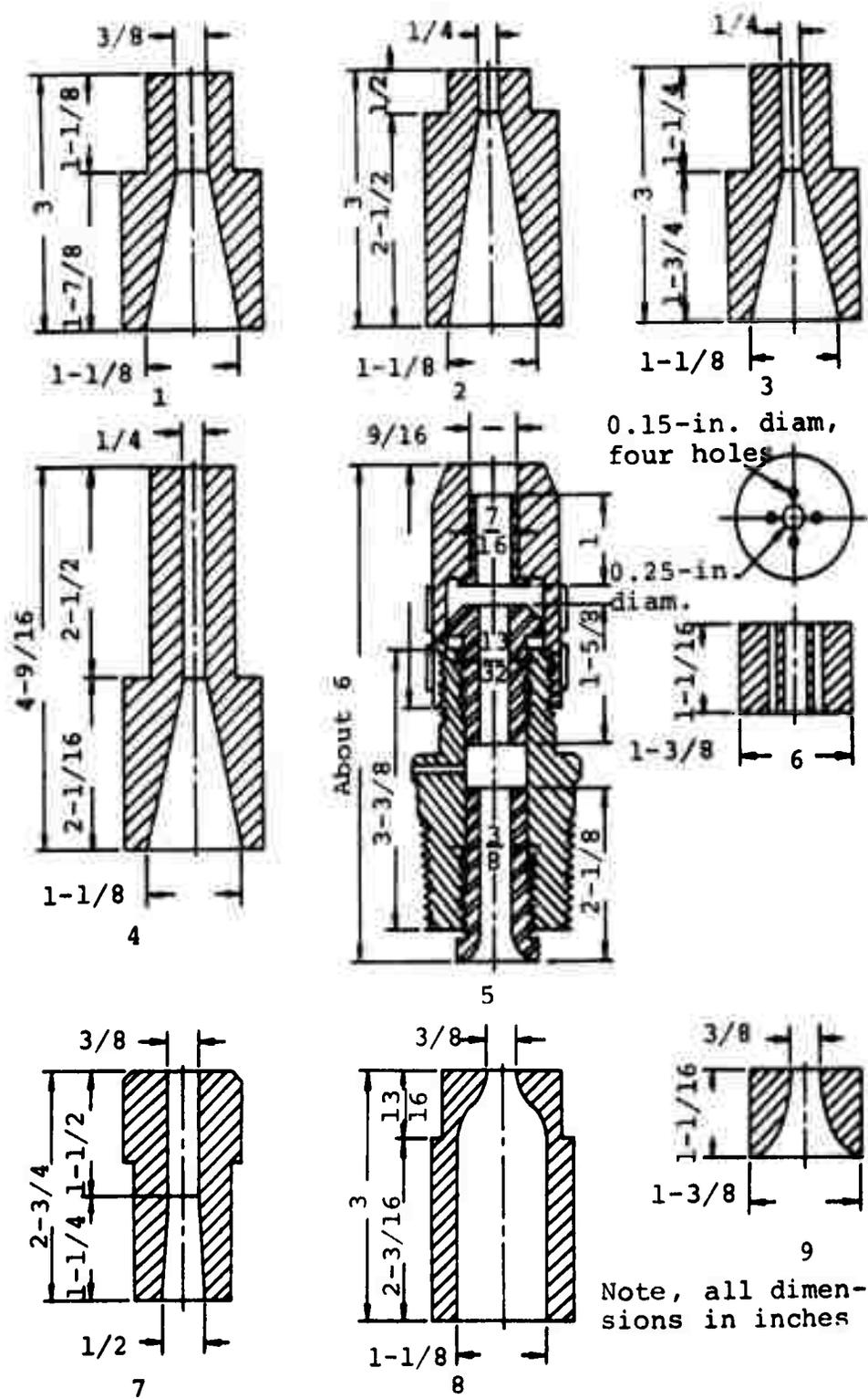
Figure 71. Various types of nozzles used by the U.S. Bureau of Mines (after Ref. 47).
