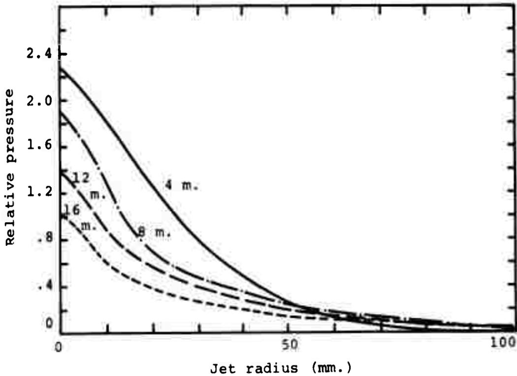
Figure 79(c). Variation in pressure distribution with distance (nozzle 3, Figure 78, after Ref. 49).
