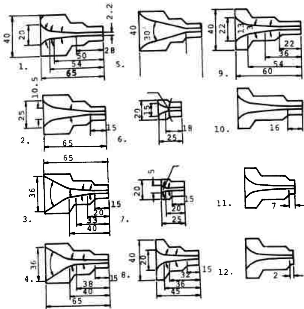
Figure 61. Profiles of experimental nozzles (after Ref. 42).
