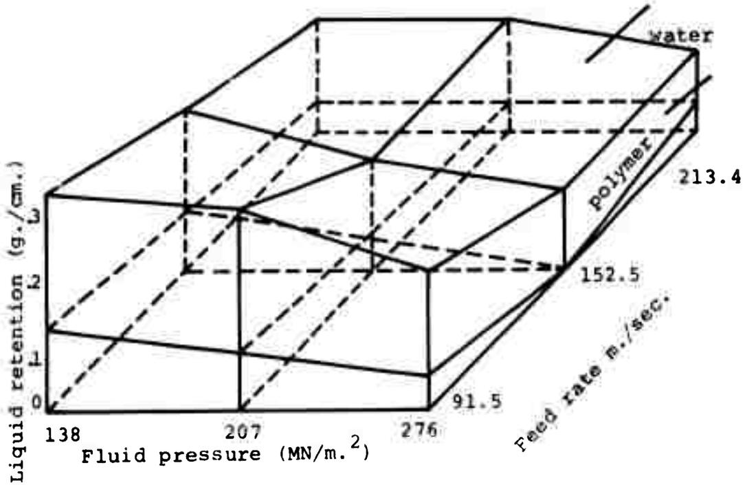
Figure 99(b). Variation in liquid retention for 0.44 kg./m.<sup>2</sup> corrugated board showing the effect of Polymer (after Ref. 39).
