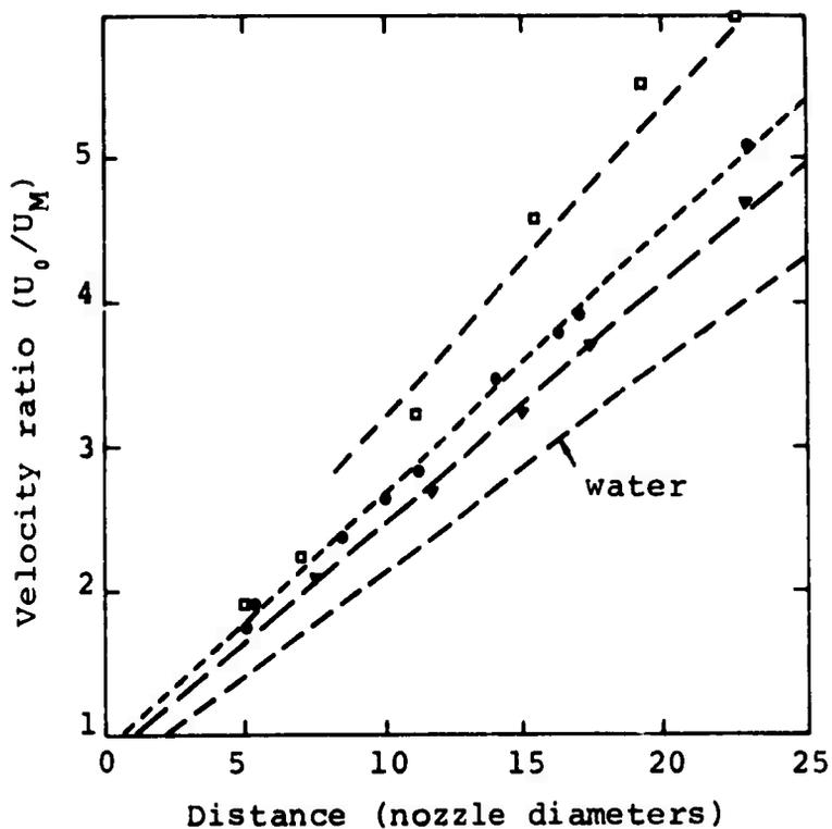
Figure 105. Centerline velocities for 50 p.p.m. of Polyox solutions, □,  $1.9 \times 10^6$  M.W., ●,  $1.2 \times 10^6$  M.W. and ▲,  $1.1 \times 10^6$  M.W. with distance (after Ref. 66).
