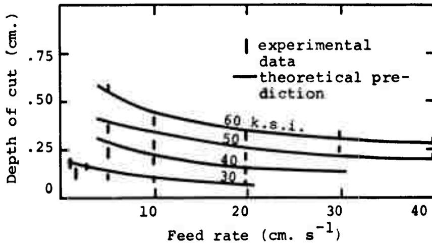
Figure 128(a). Polycarbonate cut with a nozzle of 0.076-mm. diameter (after Ref. 84).
