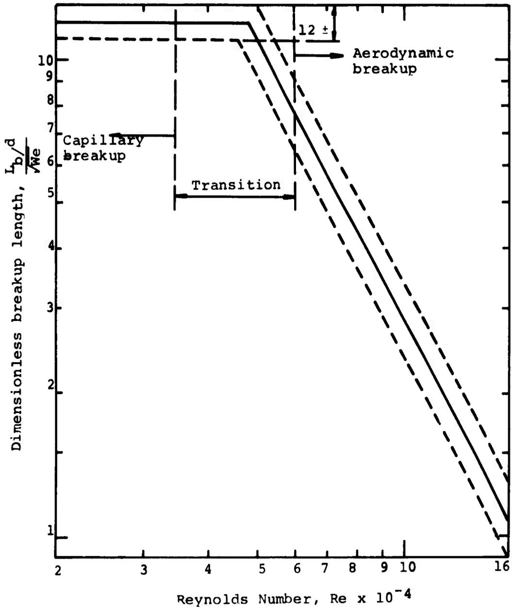
Figure 22. The effect of Reynolds Number on the form of jet breakup.
