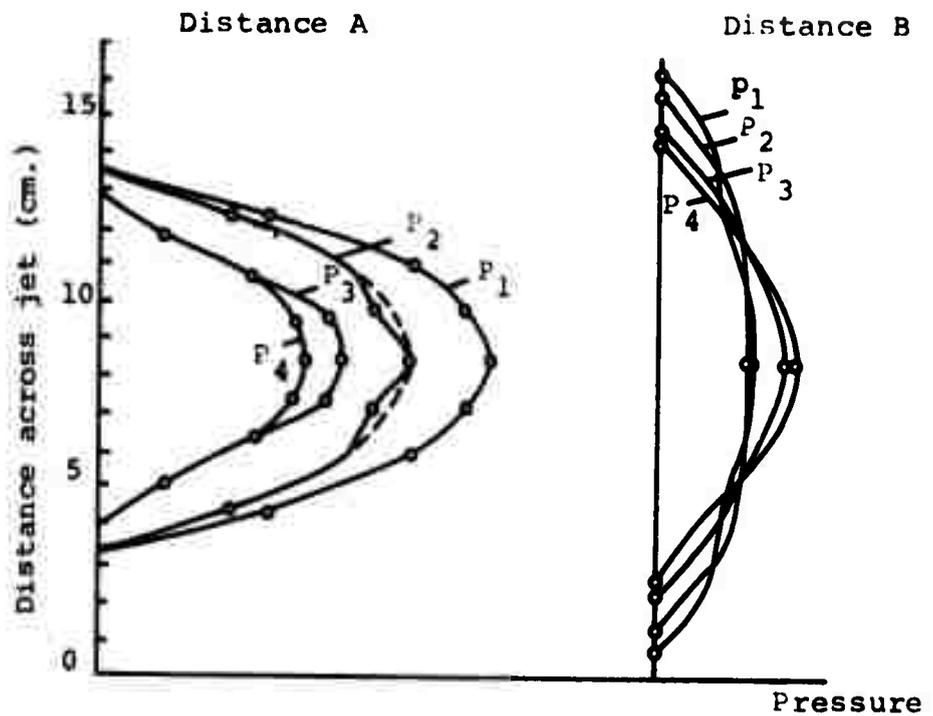
Figure 38. Relative jet pressure profiles with increasing pressure ( $P_1 > P_2 > P_3 > P_4$ ) at two standoff distances ( $B > A$ ) in front of a hydraulic monitor with a 35-mm. nozzle (after Ref. 35).
