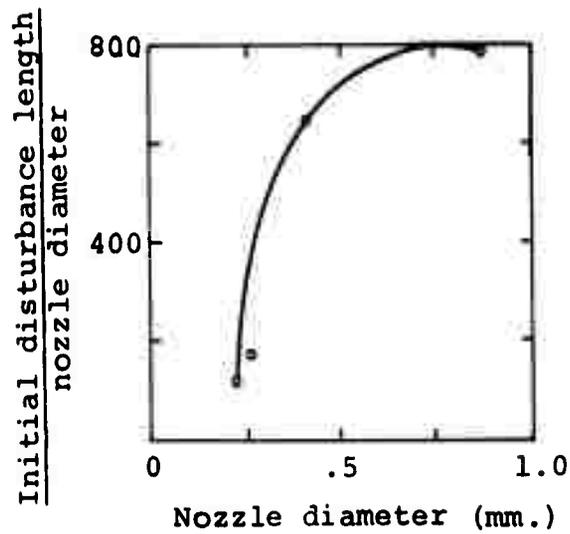
Figure 111. Variation in length with nozzle diameter for 0.25 percent Separan at 4 m./sec. (after Ref. 17).
