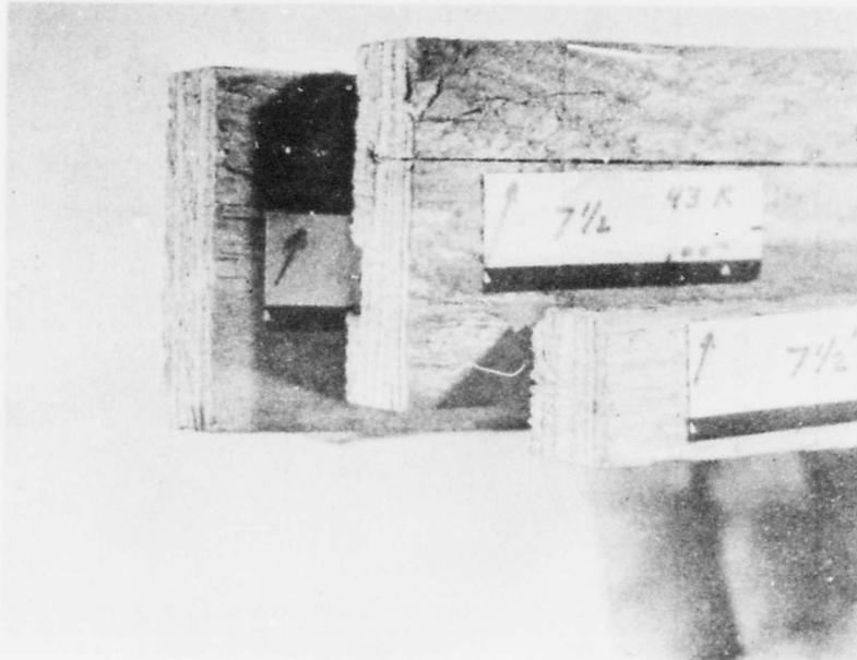
Figure 30. One-half in. plywood cut at 7-1/2 in./sec. and 43,000 p.s.i. Three nozzle diameters (0.005, 0.007, 0.012 in.).
