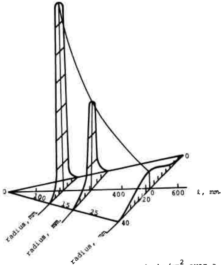
Figure 51. Distribution of momentum in  $\text{kg}/\text{cm}^2$  over a jet issuing at 1500 atm. from a 0.595 mm. nozzle (after Ref. 40).
