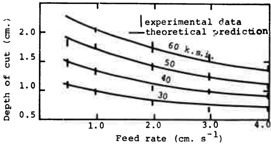
Figure 128(c). Polycarbonate cut with a nozzle of 0.178-mm. diameter (after Ref. 84).
