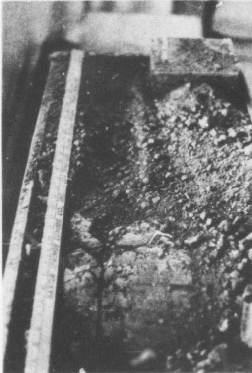
Figure 23. Loam cut by a 500 p.p.m. Polyhall, 30 k.s.i. 0.012-in. diameter jet at 10-in. standoff, showing the change where the loam changes from compacted, nearest the camera, to uncompacted.
