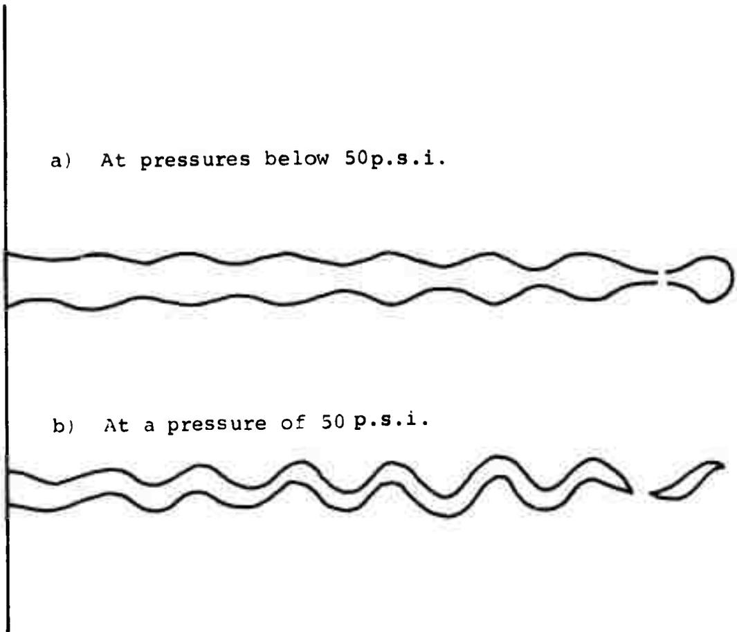
Figure 35. Forms of jet breakup at low velocities.
