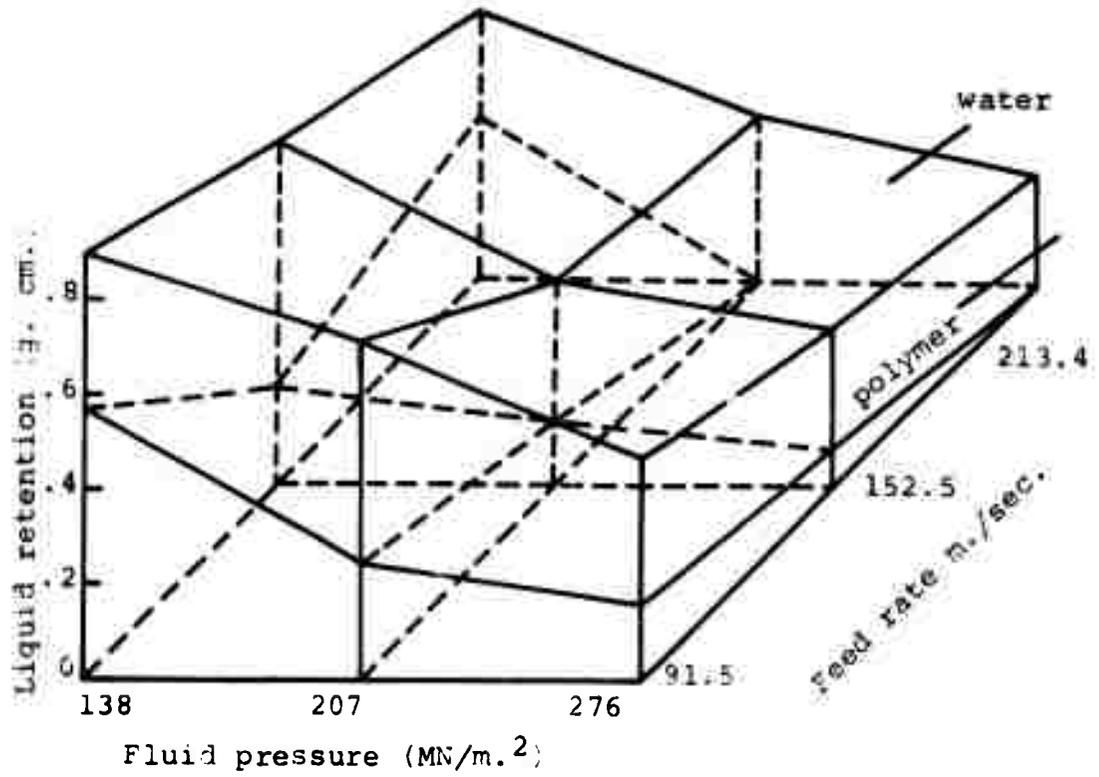
Figure 99(a). Variation in liquid retention for 0.49 Kg./m.<sup>2</sup> corrugated board.
