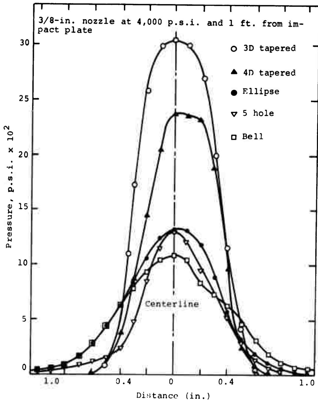
Figure 70. Pressure profile of jetstreams from various nozzle types used by U.S. Bureau of Mines (after Ref. 47).
