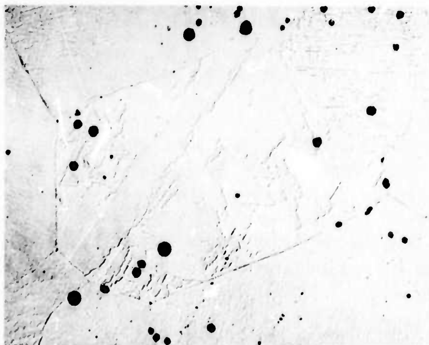
Figure 57. 80 w/o Co-20 w/o Fe Alloy Annealed at 1000°C Air Cooled to 25°C. Etched in 5% Nital. Central Grain Shows Surface Martensite (BCC) Formed during Polishing in an Austenite (FCC) Matrix (X1000).
