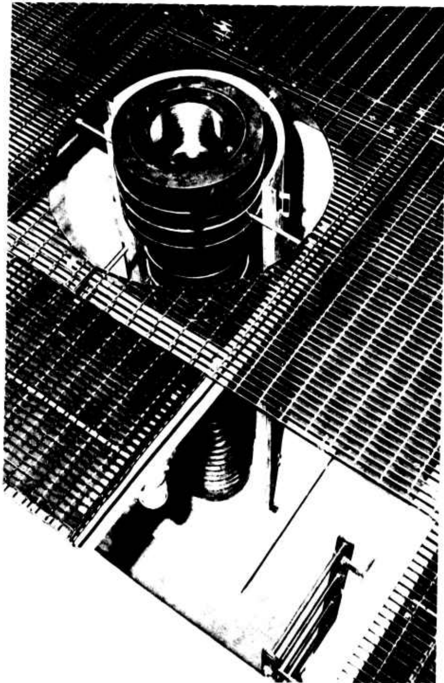
Figure 46 Nine-Inch Autoclave Installation - Insulation Jackets Removed.
