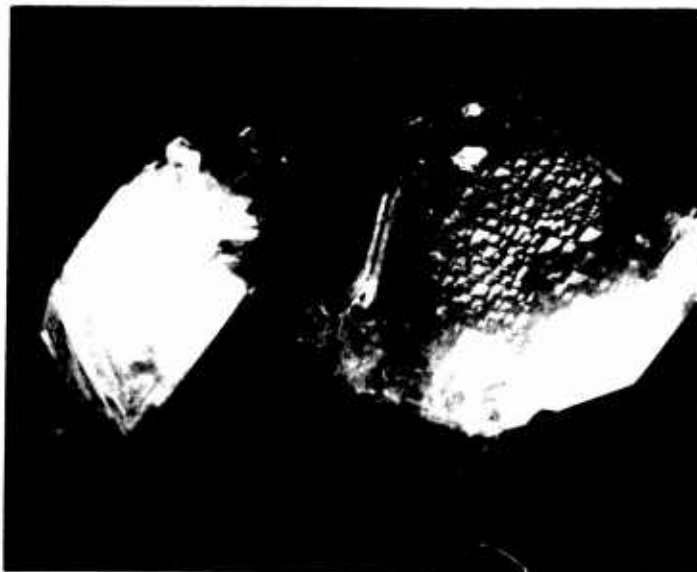
Figure 33 The effect of lithium mineralizer additions on growth on c-form faces. Inclusion of lithium in system produces smooth growth (left) on (0001) faces. Growth without lithium (right) is faceted with rhomb faces.
