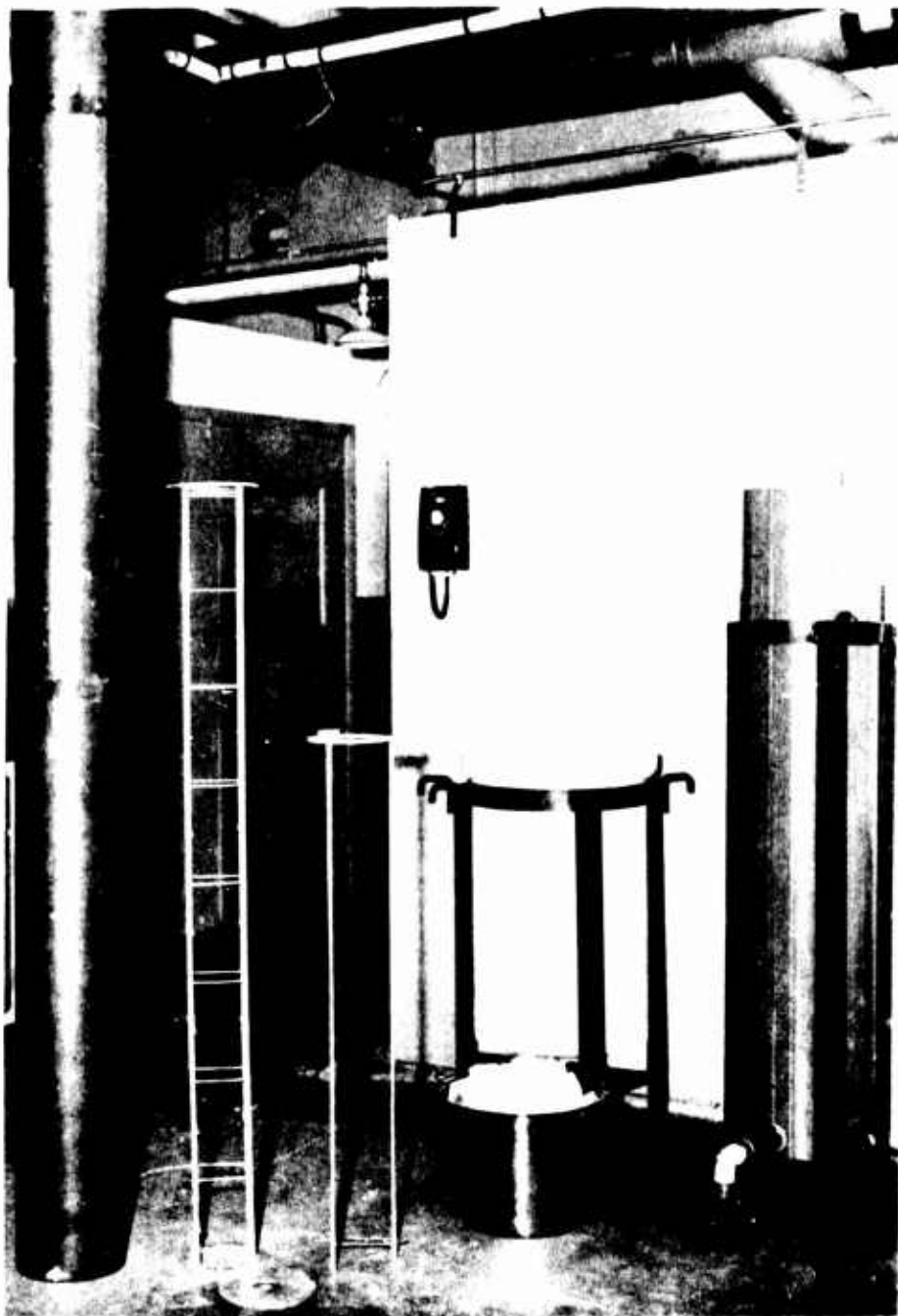
Figure 50 Production autoclave accessories. Left to right - Growth container, convection baffle, seed rack, rack support stand, and handling tanks.
