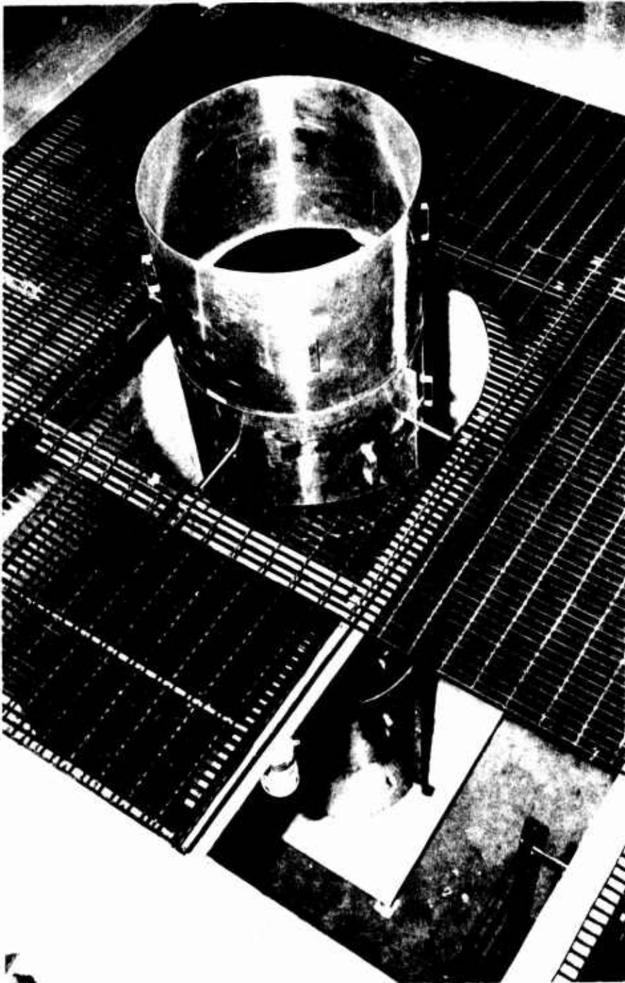
Figure 45 Nine-Inch Autoclave Installation - Leak Deflector Removed.
